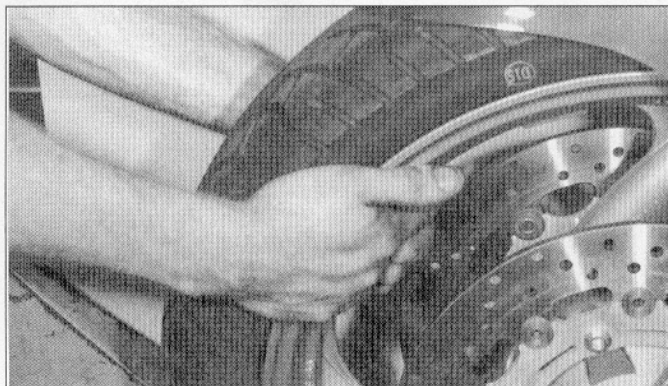
23.4 Grasp the front wheel and try to pull it back and forth; if it moves, the steering head bearings are loose and in need of adjustment
