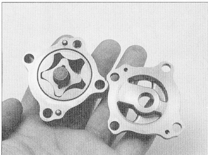
17.12 Remove the cover screw and lift off the cover
