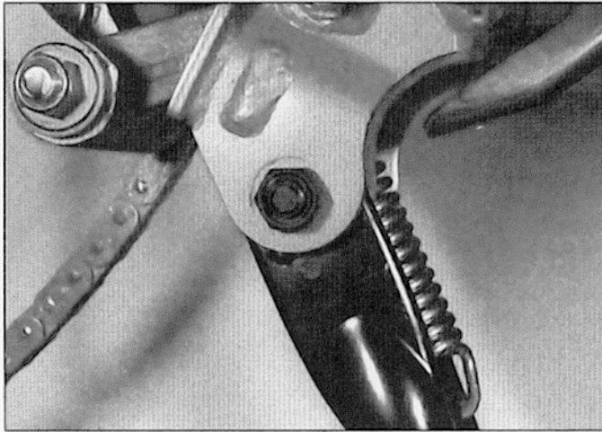
3.1 The centerstand pivots on two bolts
