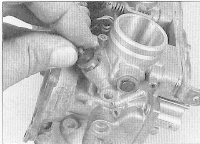
7.17a Unscrew the choke plunger cap with a box wrench (ring spanner) (FZ600 and YX600 Radian shown; XJ600 and FJ600 similar) . . .
