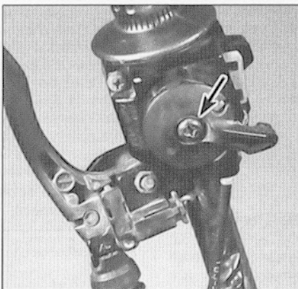
11.2 The screw that retains the choke lever on YX600 Radian models has been secured with thread locking agent; be sure the screwdriver fits correctly
