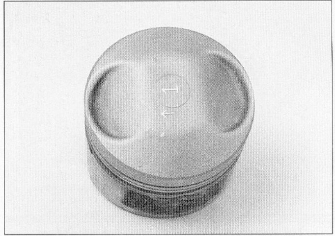
14.3a Mark the cylinder numbers on the piston crowns (if the top surface needs cleaning, use a sharp scribe so you don't accidentally remove the number) - also note the arrow, which must point to the front
