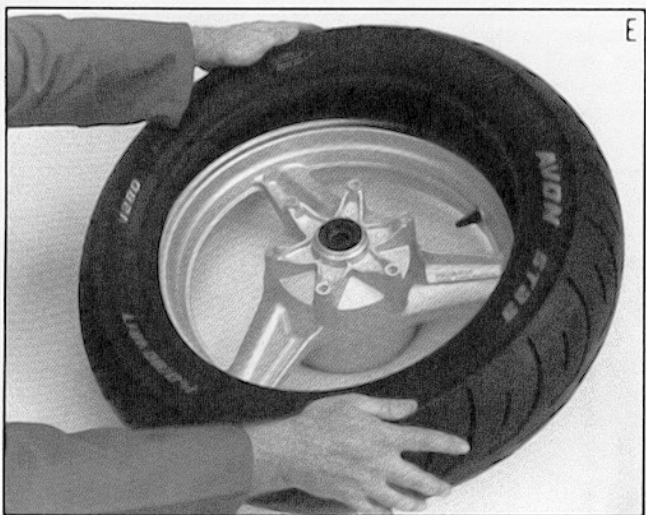
Work first bead over the rim flange.
