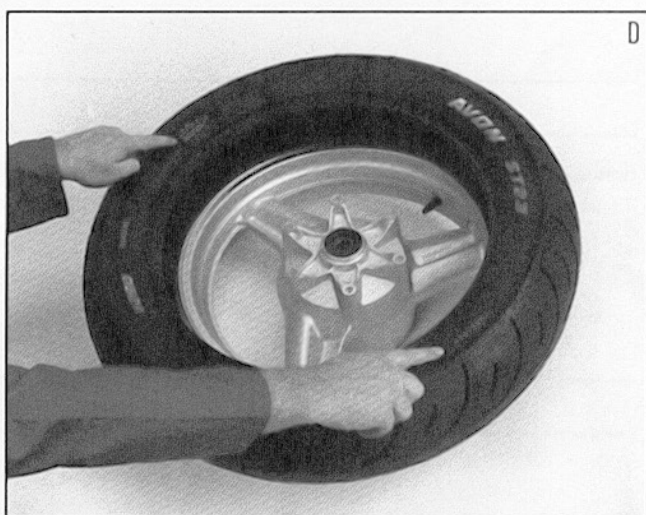
Before installing, ensure that tire is suitable for wheel. Take note of any sidewall markings such as direction of rotation arrows.
