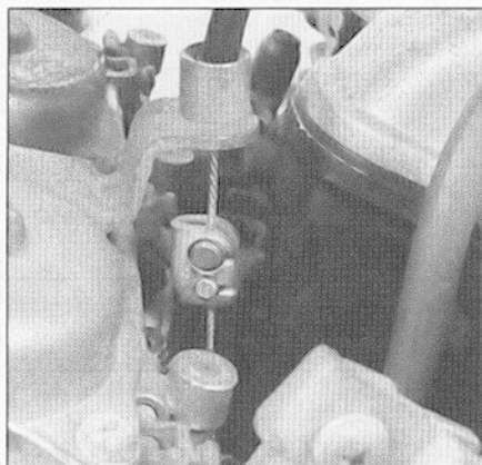
10.5 Pull up the throttle pulley to create slack in the cable, then align the cable with the slot in the pulley and slip it out
