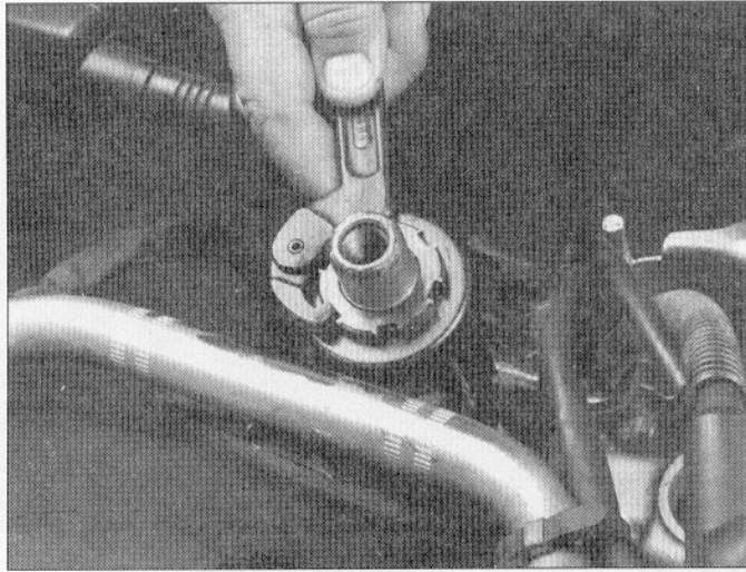
23.7 The ring nut can be tightened with a spanner wrench (C-spanner) like this one, but ideally, the spanner wrench should have a hole in the handle so a torque wrench can be used with it
