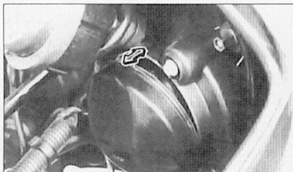
7.4 On FZ600 models, pull the cover from the back of the headlight assembly
