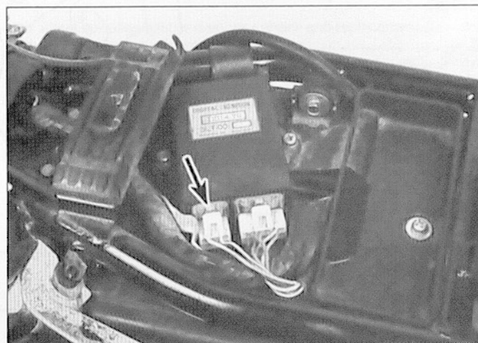
4.2 Disconnect the four-terminal connector from the igniter (YX600 Radian shown)
