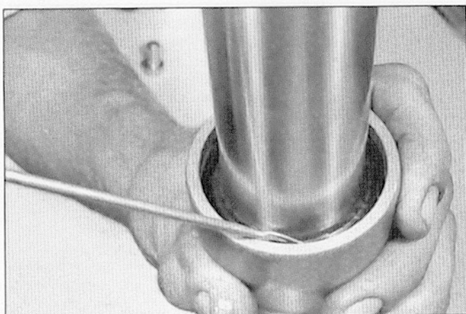
6.7 Pry out the retaining ring
