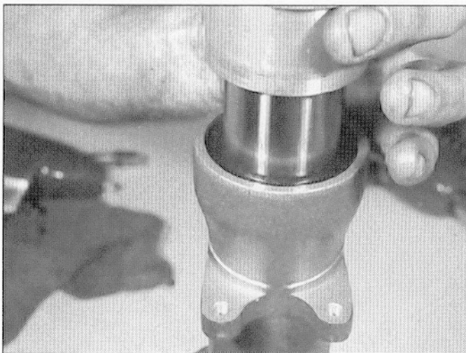
6.17a Drive the bushing into position with a tool like this one if it's available (use the tool like a slide hammer) . . .
