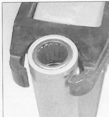
12.4 . . . to expose the bearings
