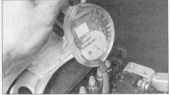
4.7 Check the specific gravity with a hydrometer
