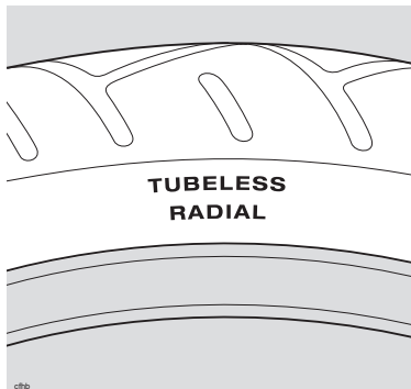
Typical Tyre Marking - Tubeless Tyre
