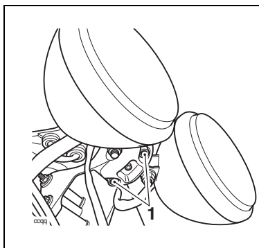
1 Vertical beam adjuster cover fasteners
