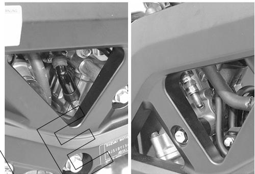
Measure ignition coil primary peak voltage (for #1 cylinder) in the following procedure.
