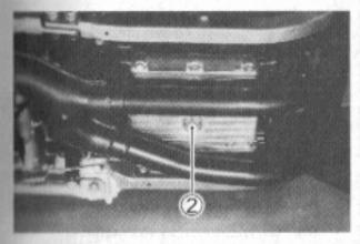
After removing the drain plug 2 from the bottom of the engine, drain the engine oil.
