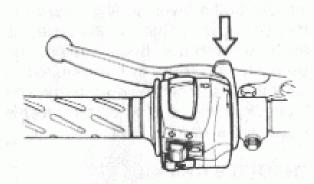
The carburetor is equipped with a choke system to provide easy starting when the engine is cold. When starting the cold engine, turn the choke lever all the way toward you. The choke works best when the throttle is in the closed position. When the engine is warm, you do not need to use the choke system for starting.
