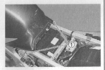
Loosen the two bolts ①. Lift up the rear end of the fuel tank.
