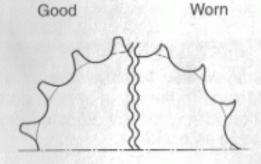
NOTE: The two sprockets should be inspected for wear when a new chain is installed and replace them if necessary.
