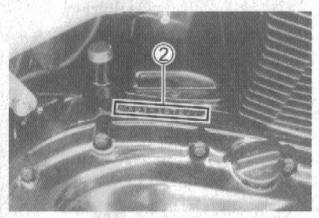
The frame and/or engine serial numbers are used to register the motorcycle. They are also used to assist your dealer when ordering parts or referring to special service information. The frame number ① is stamped on the steering head. The engine serial number ② is stamped on the crank-case assembly.
