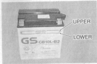
The battery is located under the seat. The solution level must be kept between the UPPER and LOWER level lines at all times. If the solution level is below the LOWER limit line, add ONLY distilled water up to the UPPER limit line. NEVER use tap water.
