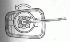
Turn the socket counterclockwise and remove it.
