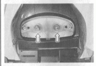
Push in the bulb, twist it to the left and pull it off.
