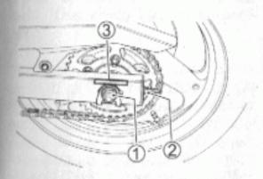
Check the drive chain slack at the middle between the two sprockets. The chain may require more frequent adjustment than periodic maintenance depending on your riding conditions.
