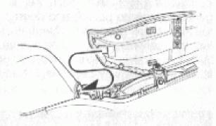
To unlock the seat, insert the ignition key into the lock and turn it clockwise. To lock the seat, slide the seat hook into the seat hook retainer and push down firmly.
