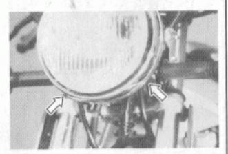
Remove the two screws from the headlight outer ring.
