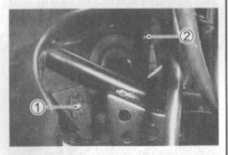
To adjust the beam horizontally: Turn the adjuster ① clockwise or counterclockwise.
