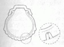
Check the condition of your tires each day before you ride. Replace tires if tires show visual evidence of damage, such as cracks or cuts, or if tread depth is less than 1.6 mm (0.06 in) front, 2.0 mm (0.08 in) rear.
