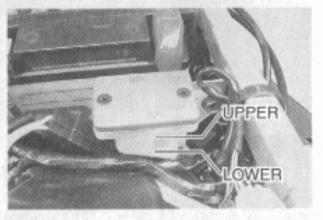
Check the brake fluid level in both the front and rear brake fluid reservoirs and inspect for brake pad wear and leaks.
