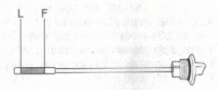
Check the engine oil level with the engine oil dipstick. The dipstick comes out together with the oil filler cap as shown. The level on the dipstick should be between the "L" (Low) and "F" (Full) lines.
