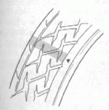
NOTE: The "Triangle mark" indicates the place where the wear bars are molded into the tire. When the wear bars contact the road, it indicates that the tire wear limit has been reached.
