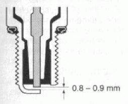
Adjust the spark plug gap to 0.8 – 0.9 mm (0.031 – 0.035 in) by using a spark plug gap thickness gauge. The spark plug should be replaced every 12000 km (7500 miles).
