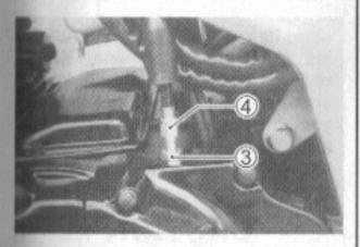
Loosen the lock nuts ③ and relocate the adjuster ④ to obtain the correct play.
