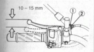
The play of the clutch lever should be 10 - 15 mm (0.4 - 0.6 in) as measured at the clutch lever end. If you find the play of the clutch incorrect, adjust it in the following way:
