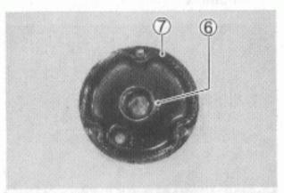
Before replacing the oil filter cover, be sure to check that the filter spring 6 and the "O" ring 7 are installed correctly.
