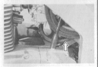
Inspect the fuel hose for damage and fuel leakage. If any defects are found, the fuel hose must be replaced.
