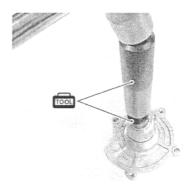
· Apply grease to the impeller shaft.
