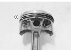
• Apply a small quantity of MOLYBDENUM OIL SOLUTION to the sliding surface of the pistons and cylinder walls.
