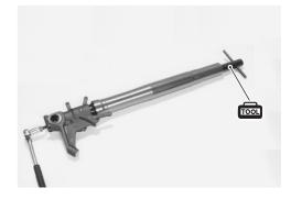
• Remove the inner rod/damper rod (cartridge) 1 .
