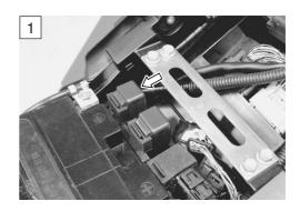
Is the cooling fan relay OK?
