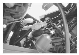
Connect proper lead wires to the fuel pump lead wire coupler (fuel pump side) and apply 12 V to the fuel pump (between Y/R wire and B/W wire) for 10 seconds and measure the amount of fuel discharged.
