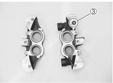
• Place a rag over the pistons to prevent it from popping out and then force out the pistons using compressed air.
