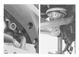
• Install the muffler chamber and mufflers . (276-16)
