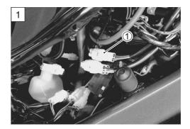
STP sensor input voltage: 4.5 - 5.5 V ( $\oplus$  R -  $\bigcirc$  Ground) ( $\oplus$  R -  $\bigcirc$  B/Br)
