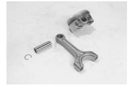
$\bullet$  Remove the piston pin circlip (1).
