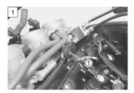
4) Disconnect the ISC valve coupler and ECM couplers.
