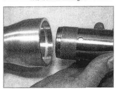
7.20a Slide the tube into the slider
