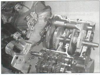
23.16 ... then assemble the crankcase halves
