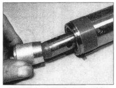
7.19b Fit the seat to the bottom of the damper rod
