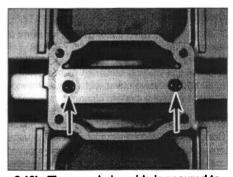
8.13b The camchain guide is secured to the valve cover by two screws (arrows)
