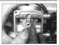
9.3c The main jet screws into the bottom of the needle jet
