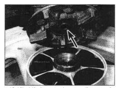
16.13b Lift the sprocket coupling out of the wheel, noting the inner spacer (arrow)
