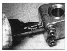
7.20b Apply thread locking compound to the damper rod bolt and use a new sealing washer
