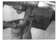
11.3a Note how the front screw secures the choke cable retainer plate
