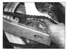
15.4a Slip the chain off the sprocket and remove the wheel
