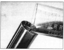
7.25a Pour the oil into the top of the tube
