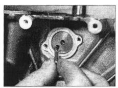
22.9a Install the spring and plunger . . .
