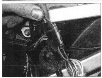
23.2 Sidestand switch wiring connectors
