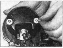
16.3a Unscrew the nuts to free the meter from the casing
