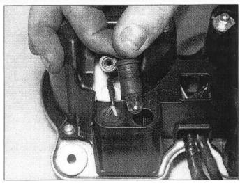
17.2a Pull the bulbholder out of the casing . . .
