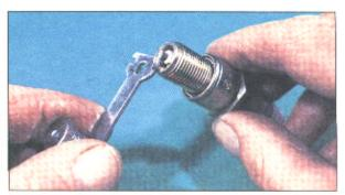
Electrode gap adjustment – bend the side electrode using the correct tool
