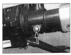
5.8 Clutch lever assembly bracket pinch bolt (arrow)
