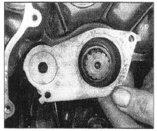
23.22a Install the output shaft retainer plate . . .
