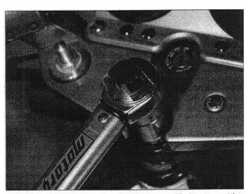
16.8 Tighten the steering stem bolt to the specified torque setting
