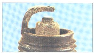
Worn plug - Worn electrodes will cause poor starting in damp or cold weather and will also waste fuel
