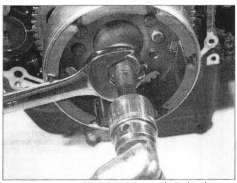
33.6c ... and tighten it until the rotor is displaced
