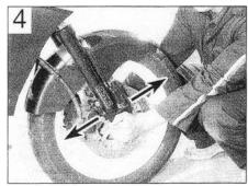
Checking the steering head bearings for freeplay
