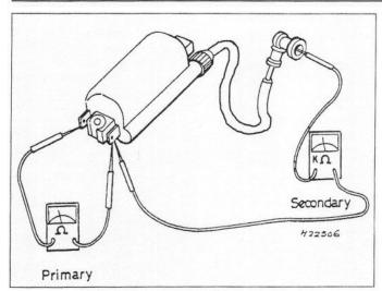
3.5 Ignition coil winding test connections
