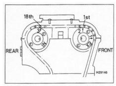
10.27 The cam chain and sprockets must be set up as shown
