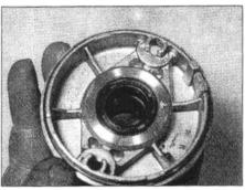
30.14 Check the oil seal in the left-hand end cover
