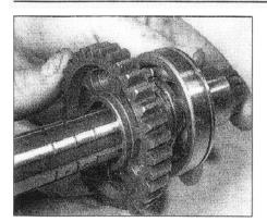
26.36a Install the 2nd gear pinion . . .
