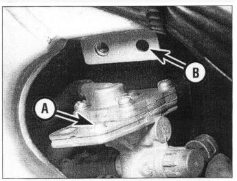
2.24 The lug (A) locates in the hole (B) in the bracket
