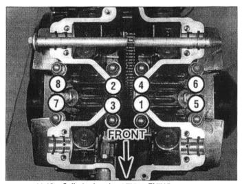
11.16a Cylinder head nut TIGHTENING sequence
