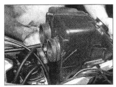
12.5 Manoeuvre the housing out of the frame
