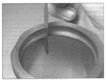
16.4 Measuring piston ring installed end gap
