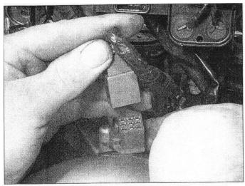
15.1 Disconnect the instrument cluster wiring connector
