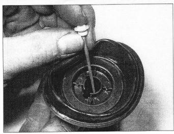
7.5 Withdraw the jet needle assembly
