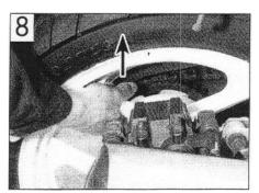
Checking for rear suspension linkage play
