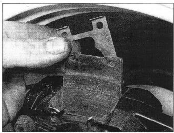
6.4 Withdraw the pads and remove the anti-chatter shims
