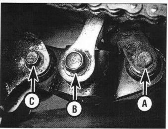
11.2b Shock absorber lower mounting bolt (A), linkage rod bolt (B), linkage arm bolt (C)
