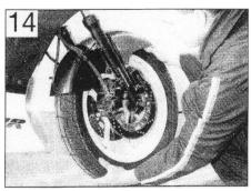
Check for wheel bearing play by trying to move the wheel about the axle (spindle)
