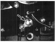
31.3 Oil pressure gauge adapter plug (arrow)
