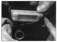
4 Ensure that the diaphragm is correctly seated before installing the plate and cover.
