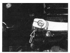
18.1a Unscrew the pinch bolt (arrow) and remove the lever
