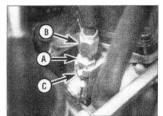
10.2a Throttle cable locknut (A), adjuster (B) and captive nut (C)
