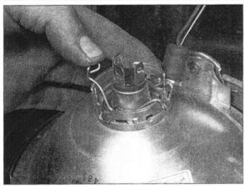
7.3a Release the bulb retaining clip . . .
