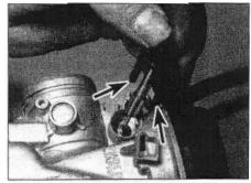
7.12b Compress the clip ends (arrows) to release the choke plunger assembly from the carburettor body
