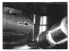
5.21 Align the mating surfaces of the clamp with the punch mark (arrow)
