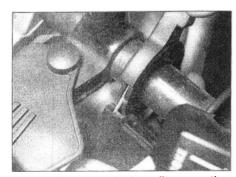
11.6a Make sure the lever fits correctly into the housing lower half
