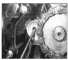
17.28a Insert the pushrod through the oil seal
