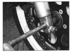
14.5 Withdraw the axle and remove the wheel
