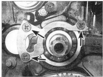
23.3 The input shaft bearing retainer plate is secured by three screws
