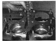
11.13a Fit the new cylinder head gasket . . .
