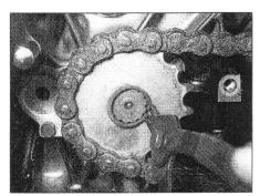
16.7c ... and retain it with the circlip
