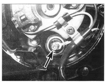
18.3 Oil pressure switch wiring connector (arrow)
