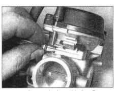
9.1b Secure the bar with the clips
