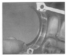
25.5a Fit the input shaft bearing retainer . . .
