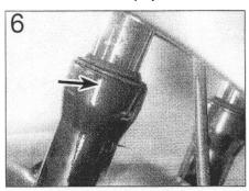
Inspect the area around the fork dust seal for oil leakage (arrow)
