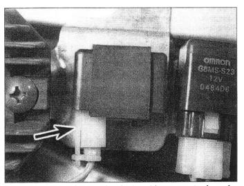
13.3 Disconnect the turn signal relay wiring connector (arrow) and check for power at the orange wire terminal
