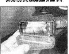
11.1b ... and remove the turn signal lens
