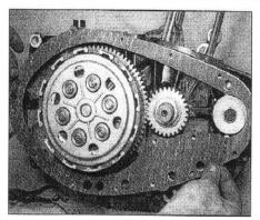
17.24 Fit a new gasket onto the crankcase
