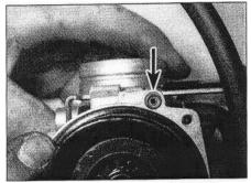
7.3 Remove the vacuum take-off pipe O-ring (arrow)
