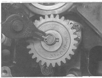
19.7d ... and secure it with the circlip
