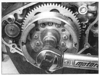
33.8c ... and tighten it to the specified torque setting
