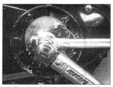
4.15c ... and tighten it to the specified torque while counter-holding the rotor
