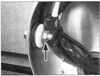
8.3a Unscrew the nut (arrow) and remove the bolt
