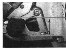
14.6a Measuring rear brake pedal height
