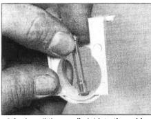
9.3a Install the needle jet into the guide
