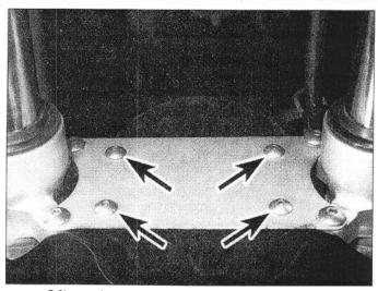
5.2b  $\dots$  then unscrew the four screws (arrows)  $\dots$
