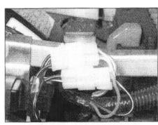
35.1b Regulator/rectifier wiring connectors
