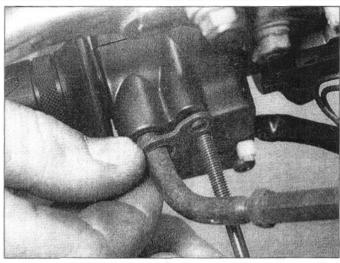
10.7b Make sure the cable retainer is secured by the screw
