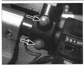
5.8 Front brake master cylinder clamp bolts (arrows)
