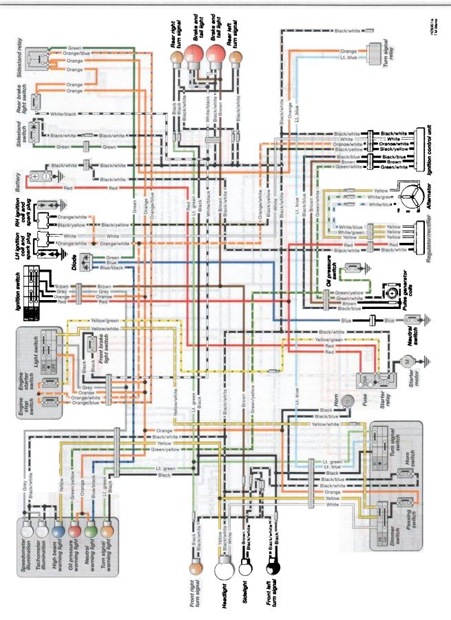
Wiring diagram - UK GS500 EL, M, N, P, R, S and T models
