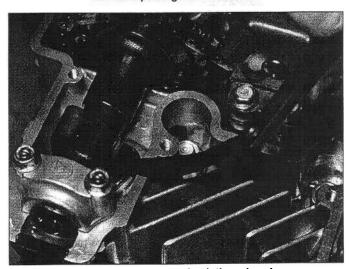
5.5c Using a feeler gauge to check the valve clearances
