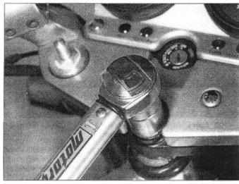
8.14 Tighten the steering stem bolt to the specified torque setting
