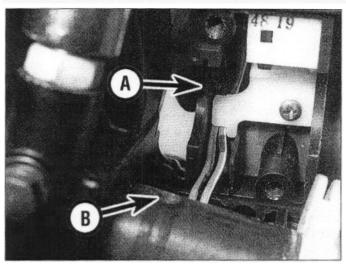
10.7a Make sure the pin (A) locates in the hole (B)
