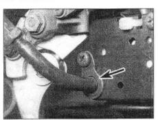
10.3a Note the throttle cable retainer plate (arrow) secured by the front housing screw
