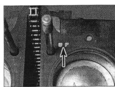
11.13b ... making sure the UP mark (arrow) reads correctly
