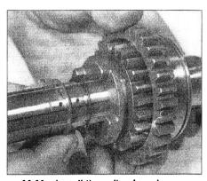
26.38a Install the splined washer . . .
