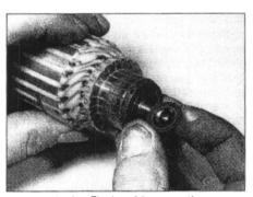
30.18a Fit the shim onto the armature shaft . . .
