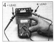
Measuring open-circuit battery voltage
