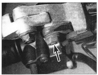
5.6a Remove the locknut (arrow) . . .
