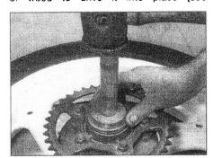
16.30 Drive the bearing seal onto the bearing
