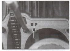
14.15b ... making sure the UP mark reads correctly
