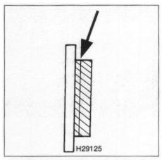
13.4 Rear brake pad wear indicator step or groove (arrow)
