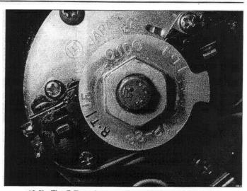
10.2b The R.T mark must align with the middle of the left-hand pulse generator coil . . .
