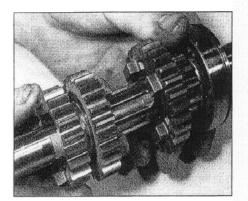
26.17 Install the combined 3rd/4th gear pinion . . .
