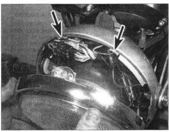
7.6 Ensure the rim fits correctly onto the tabs on the shell (arrows)
