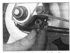
15.6 Remove the screw to free the speedometer cable from its drive housing
