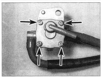
2.22 The tap diaphragm can be accessed by removing the four screws (arrows)
