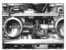
8.3 Note the arrangement of the throttle linkage assembly and various springs before disassembly
