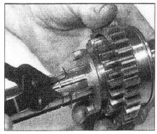
26.37b ... and secure it with the circlip
