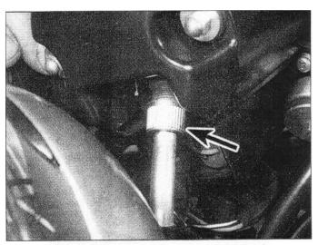
15.5 Speedometer cable retaining ring (arrow)
