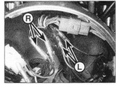
12.2 Front turn signal left (L) and right (R) wiring connectors inside headlight shell
