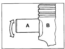
15.13a Slip the pin (A) into the piston (B). If it's loose, replace the piston and pin
