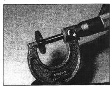
Tappet shims are measured with a micrometer
