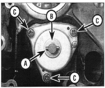
19.2b ... then slide out drive pin (A) and remove washer (B). The pump is secured to the crankcase by three screws (C)
