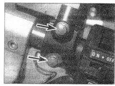
5.2 Front brake master cylinder clamp bolts (arrows)
