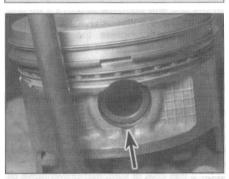
15.3a Use the notch (arrow) to aid removal of the circlip . . .
