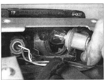
9.2 Twist the bulbholder anti-clockwise to release it from the tail light
