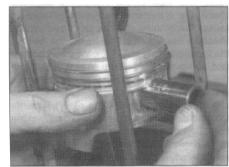
15.3b ... then push the pin out from the other side and withdraw it from the piston
