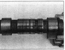
10.10b Check the lobes of the camshaft for wear - here's an example of damage requiring camshaft replacement (or repair)
