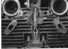
11.5 Unscrew the cylinder head front bolt (arrow)
