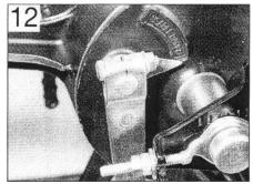
On drum brakes, check the angle of the operating lever with the brake fully applied.
