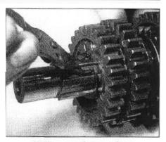
26.39c ... and secure them with the circlip
