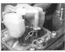
9.6a Install the float assembly using a new O-ring (arrow) . . .
