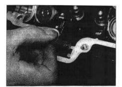
8.12 Lift the front camchain guide blade out of the engine
