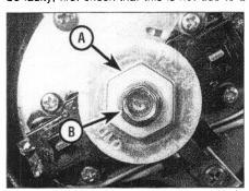
4.8 Use a spanner on the hex (A) to counter-hold the rotor, then unscrew the rotor bolt (B)
