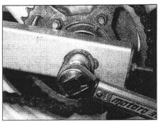
15.12 Tighten the axle nut to the specified torque setting
