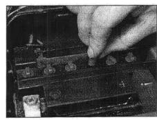
2 If the electrolyte is low the battery must be topped up with distilled water. Remove the cell caps . . .
