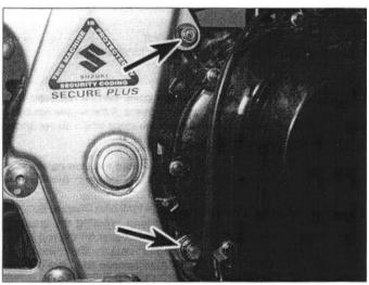
5.20 Unscrew the rear engine bolt nuts (arrows)
