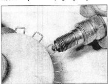
6.8a A wire type gauge is recommended to measure the spark plug electrode gap
