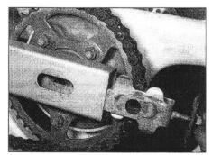
15.7 Install the chain adjusters into the swingarm
