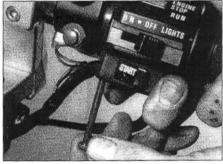
21.2 The switch is secured by two screws
