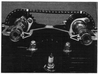
10.2c ... and the notch in the end of each camshaft must face inwards (arrows)
