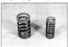
13.27 Install the springs with their closely spaced coils down (against the cylinder head)
