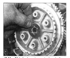
17.20c Slide lockwasher onto the shaft . . .
