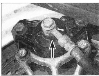
7.20 Align the hose so that it butts against the lug on the caliper (arrow)
