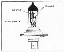
Quartz halogen headlight bulb construction
