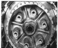
17.7 Bend back the tabs on the lockwasher to release the clutch nut
