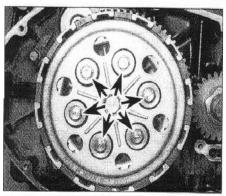
17.5b Clutch pressure plate bolts (arrows)
