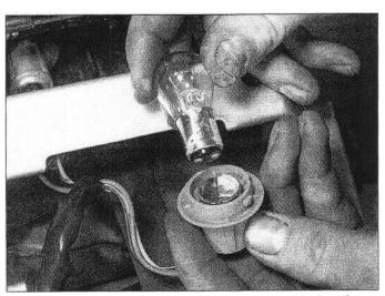
9.3 To release the bulb, gently push it in and twist it anticlockwise. Note that the pins on the bulb are offset
