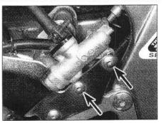
9.6 The master cylinder is secured by two bolts (arrows)
