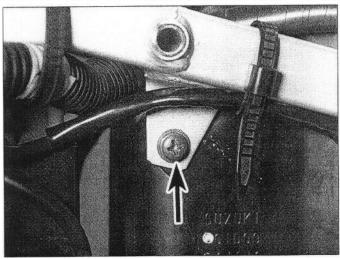
6.2a Remove the screw (arrow) on each side of the air filter housing . . .
