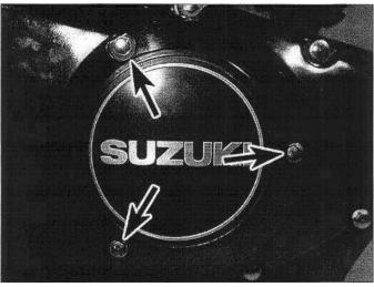
5.3 The pulse generator cover is secured by three bolts (arrows)
