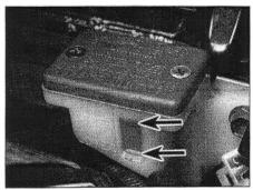
The rear brake fluid level can be seen through the translucent body of the reservoir. The fluid must lie between the LOWER and UPPER level marks (arrows).
