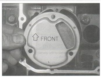
22.6 Make sure the arrow on the strainer points to the front of the engine
