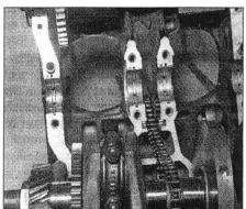
29.26a Install the crankshaft . . .
