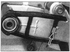
13.9 The chain slider is retained by the clip (arrow)
