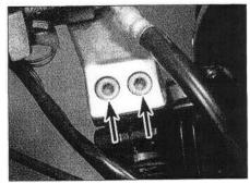
5.5 Handlebar clamp mounting bolts (arrows)
