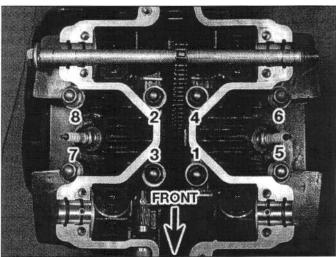
4.3b Cylinder head nut TIGHTENING sequence
