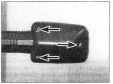
11.1a Unscrew the three screws (arrow) . . .
