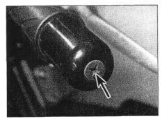
5.4 Handlebar end weight retaining screw (arrow)
