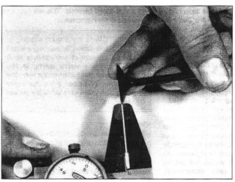
13.15 Measure the valve face thickness as shown
