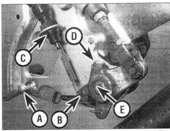
3.5 Brake pedal return spring (A), brake light switch spring (B), brake light switch retaining tabs (C), actuating arm pinch bolt (D). Note the punch mark (E)
