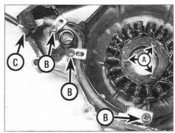
33.7 Stator screws (A), wiring clamp screws (B), wiring grommet (C)
