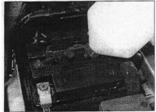
3 ... and fill each cell to the MAX level line with distilled water - do not overfill. On completion, mop up any spills and install the cell caps.
