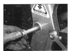
13.6b ... and withdraw the swingarm pivot bolt
