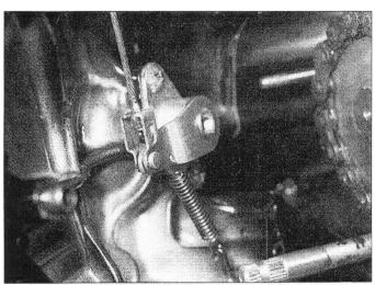
17.16a Check the release mechanism for smooth action
