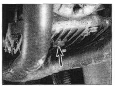
8.4a Unscrew the oil drain plug (arrow) . . .
