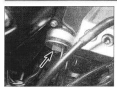
5.13 Instrument cluster mounting bolt nut (arrow)
