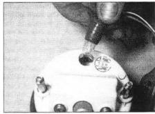
16.4b ... and remove the bulbholder
