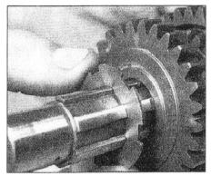
26.38c Install the inner lockwasher...
