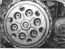
17.23a Install the pressure plate . . .
