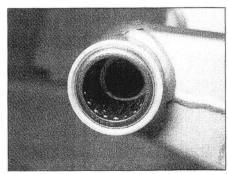
14.3d Inspect the needle roller bearings in the swingarm
