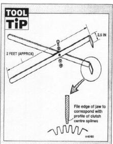
A clutch centre holding tool can easily be made using two strips of steel bent over at the ends and bolted together in the middle
