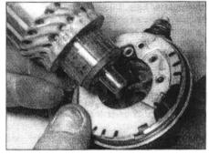
30.18b ... then install the armature into the right-hand end cover ...
