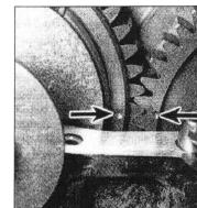
29.26b ... making sure the dot on its drive gear aligns with that on the balancer driven gear (arrows)
