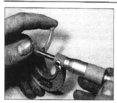
29.9 Measure the thickness of each thrust bearing
