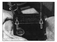
If the level is below the LOWER level mark, remove the two screws (arrows) to free the front brake fluid reservoir cover, plate and diaphragm.
