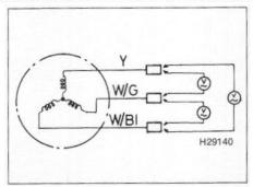
32.9 Alternator no-load voltage test connections
