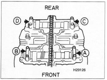
10.4 Camshaft cap identification markings
