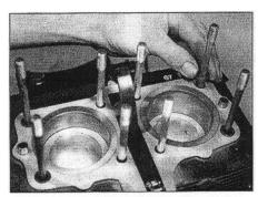
11.12 Fit a new O-ring around each stud
