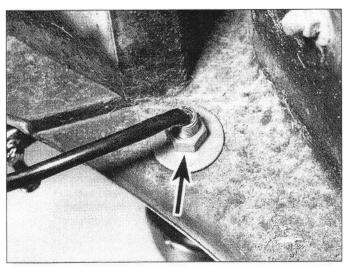
12.6 The rear turn signal assembly is secured to the mudguard by a single nut (arrow)
