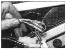
33.1 Disconnect the alternator wiring connectors
