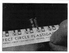
10.16 Measure the crushed Plastigauge using the scale on the pack to obtain the oil clearance
