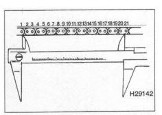
12.2 Measure distance between 1st and 21st pins to determine chain stretch
