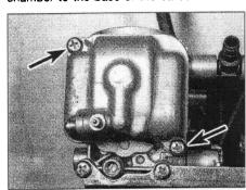
7.6 The float chamber is secured by two screws (arrows)
