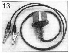
A buzzer is useful for voltage checks
