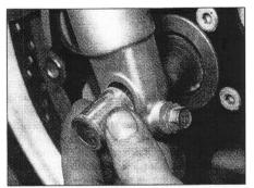
14.11b ... and the axle spacer if removed
