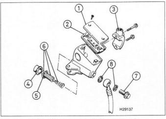
5.9 Front brake master cylinder components
