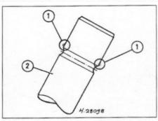
13.5c Remove any burrs (1) if the valve stem (2) won't pull through the guide
