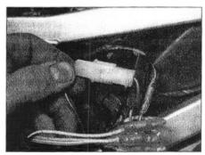
22.2 Neutral switch wiring connector
