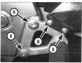
3.11 Footrest bracket mounting bolts (A), foot guard mounting bolts (B)
