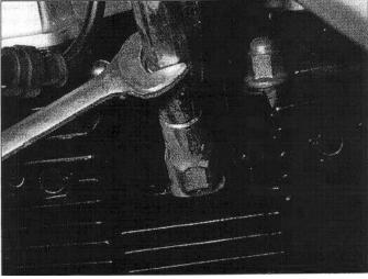
6.4a Remove the spark plug cap . . .
