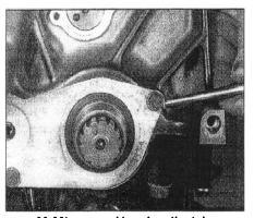
23.22b ... and bend up the tabs to lock the bolts
