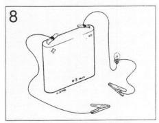
Battery and bulb test circuit
