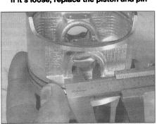
15.13c . . . the internal diameter of the bore in the piston . . .
