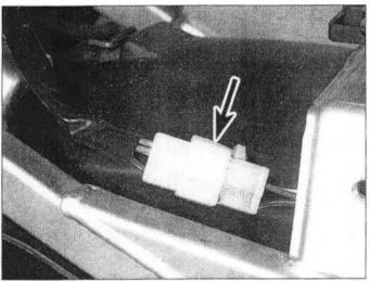
10.2 Disconnect the tail light wiring connector (arrow)
