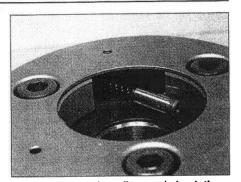
21.7 Remove the rollers and check the plungers and springs
