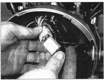
19.1 Disconnect the ignition (main) switch wiring connector
