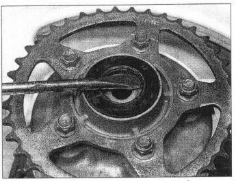
16.24b ... then lever out the bearing seal
