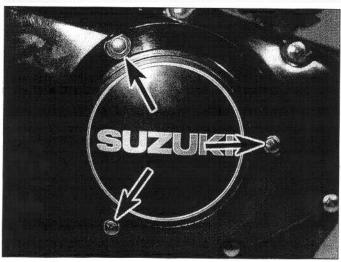
10.2a The pulse generator cover is secured by three screws (arrows)
