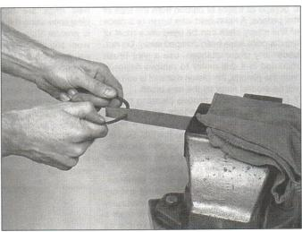
16.6 Ring end gap can be enlarged by clamping a file in a vice and filing the ring ends
