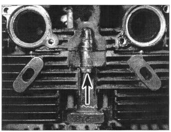
4.3a Cylinder head front bolt (arrow)
