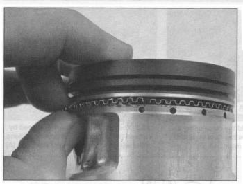
16.10a Install the oil ring expander in its groove . . .
