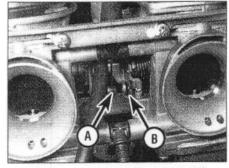
10.2c ... and detach the nipple (A) from the cam (B)
