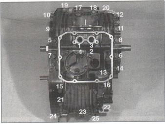
23.19 Crankcase bolt TIGHTENING sequence
