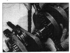
9.2 Slip the camchain off the crankshaft sprocket
