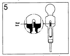
Float-type hydrometer for measuring battery specific gravity
