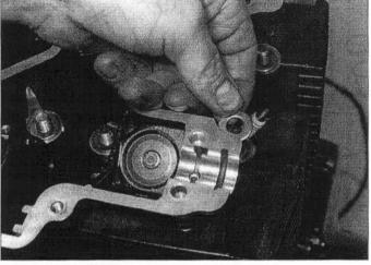
11.15a Fit new washers onto the studs . . .
