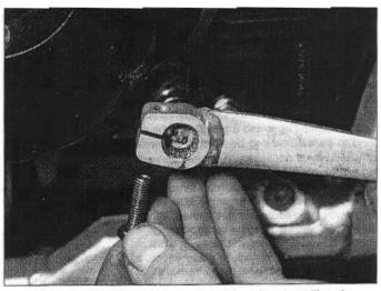
5.23c Align the previously made marks when installing the gearchange lever
