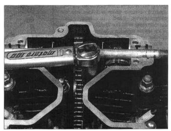
11.16b Tighten the cylinder head nuts to the specified torque...
