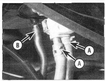
2.4b Detach the fuel hoses (A) and the water drain hose (B)
