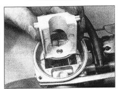
7.9 Withdraw the piston guide and needle jet
