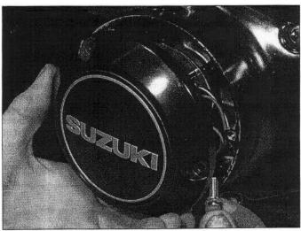
10.33 Install the pulse generator coil assembly cover
