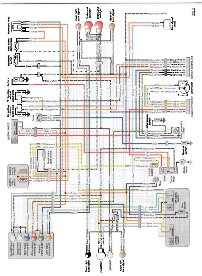
Wiring diagram - US GS500 EL, M, N, P, R, S and T models
