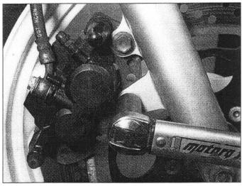
3.14b ... and tighten them to the specified torque setting
