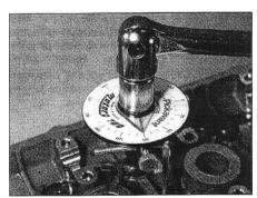
Angle-tightening cylinder head bolts
