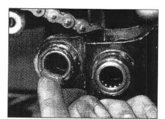
11.10 Lubricate all the bearings with grease
