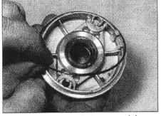
30.20a Fit a new O-ring around the left-hand end cover
