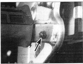
3.1 Remove the E-clip (arrow) and withdraw the pin from the top to free the footrest
