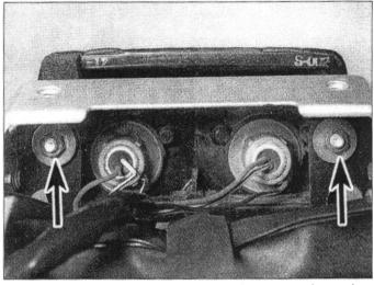
10.3 The tail light assembly is secured by two nuts (arrows)
