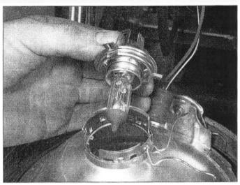
7.3b ... and remove the bulb
