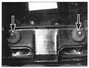
2.6 The tank bracket is secured to the tank by two bolts (arrows)
