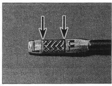
Remove the dipstick and observe the level of the oil, which should be somewhere in between the upper 'F' and lower 'L' level lines (arrows).
