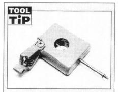
A simple spark gap testing tool can be made from a block of wood, a large alligator clip and two nails, one of which is fashioned so that a spark plug cap or bare HT lead end can be connected to its end. Make sure the gap between the two nail ends is the same as specified.
