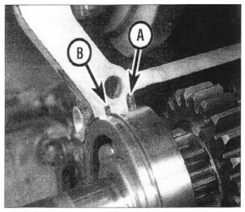
25.7b Position the bearing pin (A) against the crankcase, and make sure the half-ring retainer (B) is engaged in its slots
