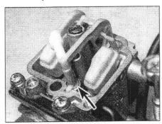
7.7a Carefully lift the float assembly out of its socket (arrow)
