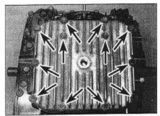
22.3 The sump (oil pan) is secured by twelve bolts (arrows)
