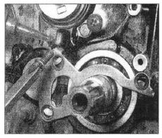
23.23b . . . applying a thread locking compound to its screws
