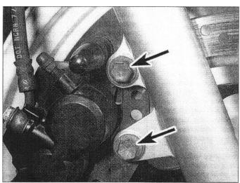
3.2a Caliper mounting bolts (arrows)
