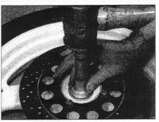
16.9 Using a bearing driver to install the bearings
