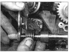
20.10a Slide the centralising spring and spacer onto the shaft . .
