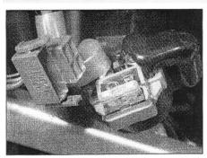
5.3a Disconnect the connector to access the fuse
