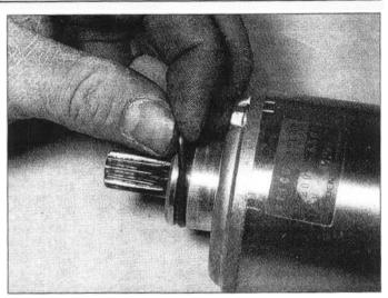
29.7 Fit a new O-ring onto the starter motor
