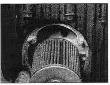
8.7a Install the new filter into the engine . . .
