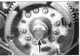
33.4 Alternator rotor bolt (arrow)
