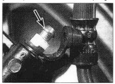
11.6 Brake caliper bleed valve (arrow)
