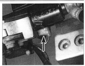
5.5 Disconnect the brake light switch electrical connectors (arrow)
