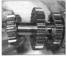
26.19a Install 2nd gear using a press . . .
