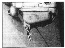
6.8 Carburettor drain screw (arrow)
