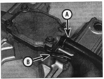
7.3 Detach the breather hose (A) and release the choke cable from its clamp (B)
