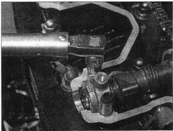
10.29c Tighten the cap bolts to the specified torque setting
