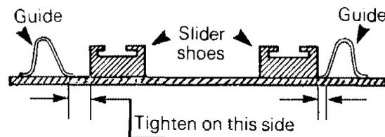
Tighten lock nuts and recheck the alignment. Ensure to retighten the idler wheel retaining screws.
