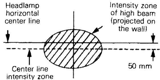
To adjust, remove the four caps, turn upper or lower adjusting screws to obtain desired beam position.
