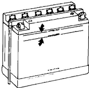
If necessary add distilled water. Battery connections must also be free of corrosion. If cleaning is necessary remove corrosion using a stiff brush then clean with a solution of baking soda and water. Rinse and dry well.
