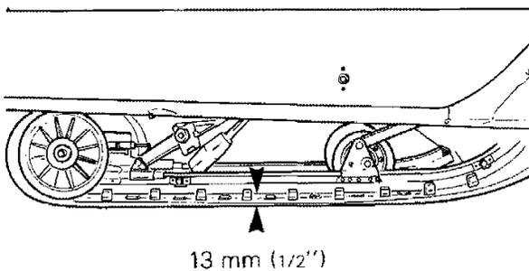
**CAUTION:** Too much tension will result in power loss and excessive stresses on suspension components.
