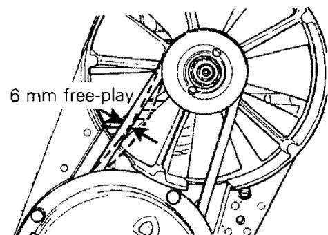
If belt seems damaged or if tension is incorrect, contact your dealer immediately.
