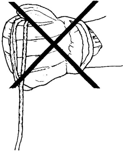
◆ **WARNING:** When starting the vehicle in an emergency situation by the drive pulley, do not make a knot at the end of the emergency rope and do not reinstall the pulley guard.
