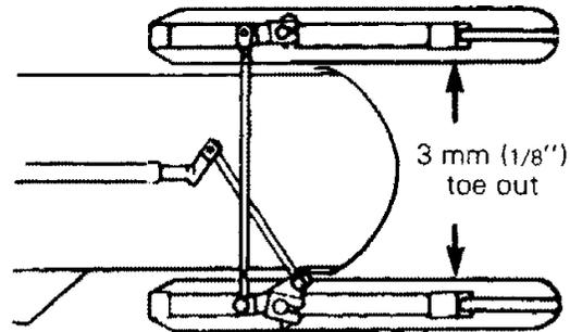
The handlebar should also be horizontal when the skis are pointed toward the front.
