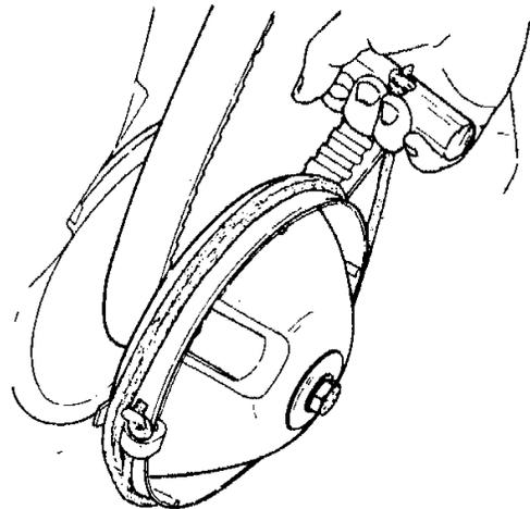
◆ **WARNING:** Do not wind starting rope around your hand. Hold rope by the handle only.
