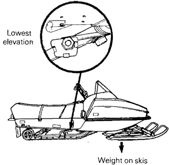
At the highest position the weight is transferred to the track. The rear adjuster blocks should be adjusted to suit the driver's preference.
