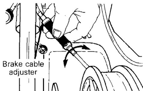
◆ **WARNING:** Whenever the brake is readjusted, the brake light switch operation must also be checked and adjusted as needed.
