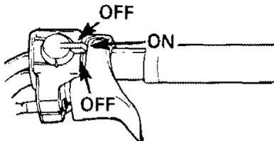
A 3 position switch located on the right side of the handlebar. To stop the engine in an emergency, flick the lever to either upper or lower "OFF" position. To start engine, lever must be in middle "ON" position.
