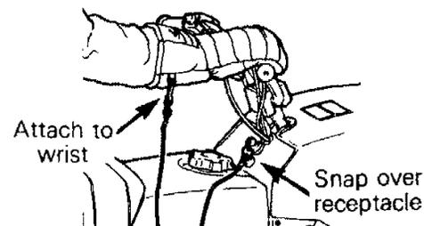
If emergency engine "shut off" is required, completely pull cap from safety switch and engine power will be automatically shut "off".
