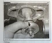
Bearing Housing and Water/Oil Pump Shaft Disassembly
