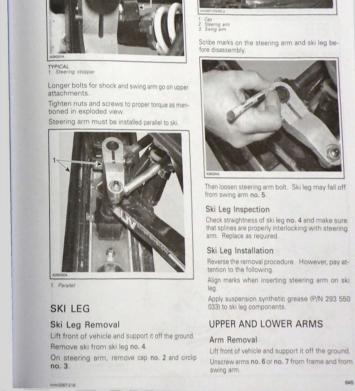
Then loosen steering arm bolt. Ski leg may fall off from swing arm no. 5. Check straightness of ski leg no. 4 and make sure that splines are properly interlocking with steering arm. Replace as required.
