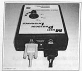
Connect remaining MPI connector to the serial port of a PC (personal computer).
