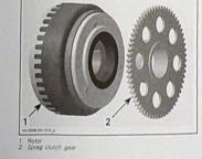
Sprag Clutch Gear Inspection Inspect gear, especially teeth and sprag clutch col-lar, for wear and other damage. Check needle bearing condition. Replace sprag clutch gear if necessary.
