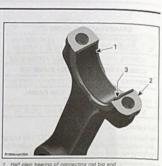
Half plain bearing of connecting rod big end Split surface of the connecting rod Nose of plain bearing in line with connecting 123 on rod o
