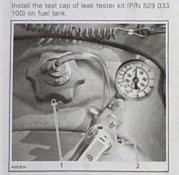
TYPICAL 1. Test cap on tank 2. Vacuum/pressure pump
