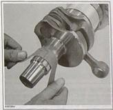
Smear Loctite 767 (antiseize lubricant) (P/N 293 800 070) on part of crankshaft where bearing fits.
