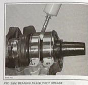
With the syringe, fill the outer ball bearing and in-ner side of outer seal with the remaining of grease.
