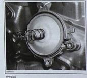
Unscrew the Allen socket screw no. 8 then re-move the RAVE valve base no. 6.
