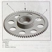
Sprag Clutch Gear Installation The installation is the reverse of the removal pro-cedure. NOTE: Apply engine oil on needle bearing and col-lar of sprag clutch gear.
