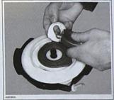
Install collar sleeve no. 10 with its collar first. Lu-bricate a new O-ring no. 11 and lock lever no. 12 with Molykote PG 54 (P/N 420 899 763). Install over pavil lock.
