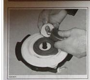
Install collar sleeve no. 10 with its collar first. Lubricate a new O-ring no. 11 and lock lever no. 12 with Molykote PG 54 (P/N 420 899 763). Install over pawl lock.
