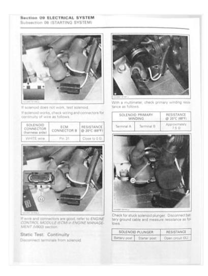
If voltage is out of specification, replace spleneed If solenoid tests good, check the electric starter Properly reinstall removed parts.
