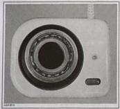
**CAUTION:** Bearing should not be heated to more than 80°C (176°F). Do not heat bearing with direct flame or heat gun or heated oil. Inappropriate heating procedure(s) may cause inner seal failure.
