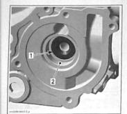
TYPICAL 1. Oil seal behind the rotary seal 2. Rotary seal bore
