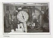
If pressure drops, it indicates a defective crank-shaft inner seal or a defective oil seal either on water pump side or oil pump side.
