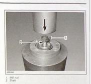
CAUTION: When removing water/oil pump shaft, always replace ceramic seal no. 9 and oil seal no. 10. Ceramic seal cannot be removed without damage. Pry inner part of ceramic seal no. 9 out.
