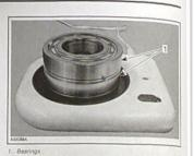
Touch the inner race of the bearing with the tem-perature indicator stick (P/N 529 035 970). Stick will liquefy when the bearing reach the proper temperature.
