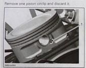
NOTE: The removal of both piston circlips is not necessary to remove piston pin. Push piston pin out of piston.
