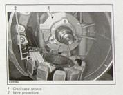
NOTE: During installation, make sure the stator harness is located on the left side. Apply Locitie 243 (blue) (P/N 293 800 060) on threads of stator screws then torque them to 7 N•m (62 lbf•in). Reinstall all other removed parts.
