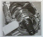
BALLS COATED WITH A SEAM OF GREASE
