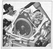
1. Marks on camshaft timing gear 2. Cylinder head base 3. Camshaft locking tool
