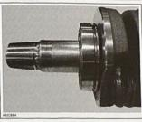
BEARING TO END POSITION Install the O-ring.
