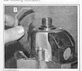
Centrifugal Weight Calibration Use the following table to calibrate this drive clutch properly.
