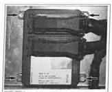
Install the new ECM to the vehicle. Reconnect connectors to ECM, and then battery cables.
