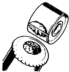
Fig. F11 Failed suspension unit with ferrule detached
