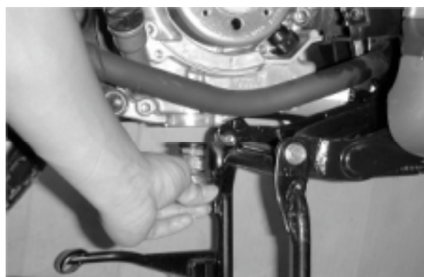
Oil Filter Screen Cap
