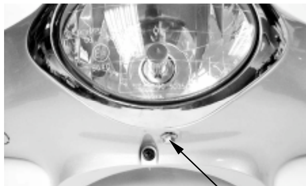
Headlight Aim Adjusting Bolt
