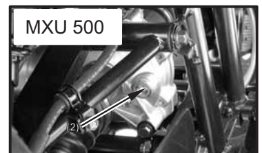
(2) Oil filler bolt/washer
