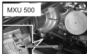
(1) Oil drain plug/washer
