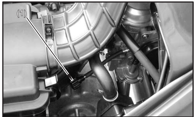
(1) Idle adjusting screw (MXU 500)
