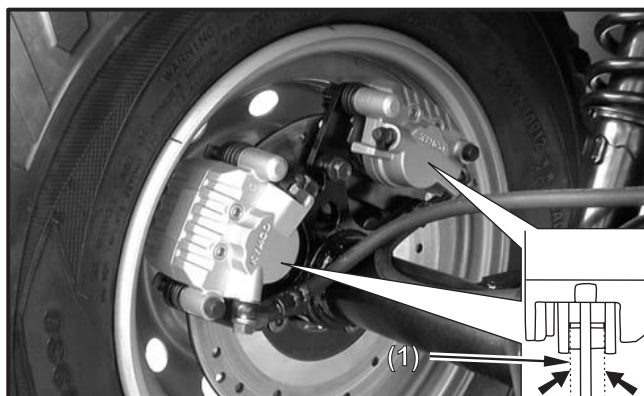
(1) Wear indicator (2) Rear brakes MXU 500 version
