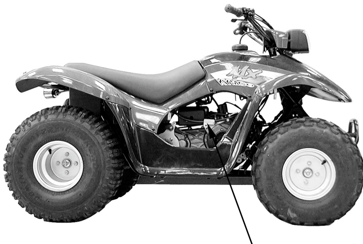
Location of Frame Serial Number
