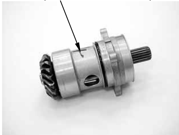
Secondary Driven Bevel Gear Assembly
