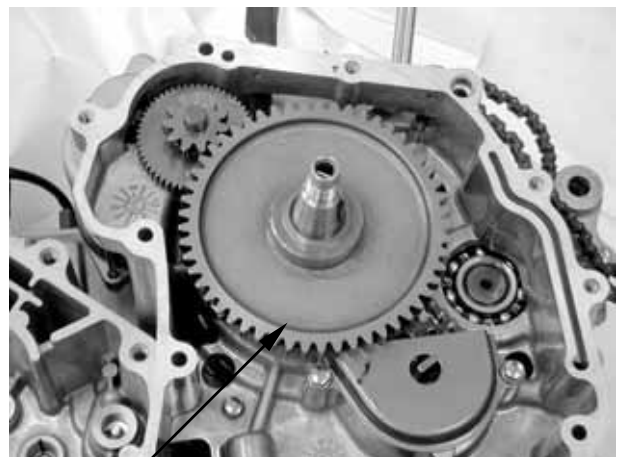
Starter Driven Gear
