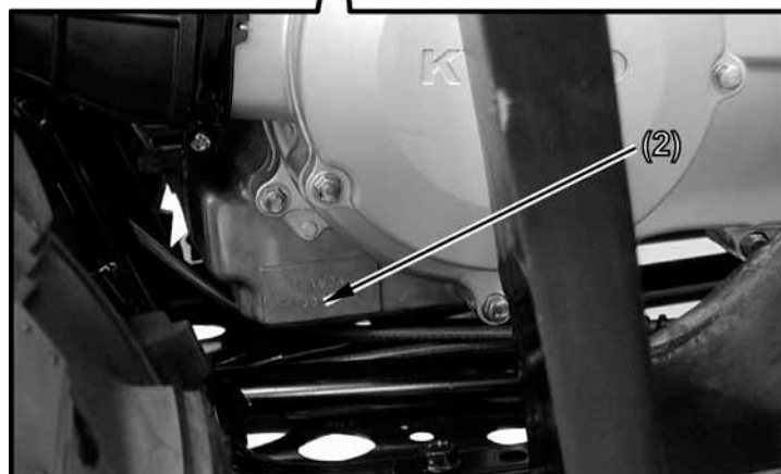
(2) Location of Engine Serial Number
