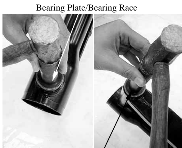
Bearing/Dust Seal
