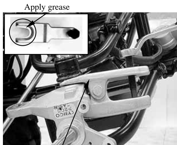
Ball Joint Remover
