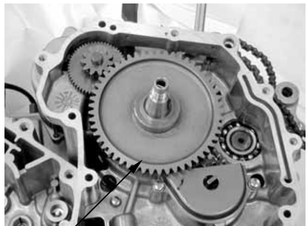
Starter Driven Gear
