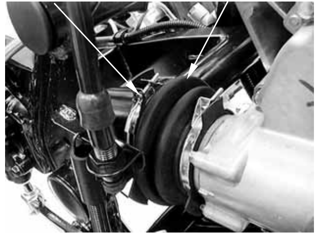
Screw (Only swingarm side) Joint Boot
