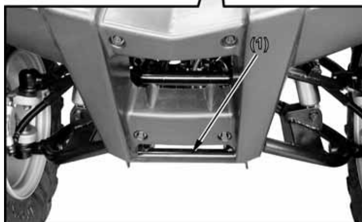
(1) Location of Frame Serial Number
