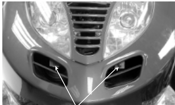
Headlight Aim Adjusting Bolt
