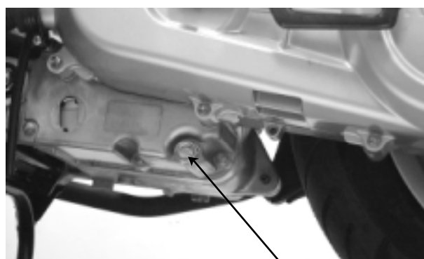
Oil Drain Bolt
