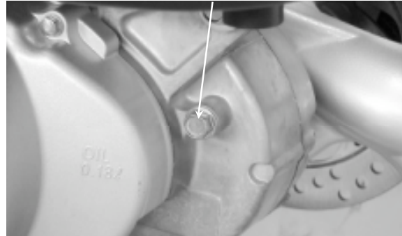
Oil Check Bolt Hole/Oil Filler
