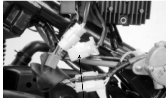
A.C. Generator Connector
