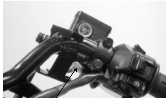
Stop Switch Wire Connector
