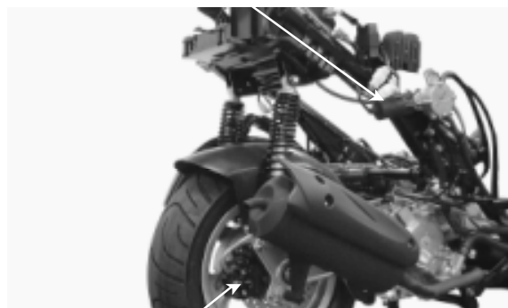
Rear Brake Caliper
