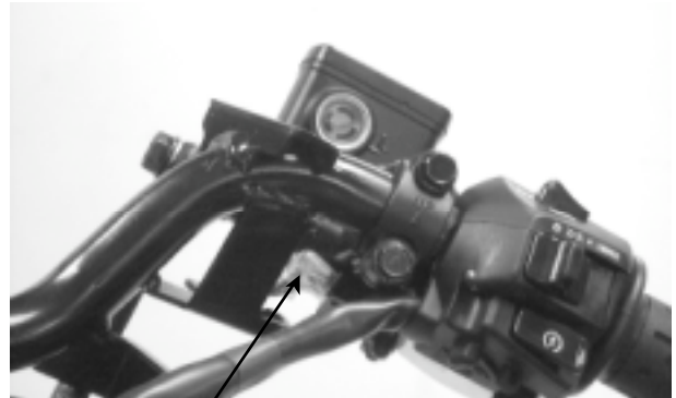
Stop Switch Wire Connector
