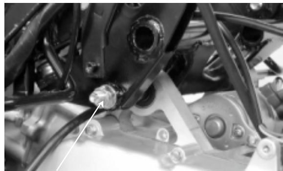
Engine Hanger Bolt
