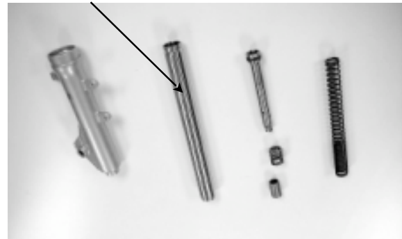
Shock Absorber Tube
