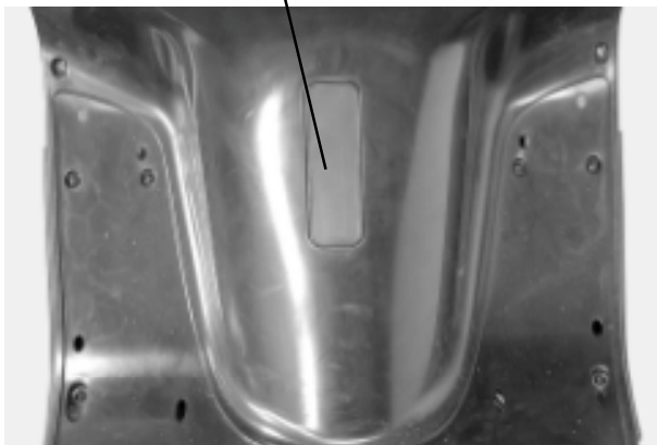
Location of Frame Serial Number
