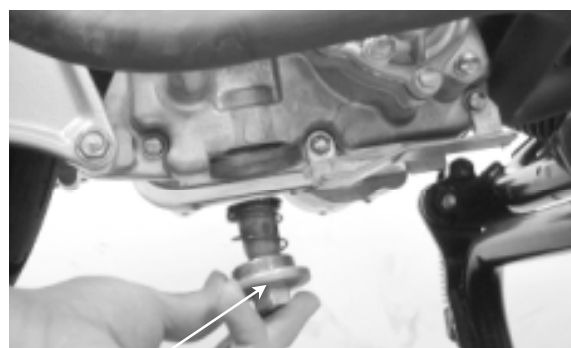
Oil Filter Screen Cap
