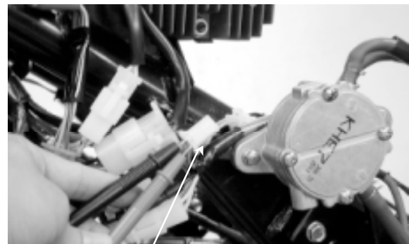
Pulser Coil Wire Coupler
