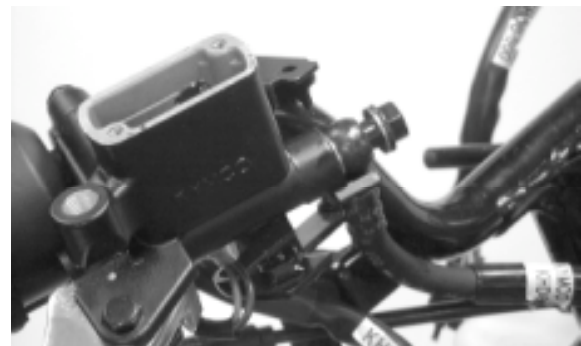
Stop Switch Wire Connector
