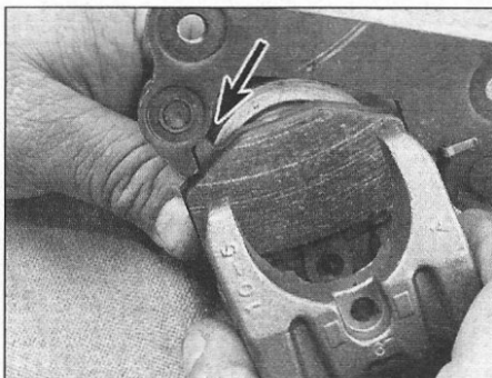
6.8 Make sure the outer pad locates correctly against the bracket (arrowed)
