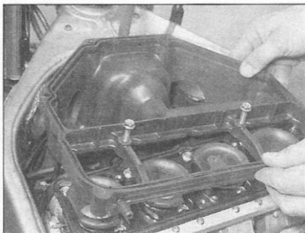
4.3b ... and remove the housing
