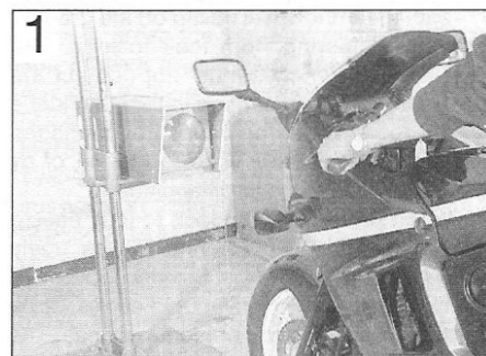
Headlight beam height checking equipment
