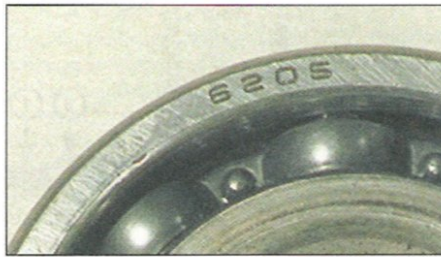
5.16 Typical bearing marking
