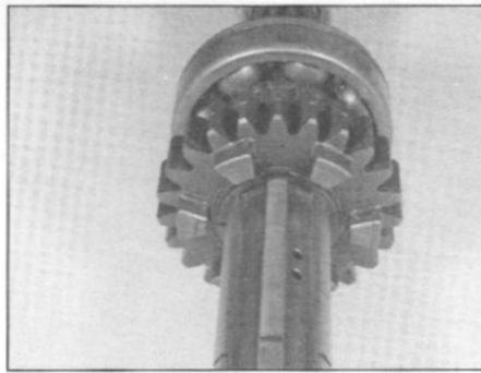
31.7a Remove the circlip ...
