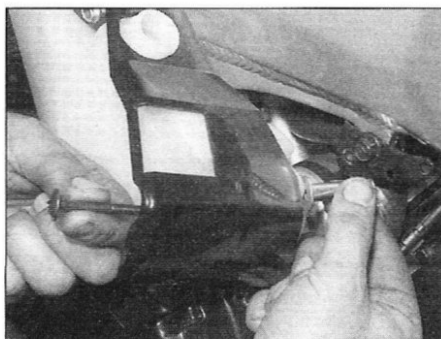
3.3b . . . noting how the cover and collar fit on F models . . .
