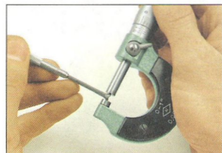
3.10 ... then measure the gauge with a micrometer
