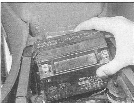
3.3b ... and remove the battery
