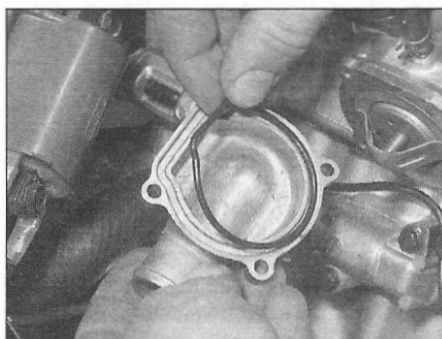
6.8a Fit a new O-ring into the cover . . .
