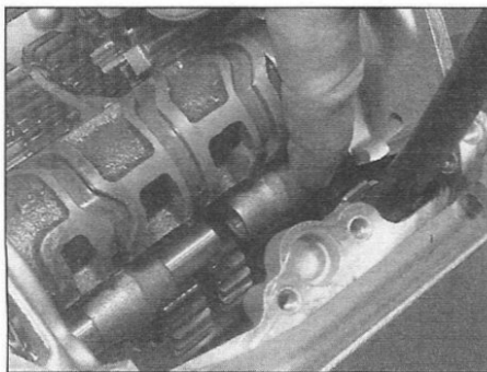
30.14a Slide the shafts through the forks . . .
