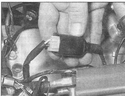
4.2 Disconnect the pick-up coil wiring connector ...
