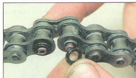
8.5 ... install the O-rings over the pin ends ...
