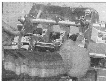
23.8b . . . separate the crankcase halves
