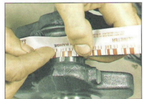
3.16 Measuring the width of the crushed Plastigauge
