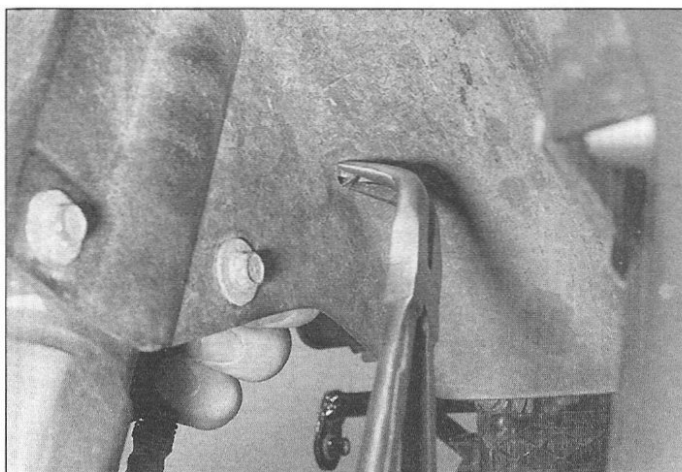
7.1a Squeeze the clips on the inside to release them
