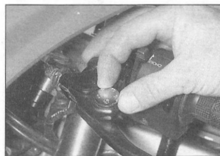
7.6 Pull the lever away from the handlebar and adjust the dial as required – F, G and H models
