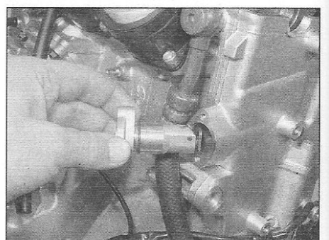
8.10b ... then install the tensioner ...
