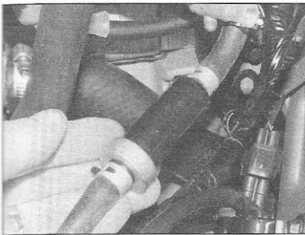
20.13 Location of the carburettor heater valve
