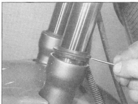
22.3 Checking for leakage of the fork seals
