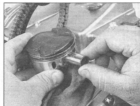
14.4b . . . then push the pin out and withdraw it from the other side of the piston
