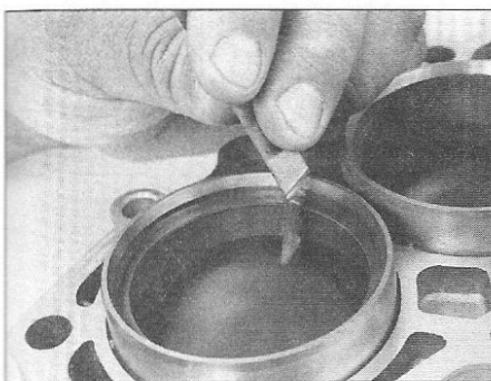
15.3 Measuring piston ring installed end gap
