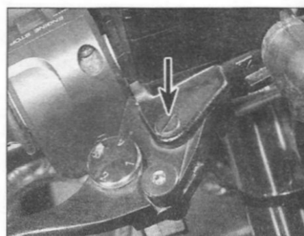
5.12b ... then unscrew the pivot bolt (arrowed) and remove the lever
