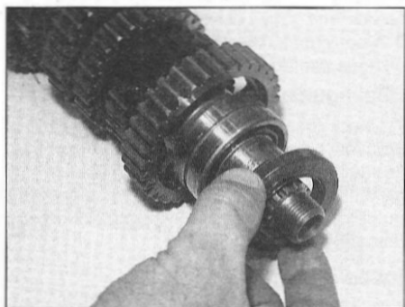
29.5 Replace the output shaft oil seal if required
