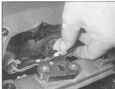
9.2 Remove the bulbholder from the tail light ...
