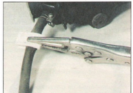
9.4 ... or thick card and self-locking grips
