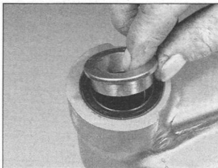
14.4a Remove the collar and cap . . .
