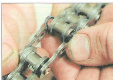
8.3 ... and separate the chain link
