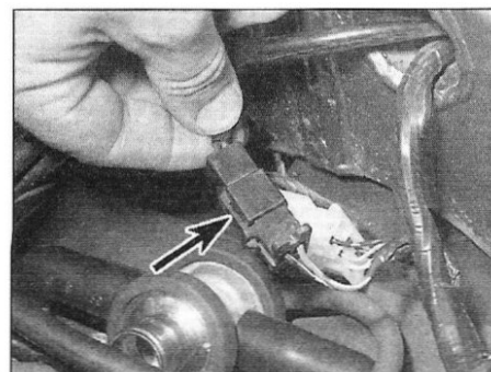
4.3a Fan motor wiring connector (arrowed) – F, G and H models
