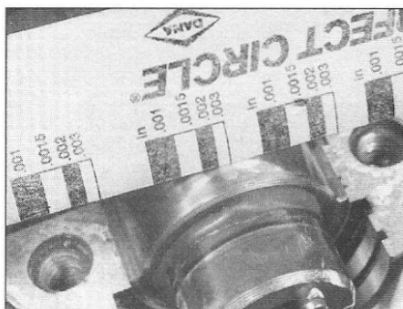
26.12 Measure the width of the crushed Plastigauge
