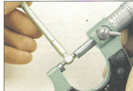
3.8 ... then measure the gauge with a micrometer
