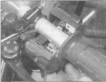
11.3b ... and separate the halves
