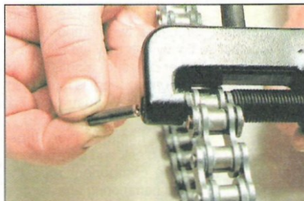
8.2 ... withdraw the pin, remove the tool ...
