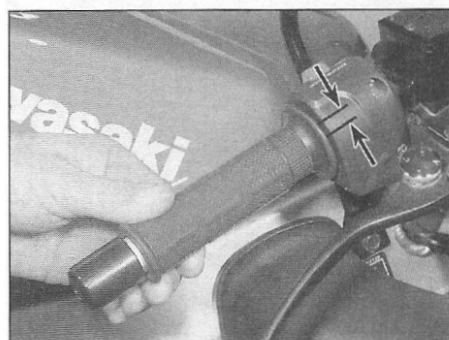
18.3 Check the amount of freeplay in the twistgrip
