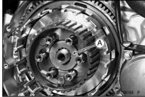
● Pile up the four torque limiter springs [A] so that the spring tongues [B] do not face the same direction in the sub-clutch hub [C].
