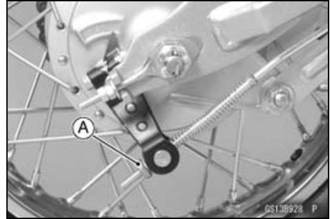
***Brake Lining Wear Inspection***
