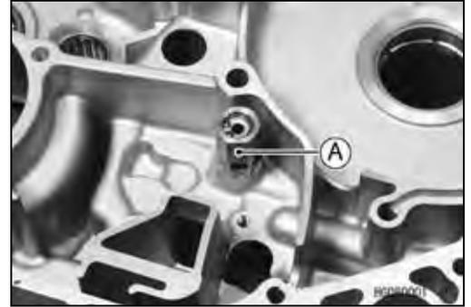
*Oil Pressure Relief Valve Installation*
