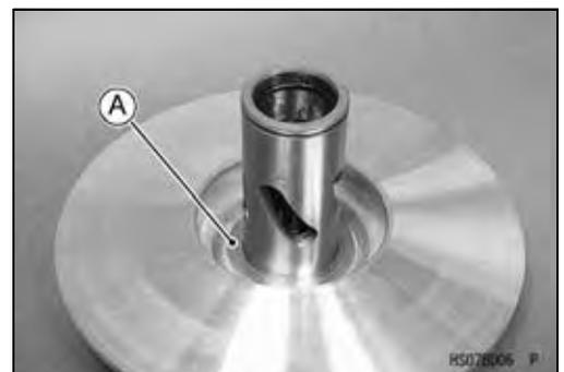
● Apply grease to the oil seal lips [A].
