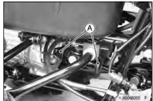
*Rear Axle/Stabilizer Joint Boot Inspection*
