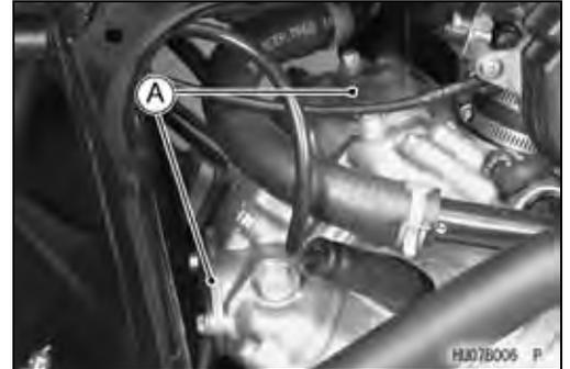
● Remove the timing inspection plug [A].
