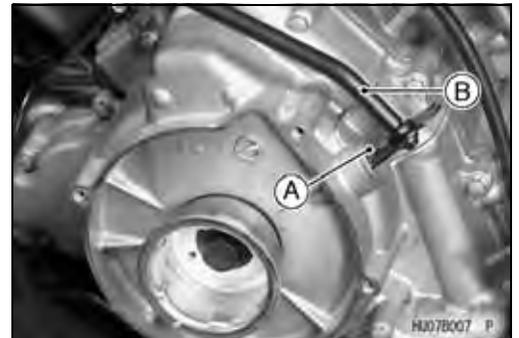
● Turn the crankshaft **counterclockwise** with a wrench on the alternator rotor bolt until "T-F" mark [A] on the alternator rotor aligns with the notch [B] as shown: the end of the compression stroke in the front cylinder head.
