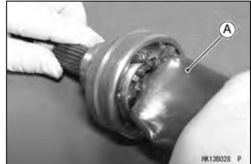
● Tap the shaft end [A] straight with a plastic hammer until it is locked by the circlip.
