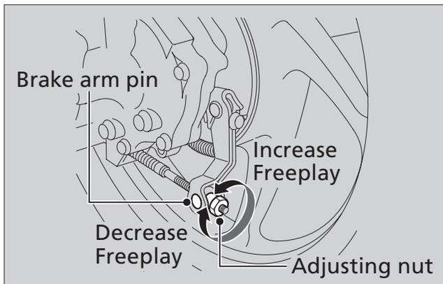
2. Apply the brake several times and check for free wheel rotation after the brake lever is released.
