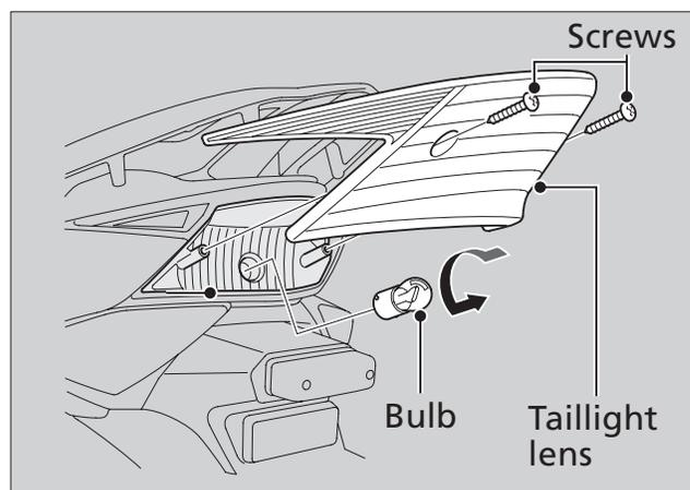
1. Remove the taillight lens by removing the screws.
