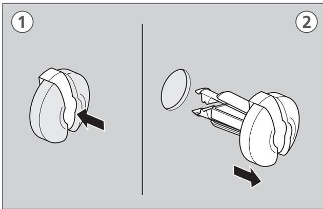
1. Press down on the centre pin to release the lock.
