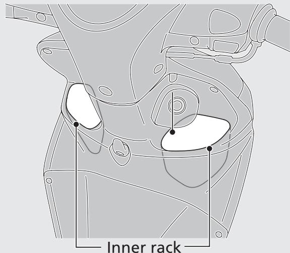
The maximum allowable load on the shopping hook and on the inner rack shall be no more than **1.5 kg (3.3 lb)**.
