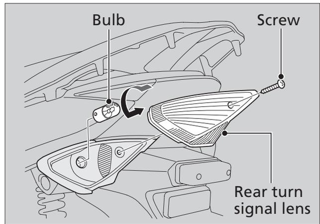
1. Remove the rear turn signal lens by removing the screw.
