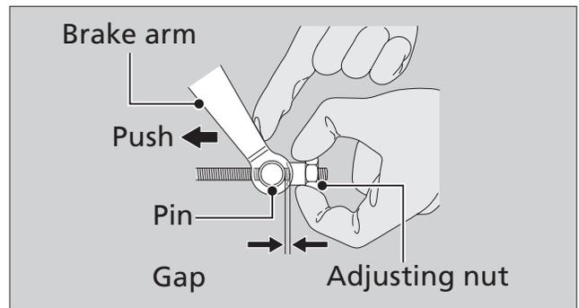
After adjustment, confirm the freeplay of the brake lever.
