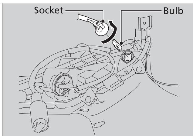
3. Turn the socket counterclockwise and pull it out.
