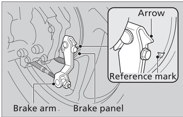
When the brake is applied, an arrow attached to the brake arm moves toward a reference mark on the brake panel. If the arrow aligns with the reference mark on full application of the brake, the brake shoes must be replaced. See your dealer for this service.
