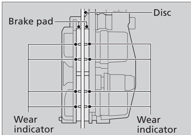
1. Inspect the brake pads from in front of the brake caliper. If necessary have the pads replaced by your dealer. Always replace both left and right brake pads at the same time.
