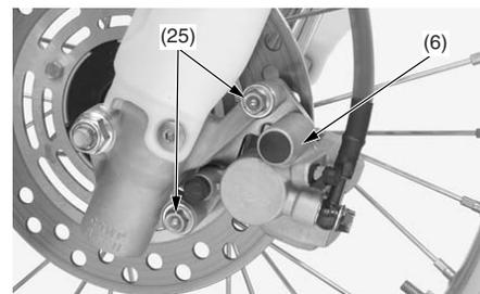
(6) caliper (25) caliper mounting bolts
