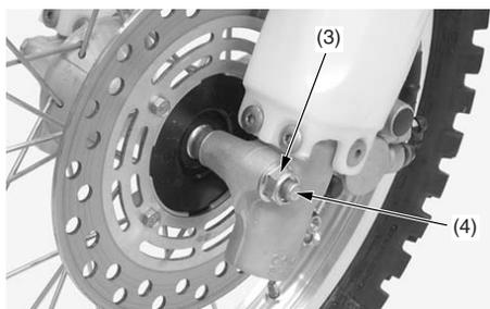
(3) axle nut (4) front axle shaft
