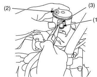
(1) piston pin (3) piston pin clip
