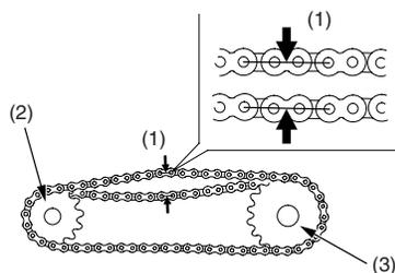
(1) drive chain slack (2) drive sprocket (3) driven sprocket
