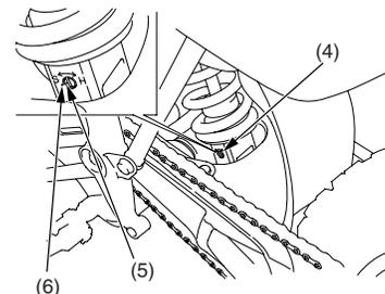
(4) rebound damping adjuster (5) punch mark (6) reference mark
