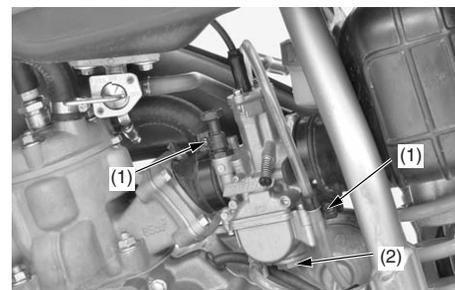
(1) connecting and insulator tube clamp screws
