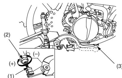
(1) lock nut (2) adjusting bolt (3) rear brake pedal
