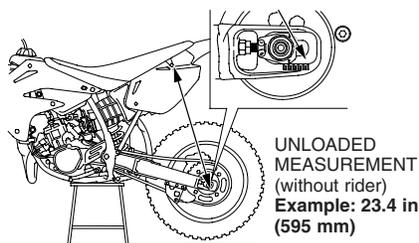
3. Measure the *loaded with rider* dimension. Remove the workstand. With two helpers available, sit as far forward as possible on your CR's seat, wearing your riding apparel. Ask one helper to steady your CR perfectly upright so you can put both feet on the pegs. Bounce your weight on the seat a couple of times to help the suspension overcome any situation and settle to a good reference point.
