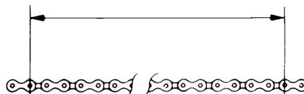
MEASURE A SPAN OF 21 PINS (20 PITCHES)
