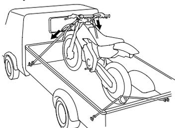
To secure your CR, brace the front wheel against the front of the truck bed or trailer rail. Attach the lower ends of two straps to the tie-down hooks on your vehicle. Attach to the upper ends of the straps to the handlebar (one on the right side, the other on the left), close to the fork.
