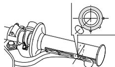
For added security, you may choose to safety wire the hand grips to the handlebar and throttle to prevent the possibility of them loosening. Position the twisted wire ends away from your palms and be sure to bend the wire ends well into the grip rubber so they will not snag your glove.
