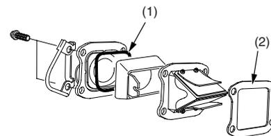
(1) insulator o-ring (2) reed valve gasket
