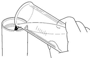
4. Raise the fork tube (2) and cover the top of the tube with your hand. Compress the fork tube fully, then release your hand. Use your other hand to secure the fork tube. Repeat this procedure 3 times.
