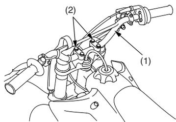
(1) handlebar (2) handlebar upper holders
