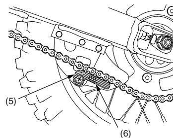
(5) chain guide slider (6) inspection window
