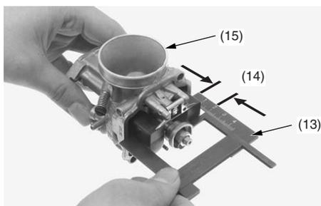
(13) float level gauge (15) carburetor intake
