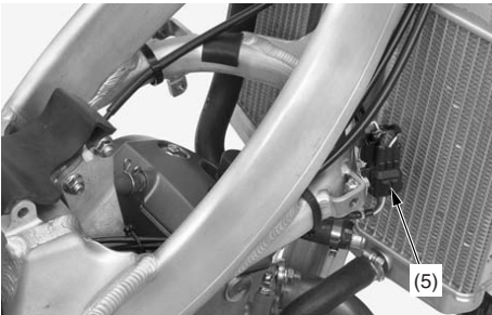
(5) throttle sensor connector
