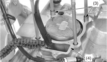
(3) dowel pins (4) cylinder gasket
