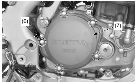
(6) clutch cover bolts (7) clutch cover
