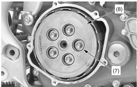
(7) clutch spring bolts/springs (8) clutch pressure plate
