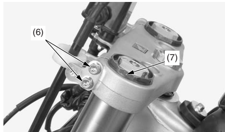
(6) upper pinch bolts (7) fork damper
