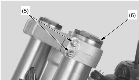
(5) upper pinch bolts (6) fork damper
