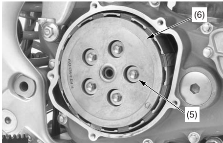
(5) clutch spring bolts (6) clutch pressure plate
