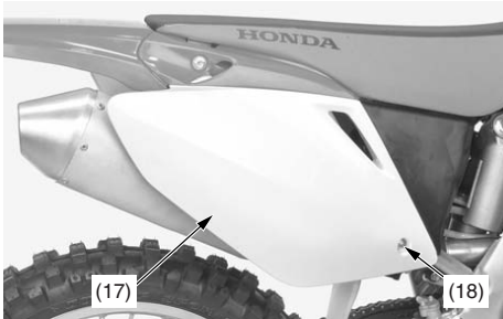
(17) side cover (18) side cover bolts/collars
