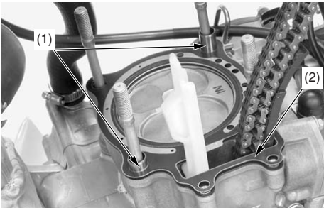
(1) dowel pins (2) cylinder head gasket
