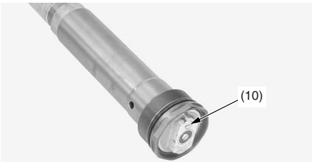
(10) pressure release screw
