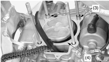
(3) dowel pins (4) cylinder gasket
