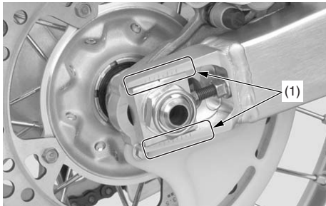
(1) chain adjuster index marks
