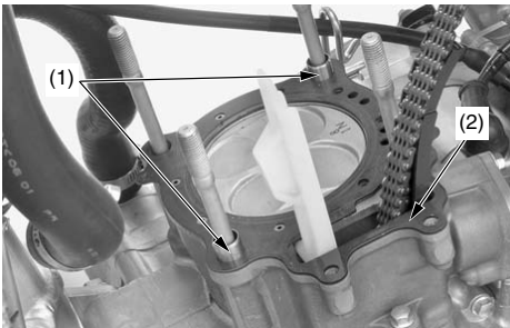
(1) dowel pins (2) cylinder head gasket
