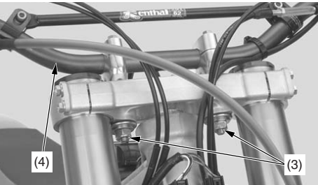
(3) washers/handlebar holder nuts (4) handlebar
