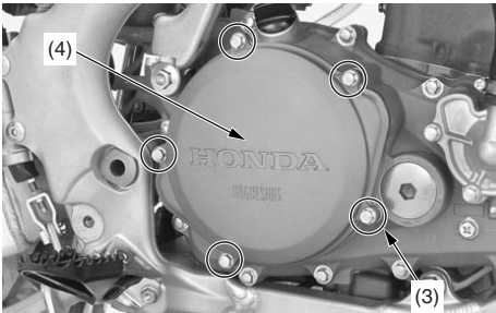
(3) clutch cover bolts (4) clutch cover
