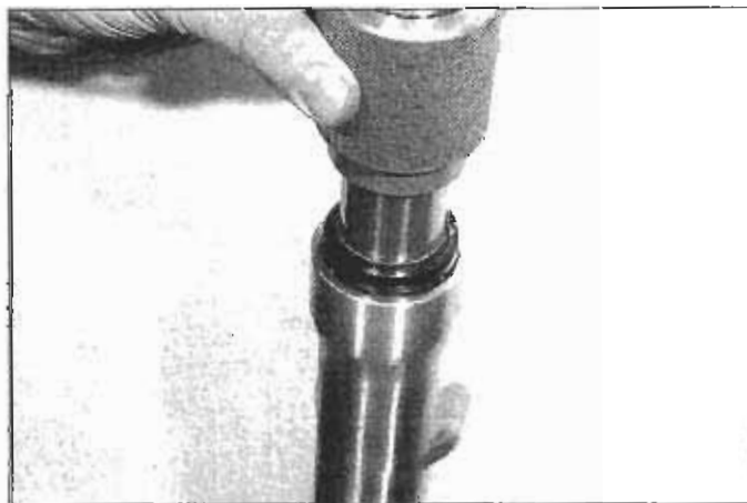
5.27 Use any of the tools previously shown to drive the dust seal into place
