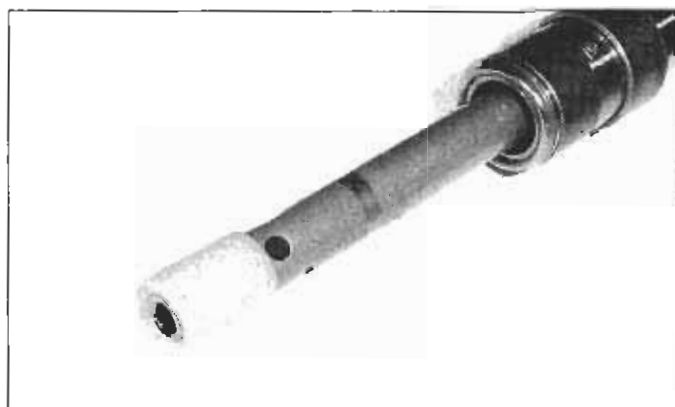
5.20 Install the lock piece on the lower end of the damper rod
