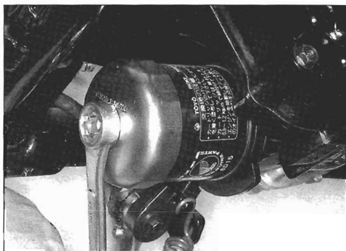
12.5b Use a filter wrench to remove the oil filter (if you don't have this type of filter wrench, use a pair of large water pump pliers)
