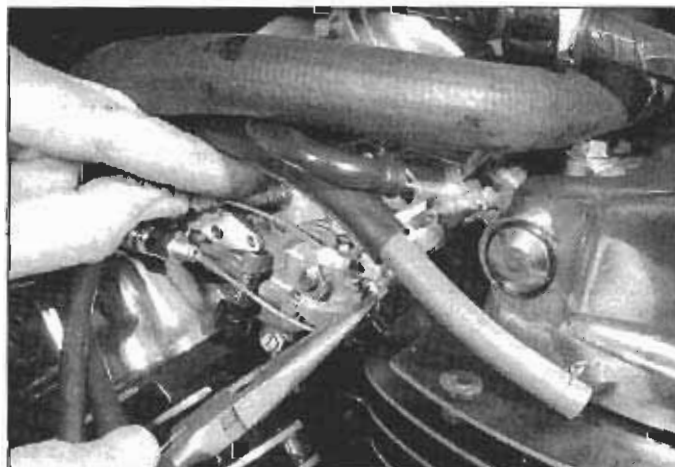
10.6 Disengage the ends of both cables from the throttle pulley
