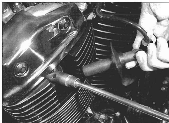
15.2 Remove the spark plug cap
