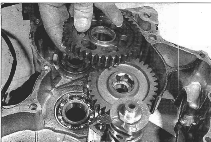
29.3h Remove the C1 gear
