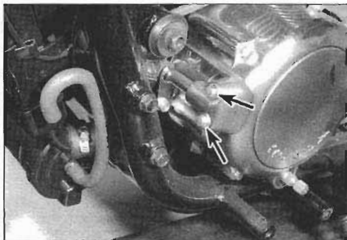
4.4 These bolts (arrows) secure the breather hose adapter to the left crankcase cover
