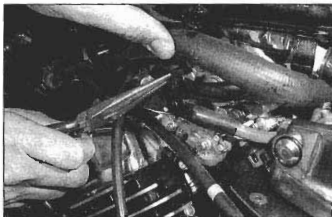
12.11b On the other side, disengage this clamp ...
