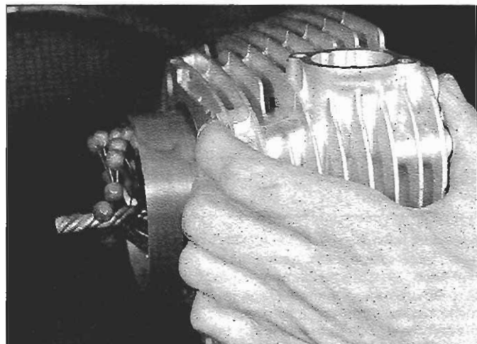
14.14 Move the hone rapidly up-and-down without stopping
