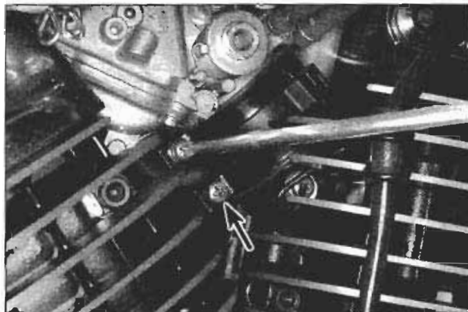
12.12a Loosen both insulator clamp screws ...
