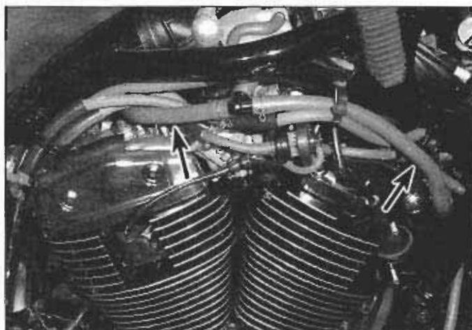
4.3 These two hoses are connected to the crankcase breather separator
