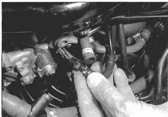
9.14b . . . and remove the SE valves (right carburetor shown)
