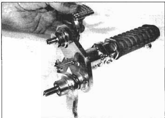
9.12 This is what the assembled footpeg bracket and rear brake pedal should look like when you're done
