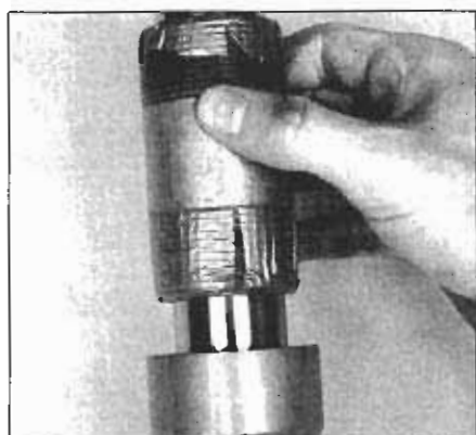
5.24c If you don't have a bushing driver, use a section of pipe instead; be sure to tape the ends of the pipe so it doesn't scratch the fork tube
