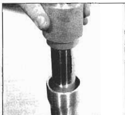
5.25c Tap the seal gently with a driver until it's fully seated in the fork slider (but don't keep hitting it after it seats or you'll damage it)
