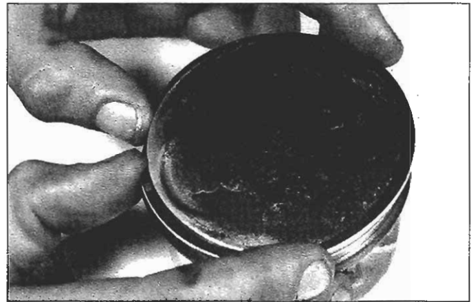
16.11a Install the middle ring with its identification mark up
