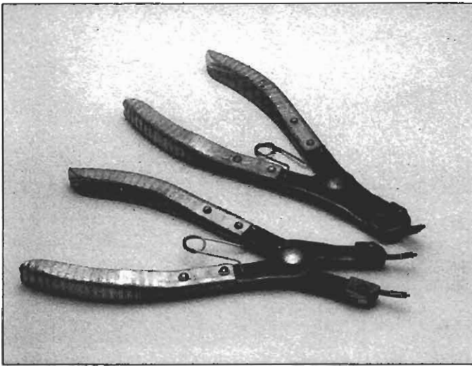
Snap-ring pliers (top - external; bottom - internal)
