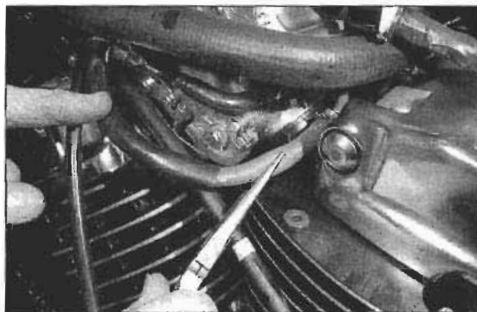
12.11c ... and detach the EVAP hose from the left (rear cylinder) carburetor
