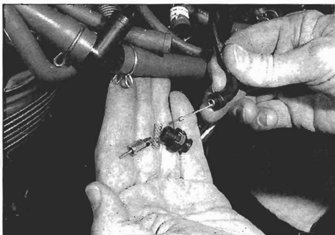
9.15 Before adjusting the choke cable, inspect the spring, valve and threaded barrel of each SE valve; replace any broken or worn pieces
