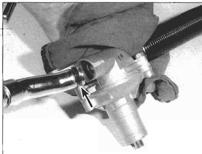
9.12 Install a new O-ring on the outlet pipe (arrow)
