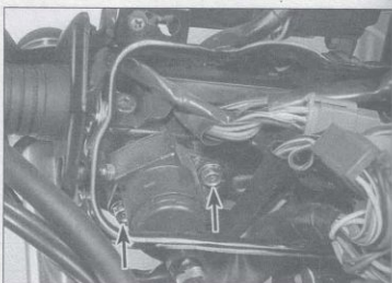
22.6 Ignition switch is retained to upper triple clamp by two bolts (arrows)
