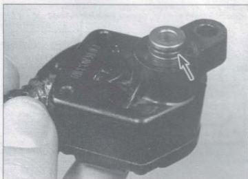
14.13 Replace the O-ring (arrow) whenever speed sensor is removed (750 Sabre)
