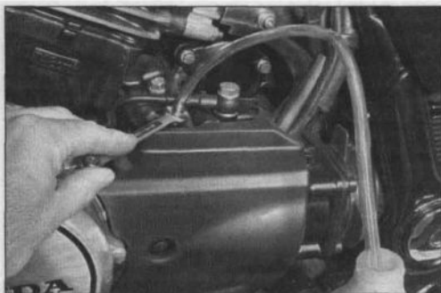
9.4 When bleeding the clutch connect tube to bleed valve as shown
