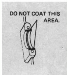
24.10 Do not apply sealant to this area of main bearing mating surfaces
