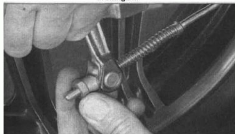
16.5 Fully unscrew the rear brake adjusting nut from the brake rod
