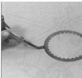
14.20 Measure clutch plain plate warpage on a perfectly flat surface
