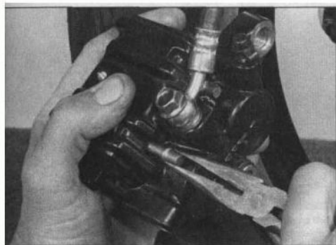
2.2c ... and pull the pins out with pliers
