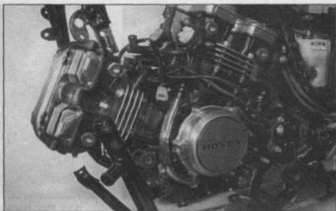
5.22 Removing the subframe
