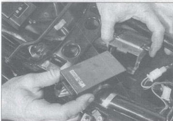
14.20 Turn signal cancel unit location on the 1982 750 Sabre
