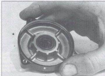
34.3 Check oil seal (arrow) and needle bearing in rear cover
