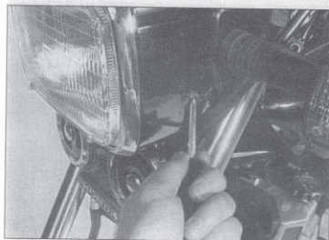
11.4 Headlight aim horizontal adjustment (1982/83 Sabres)
