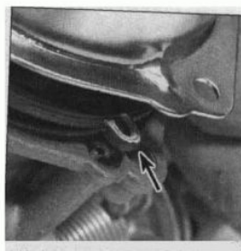
9.11 Ensure diaphragm tab, vacuum tube and cover protrusion align
