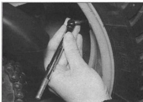
7.4 Measuring tire air pressure
