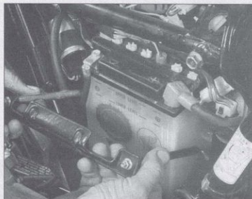
3.2 Battery clamp is held by two nuts on 700/750 Sabres
