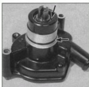
9.14 Check the water pump seal for damage and replace the O-ring whenever the pump is removed (arrows)
