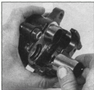
3.16 Ensure that the pistons are inserted squarely into their bores
