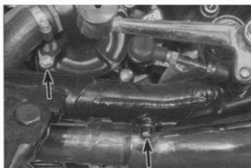
8.5 Coolant drain plug in frame section (right arrow), and water pump drain plug (left arrow)
