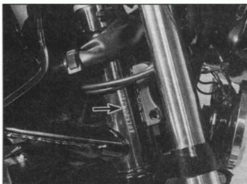
Frame number location on steering head right side
