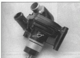
8.2 Water pump drainage hole (arrow)
