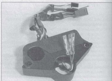
19.15 Position wire harness as shown when installing odometer assembly
