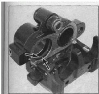
3.14 Piston seal (upper arrow) and dust seal (lower arrow) locations in caliper bore
