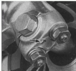
15.14 Arrow mark must face forward on 700/750 Sabre axle clamp
