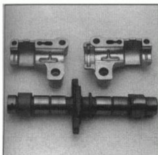
9.15 Check the cam bearing surfaces and camshaft for wear or damage
