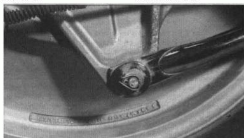
16.4 Brake torque arm is retained to brake panel by split pin, nut and pivot bolt on 1985-on models
