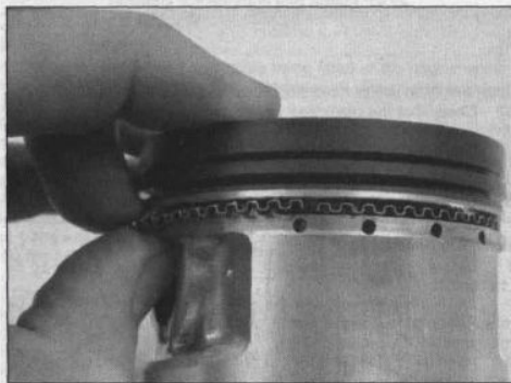
30.9b Make sure the oil control expander ends don't overlap
