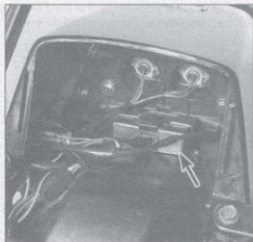
16.2 Tail/stop light sensor (arrow) is located on rear fender (750 Sabre shown)
