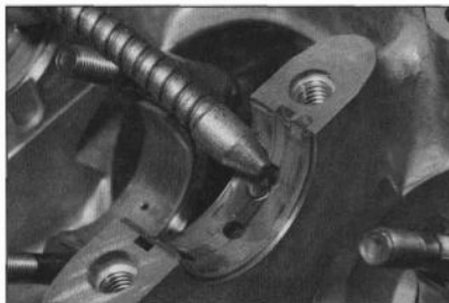
28.27 Oil insert liberally before crankshaft is installed
