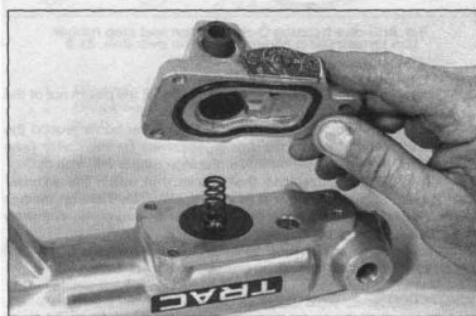
9.4 Remove the four socket-head screws to free housing from slider
