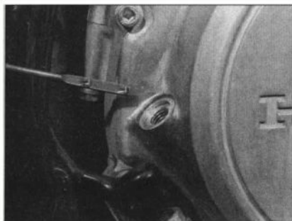
3.7 Oil level should lie between dipstick marks (all except 1882 750 models)
