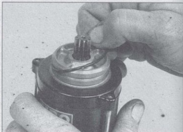
33.5 Install a new O-ring on the starter body
