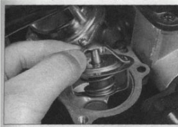
6.7 Lift the thermostat out of its housing
