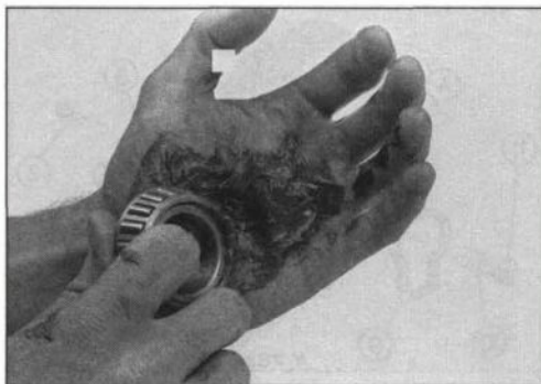
10.57 Work grease fully into the rollers or balls
