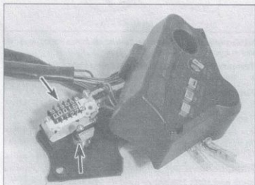
19.13 Release bottom cover to access odometer and bulb (arrows)
