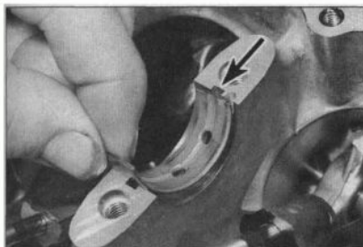
28.26 Ensure locating tab engages cutout (arrow) when installing main bearing inserts
