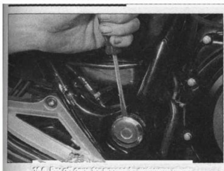
16.6 Pry off caps for access to swingarm pivots
