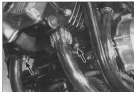
8.6 Front cylinder bank drain plugs (arrows)
