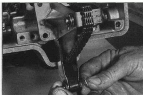
8.2a Camchain and tensioner assembly
