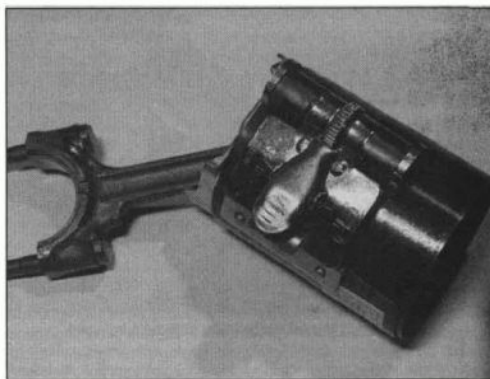
29.47 Piston ring compressor installed
