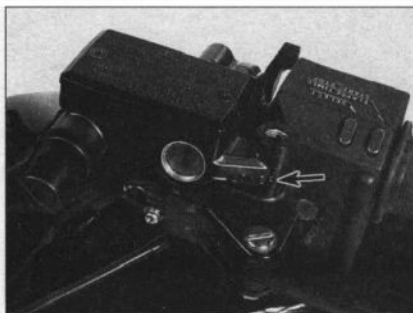
3.12 Brake/clutch fluid level must be above LOWER mark on master cylinder
