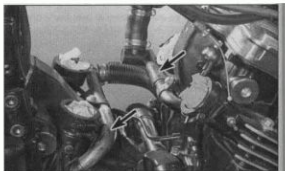
9.13 Coolant crossover pipe locations
