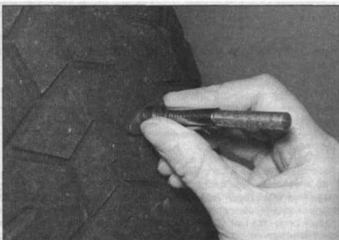
7.2 Measuring tire tread depth
