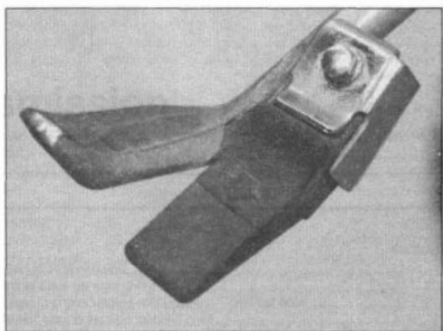
28.2 Side stand rubber wear limit is indicated by arrow
