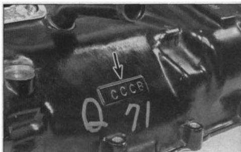
28.11 Main bearing bore diameter codes are stamped in upper crankcase half (arrow)
