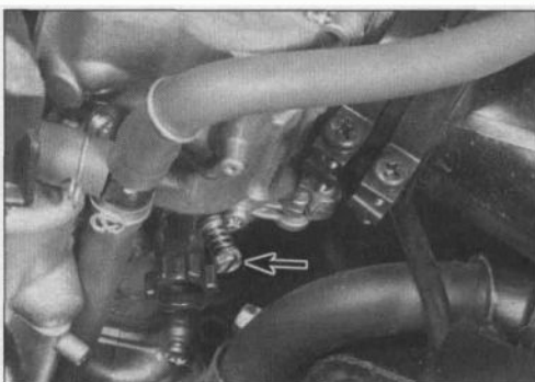
18.12 Synchronization screw for No 3 carburetor (arrow)
