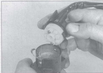
22.7b Release the wire clamp tabs and remove switch
