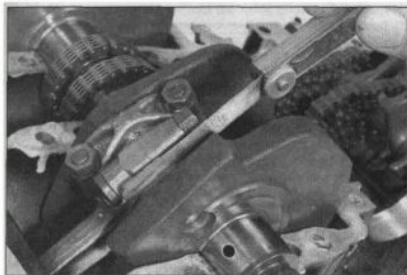
29.1 Measuring connecting rod side clearance
