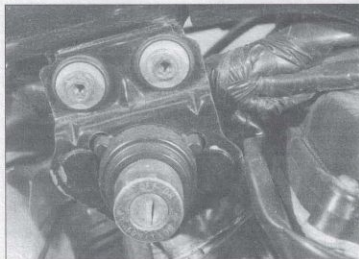
22.14 Switch is retained to frame top tube by two socket head bolts on 1987 and 1988 700/750 Magnas
