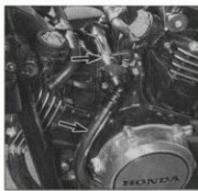
9.7 Coolant inlet and connecting pipe locations
