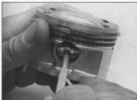
29.20b ... or check by direct measurement
