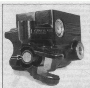
5.10 Master cylinder piston and dust boot location
