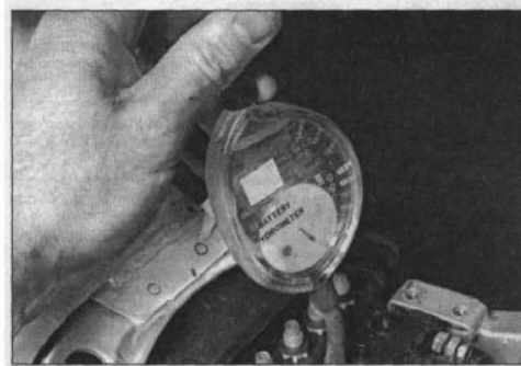
4.6 Measuring electrolyte specific gravity with a hydrometer
