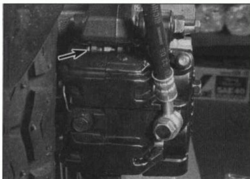
5.1 Brake pad wear can be checked through inspection window in caliper body (arrow)
