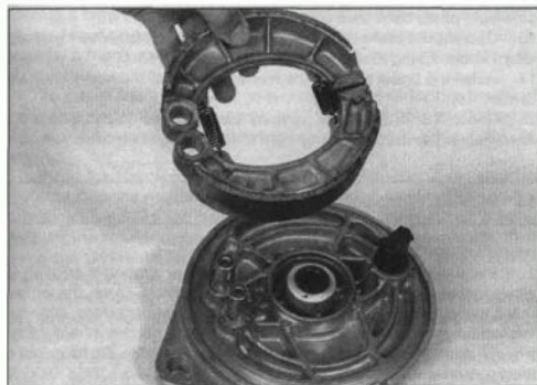
12.4 Remove the brake shoes and springs as a single unit
