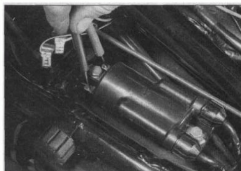
3.5 Measure the coil's primary resistance between the low tension terminals
