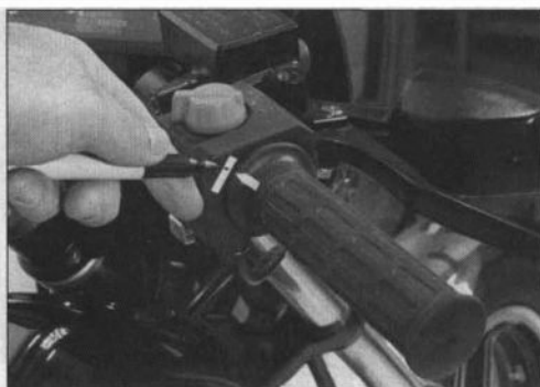
8.3a With the throttle at rest, mark the relationship of the grip to the right switch assembly...
