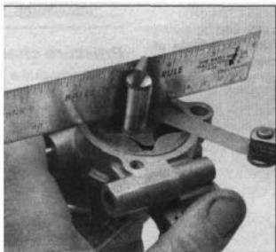
21.26c Use a straightedge and feeler blades to measure rotor end clearance
