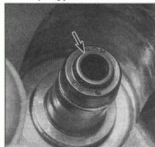
12.27 Install new valve stem seals (arrow) on the guides
