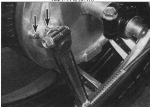
5.4 Drum brake linings are worn when indicator pointer and index mark align
