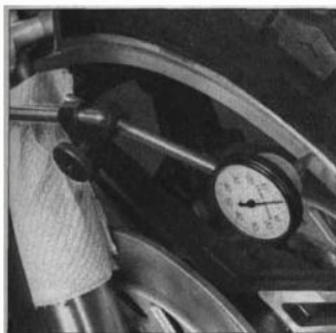
13.2b Measuring axial runout
