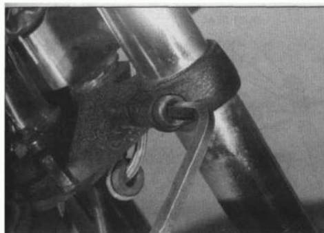
7.8 Loosen fork pinch bolts on upper and lower triple clamps to release forks
