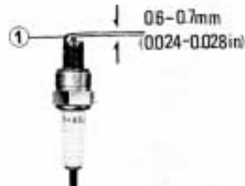
① Bend side electrode to adjust gap
