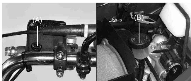
(A) and (B). Front and rear brake fluid reservoirs.
