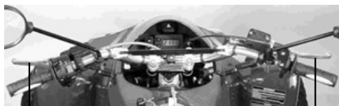
(1). Clutch lever (2). Front brake lever.
