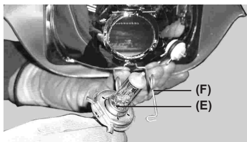
(F) Wire spring bulb attachment.
