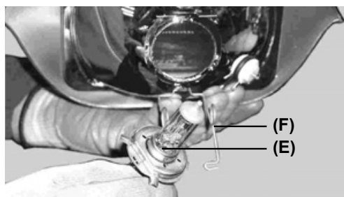
(F). Wire spring bulb attachment.
