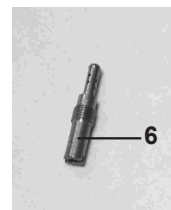
5 - Chain and swing arm adjustment tool. 6 - Idle jet.
