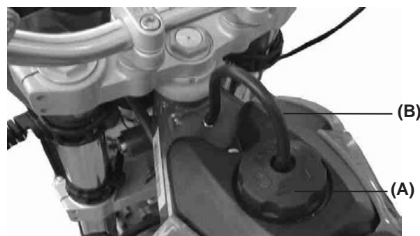
(A). Fuel cap. (B). Fuel vent hose.
