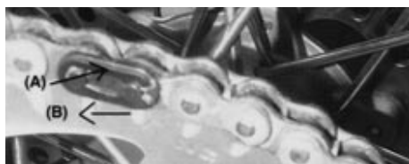
(A). Clip. (B). Direction of Chain Rotation.
