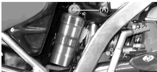
(A). Compression dampening adjuster
