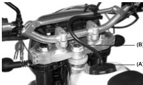
(A). Fuel Cap. (B). Fuel Vent hose.
