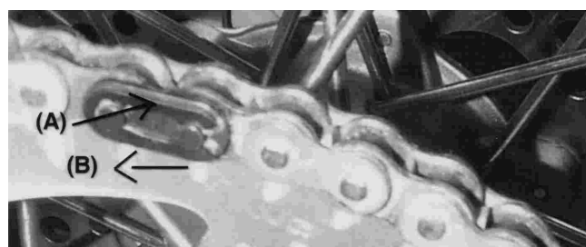
(A). Clip. (B). Direction of Chain Rotation.
