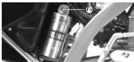
(A). Compression dampening adjuster
