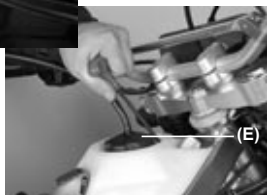
6. Unscrew screw of fuel tank (E).
