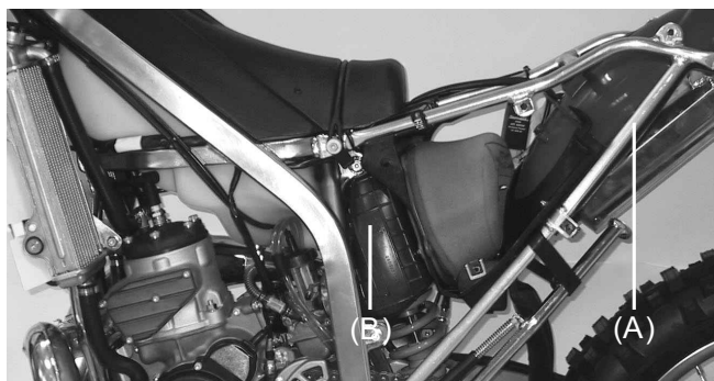
(A). Rear subframe. (B). Air cleaner box.
