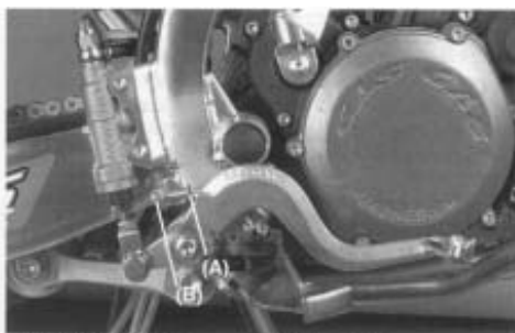
(A). Adjusting Bolt (B). Locknut
