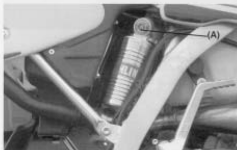
(A). Compression dampening adjuster.
