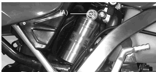
(A). Compression dampening adjuster
