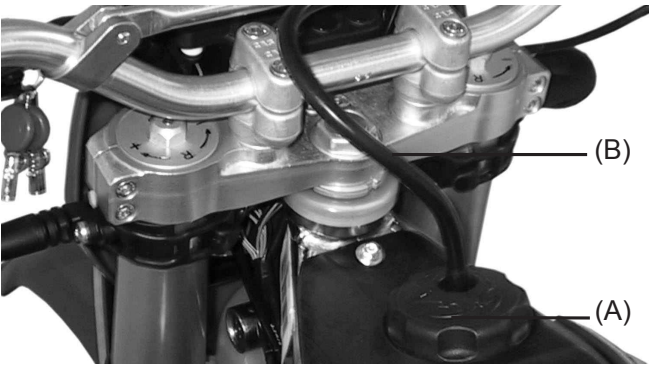
(A). Fuel Cap. (B). Fuel Vent hose.
