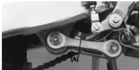
(A). Rebound dampening adjuster
