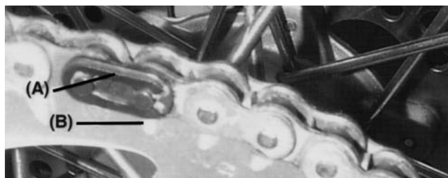
(A). Clip. (B). Chain direction of rotation.
