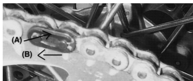
(A). Clip. (B). Direction of Chain Rotation.
