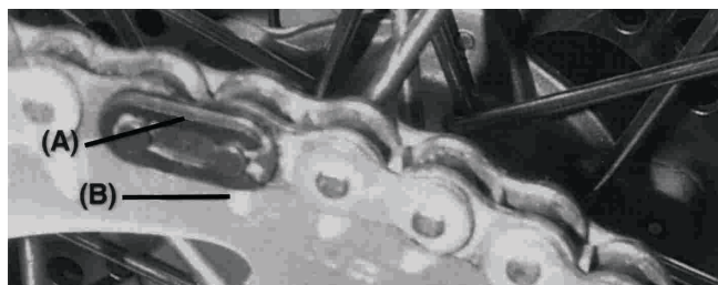
(A). Clip. (B). Chain direction of rotation.
