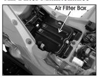
To maintain the highest performance from your engine and to reduce excessive wear that could cause engine failure the engine requires a continuous flow of clean air. Air is taken into the engine through an air filter to clean the air prior to mixing it with fuel in the carburetor.
