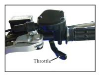
The travel of the throttle lever is controlled by the throttle stop bolt.
