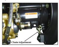
The chain should be kept well lubricated to prevent excess wear and premature failure. We recommend that you lubricate the chain every 15 hours of operation, or more frequently if needed, with a high quality chain lubricant.
