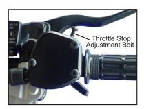
and turn the throttle stop screw clockwise to reduce the throttle travel thus reducing the maximum speed of the unit. Turning the stop screw counter clockwise will increase the throttle travel thus increasing the maximum speed of the unit. Tighten the stop screw locking nut when the desired throttle travel has been established.
