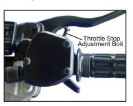
To increase the throttle's travel, thus increasing the maximum speed, turn the throttle stop bolt counter clockwise. To decrease the throttle's travel, thus decreasing the maximum speed, turn the throttle stop bolt clockwise.
