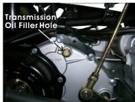
1. Place an oil catch pan under the unit directly below the transmission box.
