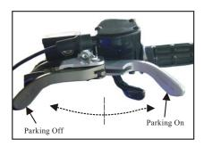
The parking brake is shown on the picture. The position of parking Off is on the left side. Turn parking brake to right side is parking On.
