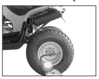
It is important to inspect your tires and wheels for damage and wear before each riding session. Inspect each tire for cuts, tears and punctures. Inspect the wheel rim for dents and separation of the wheel from the tire bead.
