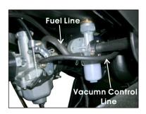
When the fuel valve set on the "PRI" Position, the unit is not equipped with a vacuum controlled fuel valve. The fuel will flow to the carburetor directly.
