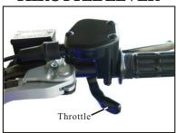
The throttle lever is located beside the righthandlebar grip and is operated by using the righthand thumb. The lever is spring loaded and will return to the idle position when you remove your thumb from the lever. To accelerate the unit, simply press the lever forward to open the throttle slide in the carburetor. To slow the unit, reduce the pressure on the lever or remove your thumb and the throttle will return to the idle position automatically.
