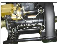
Loosen the axle position lock bolt slightly and turn the chain adjuster nut to take up the excess slack in the chain. Once the chain has been adjusted to the proper tension retighten the axle position locking bolt.
