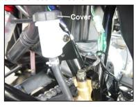
Fill the reservoir to 1/8" from top with Dot-3 SAE-J 1703 grade brake fluid.
