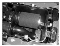
Wash the element in a non-flammable solvent such as air-filter cleaner from your local auto parts dealer.
