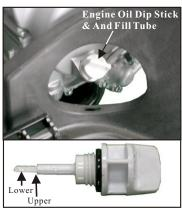
Your ATV uses automotive type engine oil to lubricate the engine. The engine oil dip stick is located on the right hand side of your engine below the transmission shifting lever.
