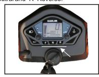
The instrument panel has three lights that correspond to the transmission shifter shaft position.
