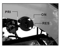
Place the valve in the "ON" for normal operation of the unit. This allows fuel to flow to the carburetor for normal operating. The "RES" position allows fuel to flow from the small reserve in the tank to allow the unit to be taken to a refueling location. When you have to switch to the "RES" position you must refuel the unit as soon as possible.
