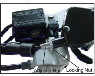
The cable should be adjusted to allow for  $\frac{1}{8}$ " free travel before the throttle engages the carburetor throttle slide. Slide the adjuster cover down the cable to uncover the adjuster assembly. To adjust the cable's free travel, loosen the locking nut of the cable adjuster, and turn the adjuster nut until there is \( \frac{1}{8} \)" free travel in the lever. Tighten the locking nut to secure the adjusting nut. Slide the cover back over the adjuster assembly.
