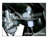
The filter should be replaced every 600 hours of operation and at the start of each season.
