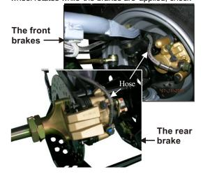
your fluid level and brake pads. If the brake lever feels spongy or does not stop when squeezed, you may have air in the lines. All air must be purged from the brake lines for the disc brake to operate properly. (See purging brake lines).
