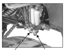
• Rear brake cable • Front brake cable
