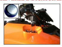
Your ATV is equipped with a fully automatic C.V.T. transmission and has forward and reverse gearing. Atransmission shifting shaft is located on the right hand side of your vehicle. The shifter has three positions "F" Forward, "N" Neutral and "R" Reverse.
