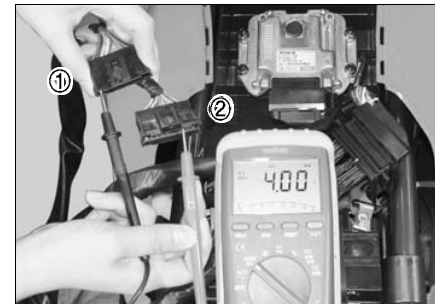
Connecting the wire harness for checking
