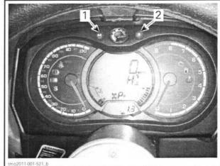
M (mode) button 2 S (set) button (pressed repeatedly to toggle secondary display)
