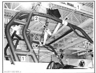
Lifting strap around horizontal side tubes (top)
