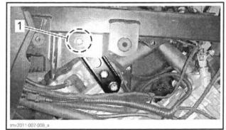
Rubber isolator is located between frame and engine support
