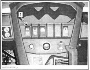
Low/High beam headlight switch to toggle quickly
