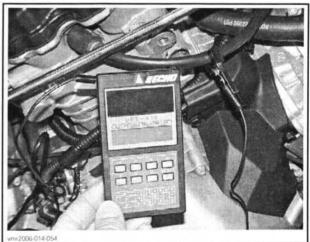
VERIFYING ENGINE RPM USING A DIGITAL INDUCTION TACHOMETER
