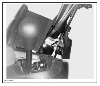
Remove ignition switch and choke lever.
