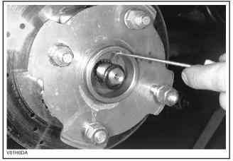
CHECK THE O-RING FOR DAMAGE, REPLACE IF NECESSARY
