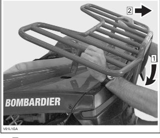
Step 1: Pivot botton of rear rack toward inside Step 2: Pull rear rack toward back
