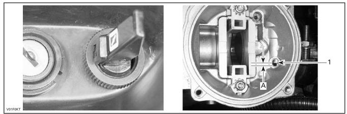
HALFWAY POSITION 1. Plunger end must be here A. Opening to specification value
