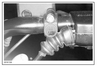
Connect brake hose to master cylinder with bolt and new sealing washers.
