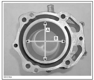
Perpendicular to crankshaft axis Α.
