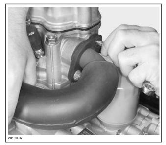
Remove screw from exhaust pipe bracket **no. 16**. Remove springs **no. 17** retaining exhaust pipe and muffler **no. 18**.
