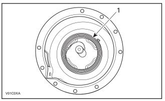
TYPICAL 1. Grease inside spring guide
