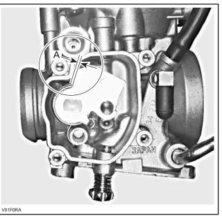
*THROTTLE LEVER AT THE FULL POSITION A. 1 mm (1/32 in)* Retorgue lock nut.
