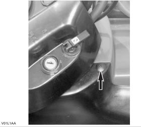
Remove screw on the LH side and separate from dart on the RH side.
