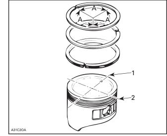
1. DO NOT align ring gap with piston trust side axis
