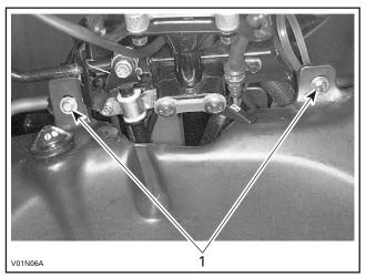
1. Remove both top fuel tank screws
