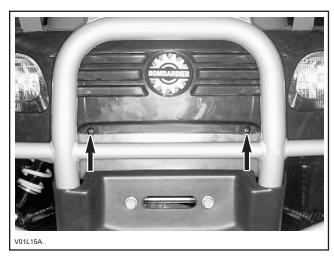
Remove the screws no. 38 on the top of facia.
