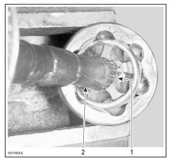
1. Circlip 2. Shaft
