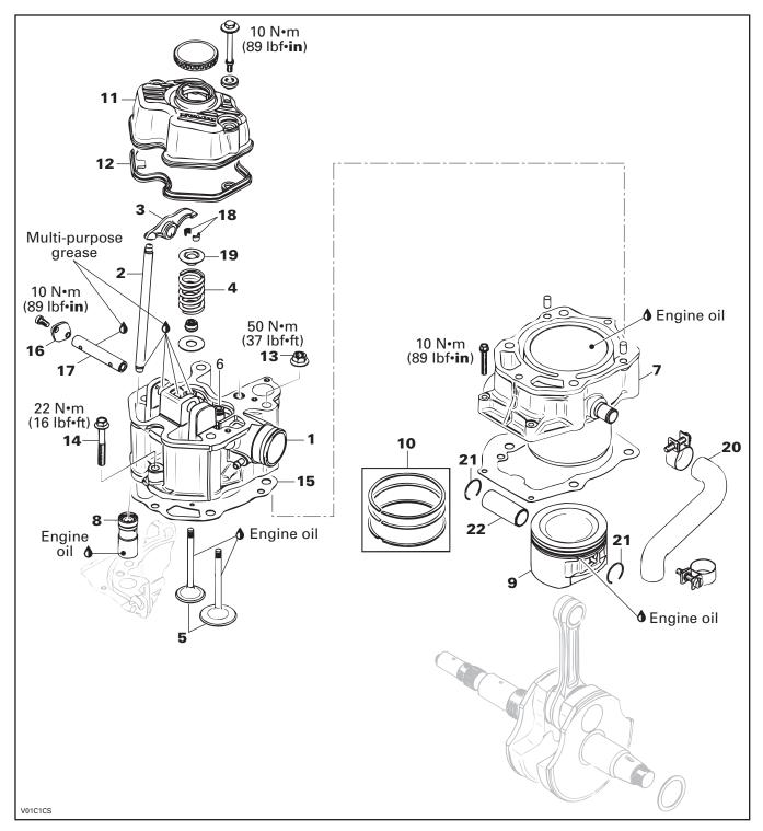
**NOTE:** For cylinder head, cylinder and piston removal, it is not necessary to remove engine from vehicle.
