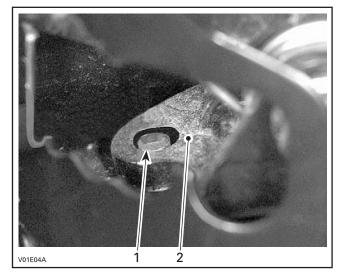
Interlock pin end 1. 2. Sifter lever plate
