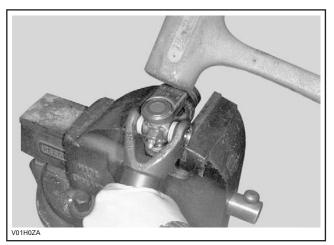
Support U-joint in vice and drive inner yoke down to remove remaining bearing caps.
