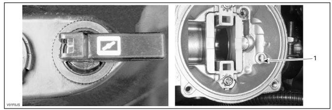
**FULLY CLOSED POSITION** 1. Plunger end must be here
