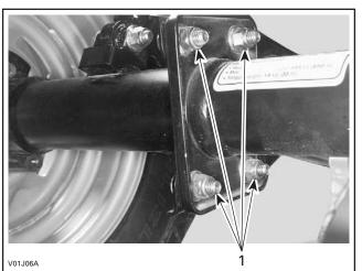
1. Remove flanged bolts and elastic flanged nuts
