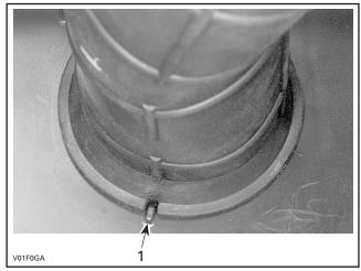
AIR BOX SIDE — RUBBER FLANGE INSTALLATION 1. Notch aligned with recess
