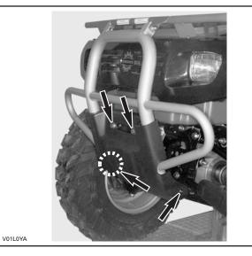
**7, Front Bumper** Remove front skid plate. Remove bolts **no. 29** and **no. 30**.
