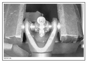
Using a suitable arbor, fully seat bearing cap in one side. Continually, check for free movement of bearing cross as bearing caps are assembled.
