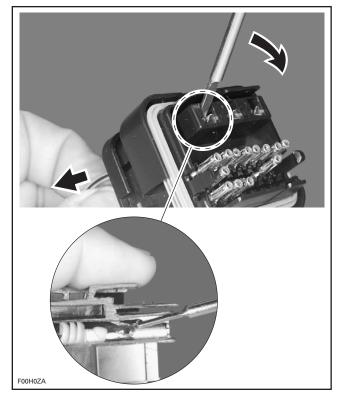
Pry back the retaining tab while gently pulling wire back until contact is removed.
