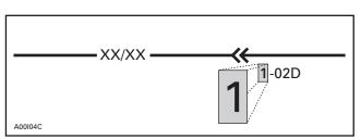
THE SHADED PART INDICATES THE CONNECTOR HOUSING AREA
