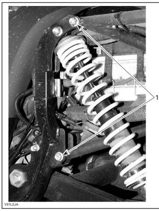
1. Remove the M10 x 55 mounting flanged bolts
