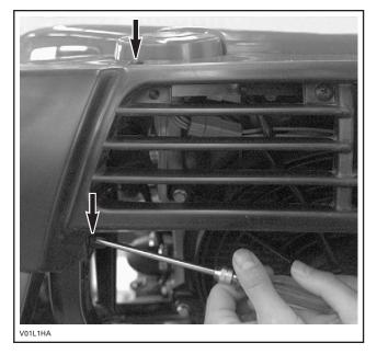
Remove plastic pin of rear fender. Remove screws **no. 33** and **no. 34**.
