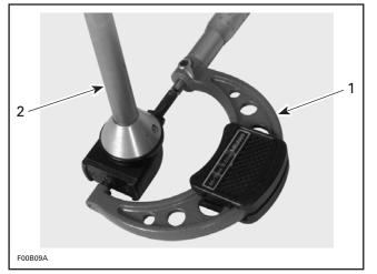
Use the micrometer to set the cylinder bore gauge
