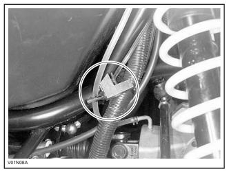
HOSE PINCHER INSTALLED ON FUEL TANK VENT LINE
