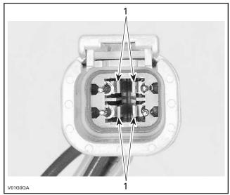
FEMALE CONNECTOR HOUSING 1. Retaining tab
