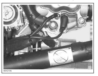
Before to start the engine, remove spark plugs and ground them on engine or frame. Start vehicle about thirty seconds. This operation activated the oil pump. Reinstall spark plug and check if vehicle run correctly.
