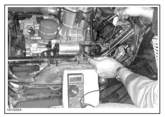
**NOTE:** If the voltage regulator/rectifier is within the specification, the wiring harness between the voltage regulator/rectifier and battery is defective. If the voltage regulator/rectifier is out of specification and the stator test good, the voltage regulator/ rectifier is defective.
