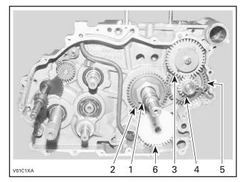
1. Crankshaft gear nut
