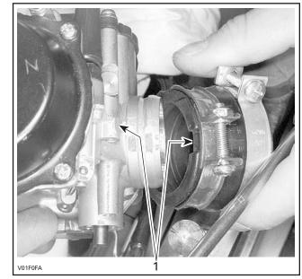
CARBURETOR SIDE — RUBBER FLANGE INSTALLATION 1. Flange recess aligned with carburetor notch
