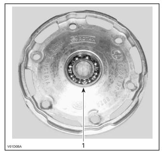
1. Retaining plate bearing
