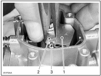
Release tension on throttle lever
