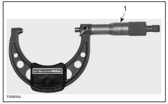
1. Micrometer set to the piston dimension
