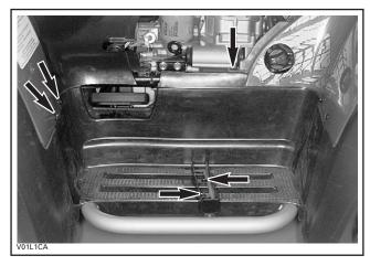
On front and rear mudguards, remove the three first screws **no. 35** and screws **no. 34** retaining side panel with mudguards.
