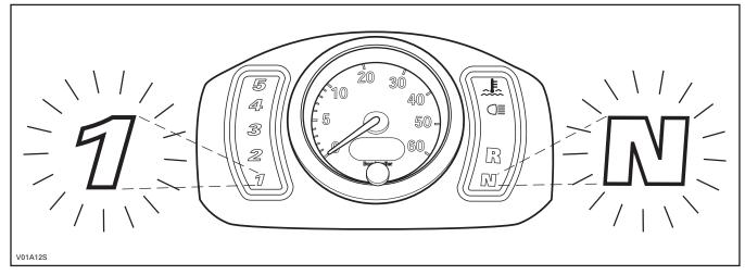
To set the MPEM into the diagnostic/calibration mode, the following sequence needs to be done: – Place a diagnostic jumper in the diagnostic connector.
