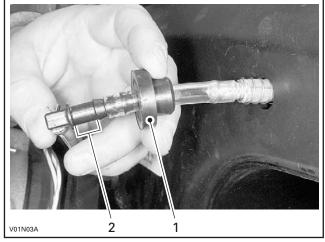
Grommet properly position for tank insertion
