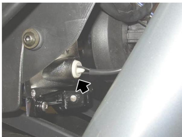
LOW BEAM/HIGH BEAM BULB (2)
