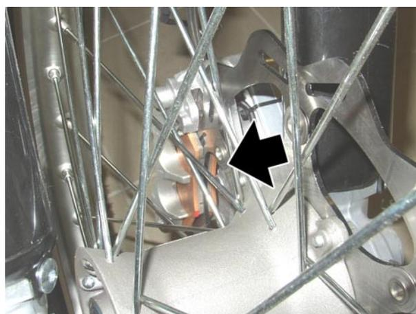
**Checking the rear brake calliper pads:**
