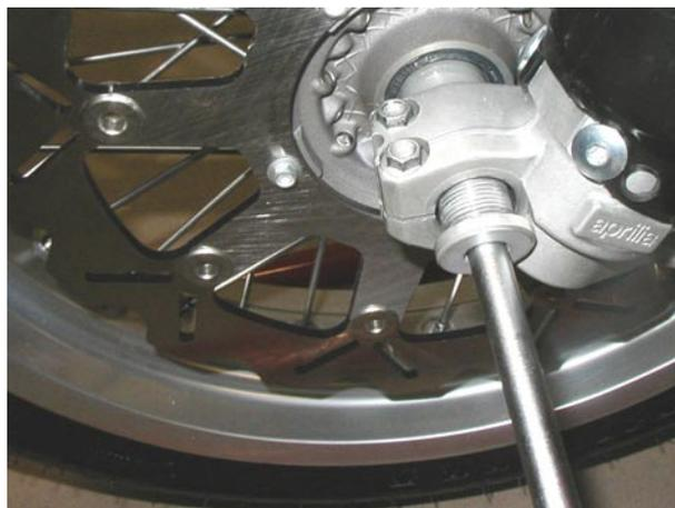
**NOTE** To lock wheel shaft rotation tighten the two screws on fork clamp, right side.
