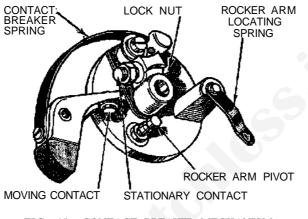
FIG. 45.—CONTACT BREAKER MECHANISM.
