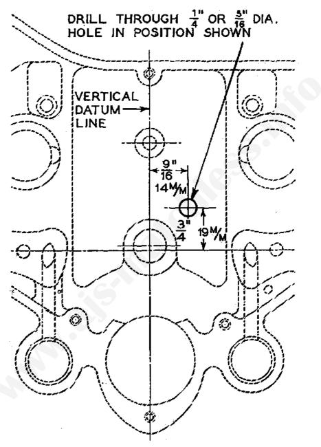
FIG. 9.—ADDITIONAL OIL DRAIN HOLE IN THE TIMING CHEST. This modification has the effect of lowering the level of oil in the sump when the machine is stationary.
