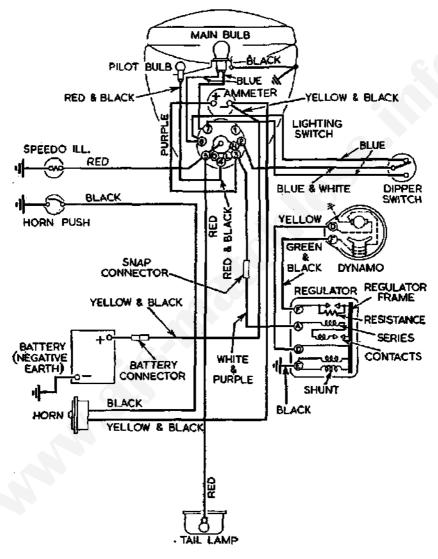
FIG. 48.-WIRING DIAGRAM FOR 1950 MODELS.
