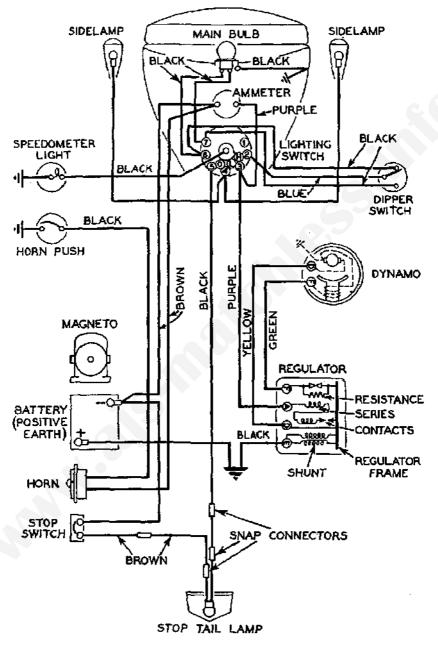
FIG. 50.-WIRING DIAGRAM FOR 1954 MODELS.
