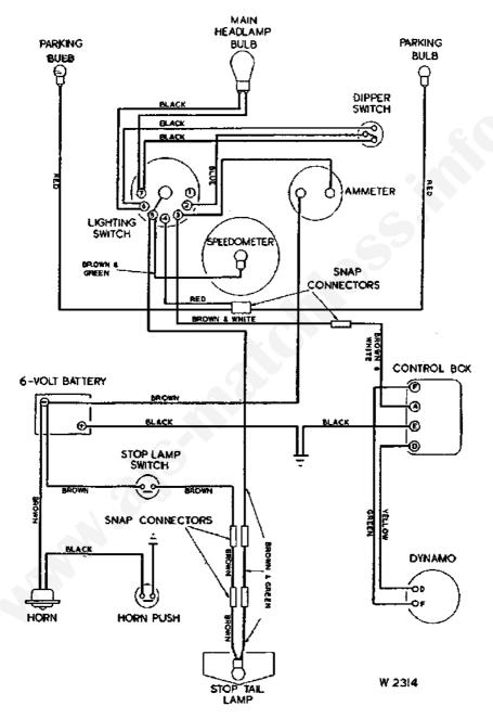
FIG. 51.—WIRING DIAGRAM FOR 1955 MODELS.
