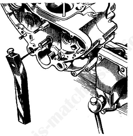
FIG. 14.—AN EASILY-MADE TOOL FOR EXTRACTING THE INTERMEDIATE TIMING GEAR SHAFT.
