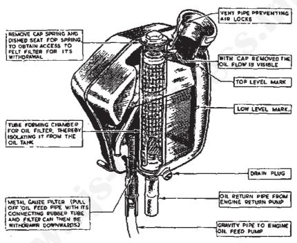
FIG. 3.—CUTAWAY VIEW OF THE OIL TANK FITTED **FORE**-1955 MODELS.
