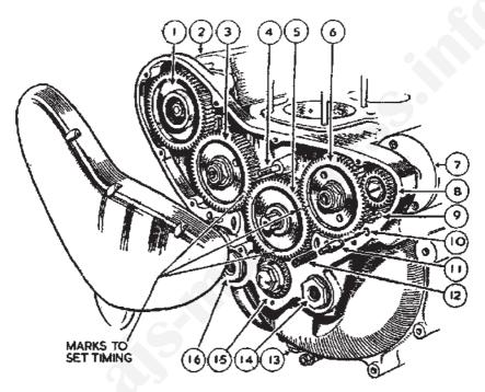
FIG. 1.-TIMING GEARS, SHOWING THE TIMING MARKS.
