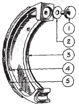
FIG. 42.—BRAKE SHOE AND THRUST PIN WITH PACKING WASHER.
