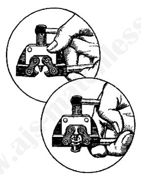
FIG. 21.—METHOD OF USING THE RIVET EXTRACTOR.
