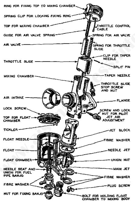
FIG. 18.—EXPLODED VIEW OF AMAL TYPE 76 CARBURETTER.
