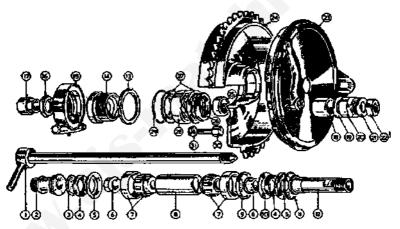
FIG. 39.—EXPLODED VIEW OF THE REAR WHEEL BEARING AND BRAKE DRUM FITTED TO 1955 MODELS.
