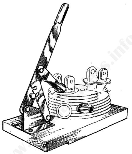
FIG. 11.—VALVE SWUNG COMPRESSOR. This tool is recommended where the utilisation justifies the expense.
