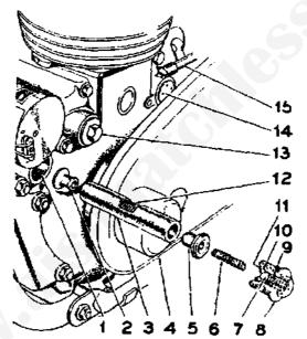
FIG. 6.—EXPLODED VIEW OF FELT OIL FILTER IN DRIVING SIDE CRANKCASE.
