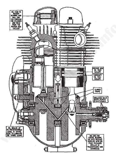
FIG. 8.—CROSS-SECTION OF ENGINE SHOWING OIL GALLERIES, OIL PASSAGES AND RELEASE VALVE.
