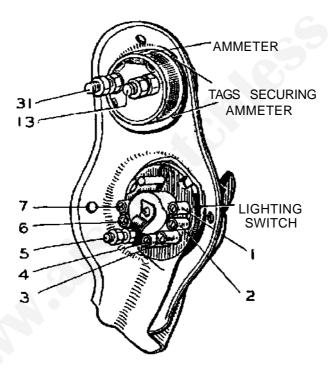
FIG. 47.-AMMETER AND SWITCH PANEL ON HEADLAMP.
