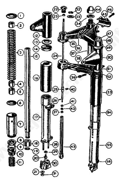
FIG. 32.—EXPLODED VIEW OF FRONT FORKS FITTED TO 1953<sup>-54</sup> MODELS.
