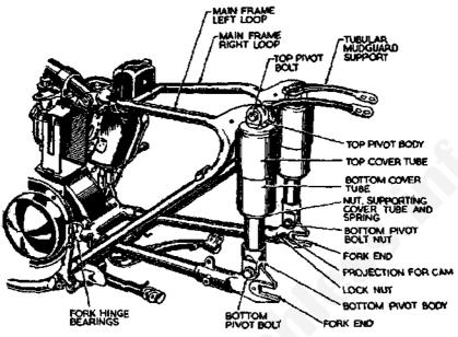
FIG. 36.—THE REAR SUSPENSION.
