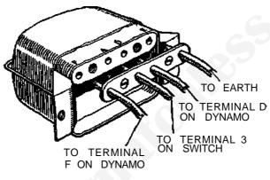
Fig. 46.—REGULATOR CONNECTIONS.
