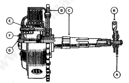
FIG. 22.—SECTION THROUGH CLUTCH FITTED TO B.52 GEARBOX.
