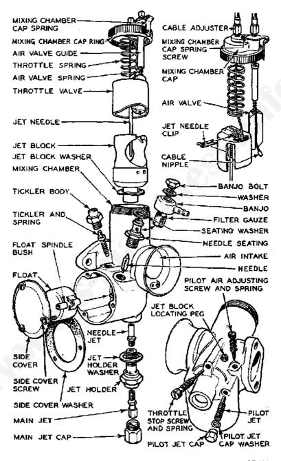
FIG. 19.—EXPLODED VIEW OF AMAL MONOBLOC TYPE 376/6 CARBURETTER.
