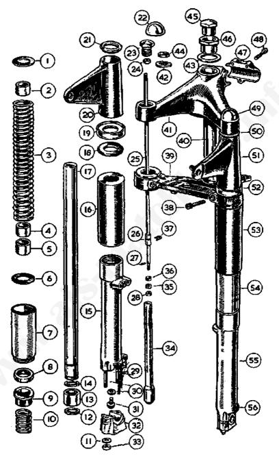
FIG. 33.-EXPLODED VIEW OF FRONT FORKS FITTED TO 1955 MODELS.
