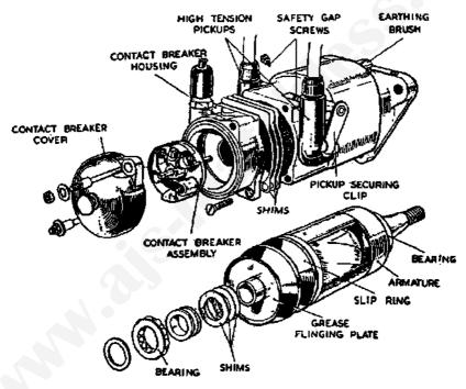
FIG. 44.-EXPLODED VIEW OF THE LUCAS K2F MAGNETO.
