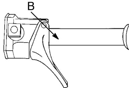
The throttle safety switch is designed to stop the engine whenever all pressure is removed from the throttle lever and the throttle cable or valves do not return to the normal closed position.
