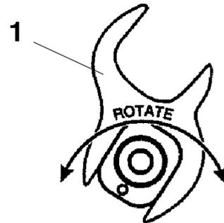
To decrease weight transfer under acceleration (for improved cornering), rotate the RRSS to a higher position.
