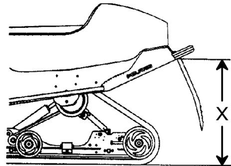
Take the first measurement with no rider and with the rear suspension at full extension. **NOTE:** The rear bumper may need to be lifted upward slightly to fully extend the rear suspension.
