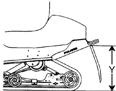
To determine sag, commonly referred to as ride-in, subtract measurement Y from X ( $\text{Sag} = X - Y$ ). Adjust sag by rotating the torsion spring preload cams located on the rear torque arm. Use the illustration or the decal found under the hood for reference. The ideal amount of Sag for the PRO X rear suspension is five inches ( $X - Y = 5$ ).
