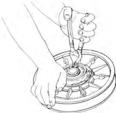
Check sliding half bushing wear, replace bushing if wear is excessive.
