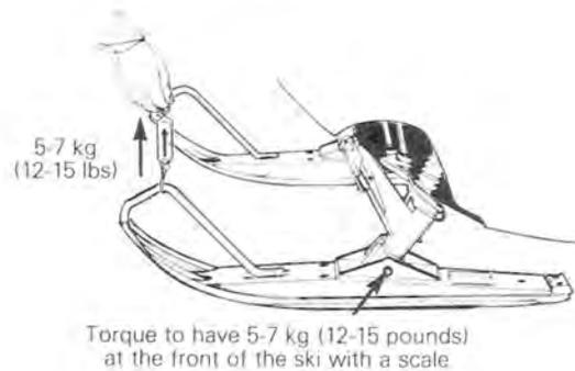
③⑤ Torque the elastic stop nut on the ski leg coupler to 56-57 N•m (42-50 ft-lbs).
