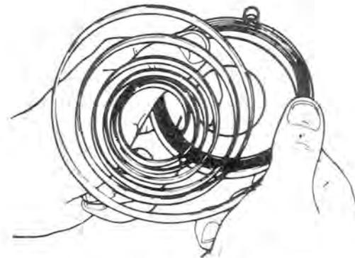
Position spring assembly into starter housing as illustrated, then place rope sheave into starter housing making sure that the sheave hub notch engages in the spring hook.
