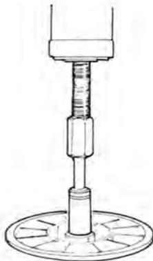
Install new bushing using same procedure.
