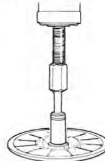
Install new bushing using same procedure.
