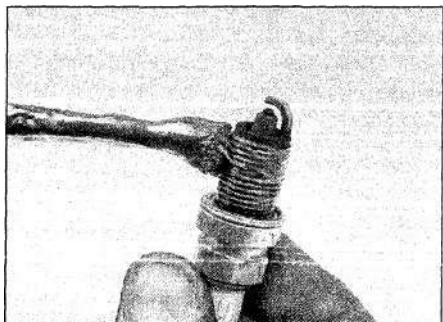
22.16a Apply a thin coat of anti-seize compound to the spark plug threads
