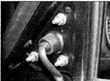
20.3 Undo the three mounting nuts and remove the mirror assembly
