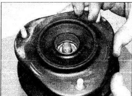
3.5a Lift off the upper mounting/bearing ...
