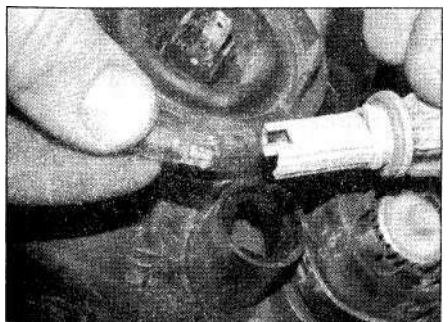
7.13 Pull the sidelight wedge bulb from the holder
