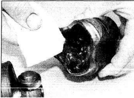
3.11 c Apply the supplied grease to the joint housing
