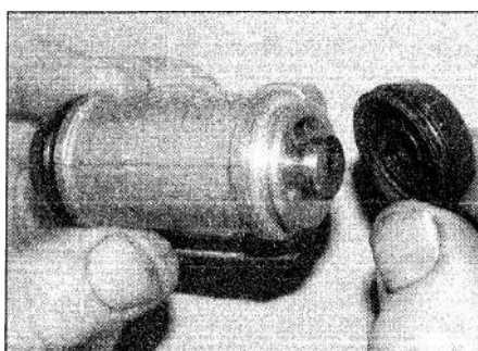
12.6 Pull the rubber dust seals from the cylinder
