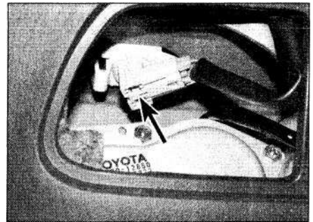
7.80 Rotate the bulbholder (arrowed) anti-clockwise
