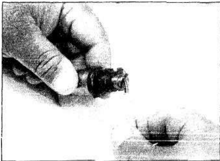
12.44a Remove the O-ring from the injector
