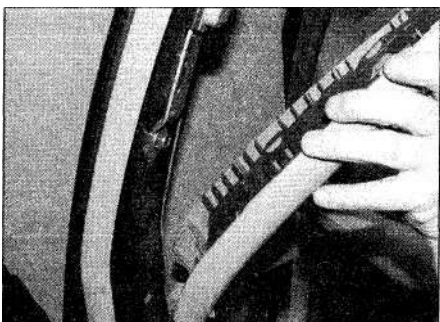
27.12 Pull the top of the B-pillar trim towards the centre of the vehicle
