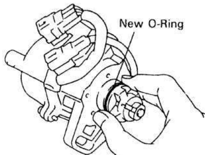
3.8 Fit a new O-ring to the distributor housing
