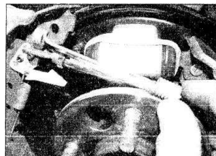
11.7m Fit the adjuster strut and spring to the front brake shoe . . .
