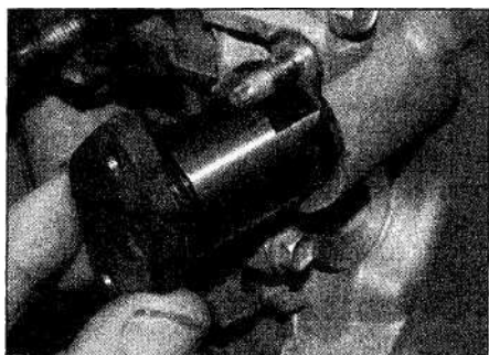
6.11 Undo the two nuts and remove the chain tensioner assembly
