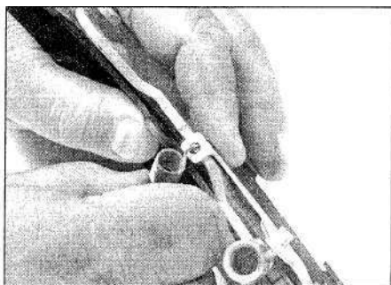
11.5q ... hook the short end of the adjusting lever spring into the shoe lever...
