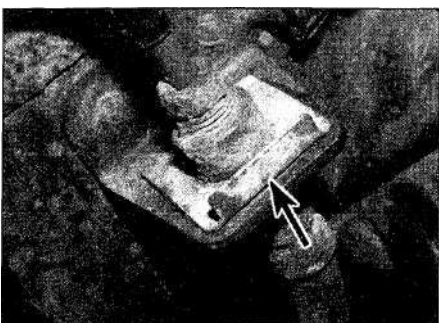
10.3b ... then undo the hose union, and pull out the hose retaining clip (arrowed)
