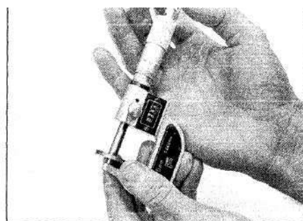
24.8 Measure the shim thickness with a micrometer
