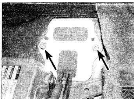
2.7 Undo the two bolts (arrowed) and remove the cable grommet/retaining plate assembly
