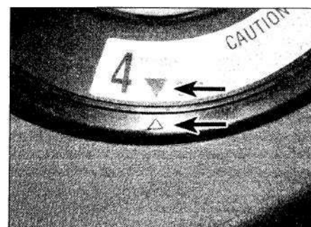
16.7 Align the contact reel pointers (arrowed)
