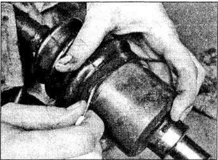
3.13a Equalise the pressure in the gaiter with a screwdriver between the gaiter and the housing
