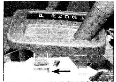
5.3a Release the indicator panel clips (arrowed)
