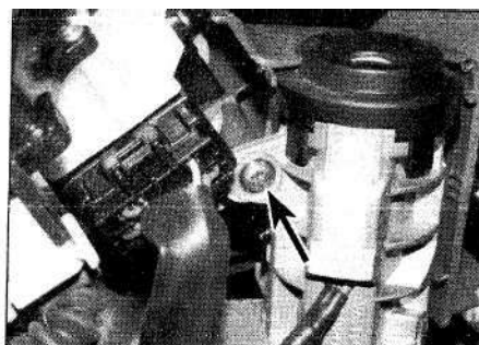
4.4b Upper steering column shroud retaining screw (arrowed)
