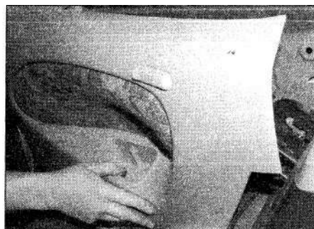
27.17b ... then pull the side panel from place
