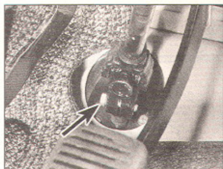
10.10 Steering shaft lower coupling securing bolt (arrowed)
