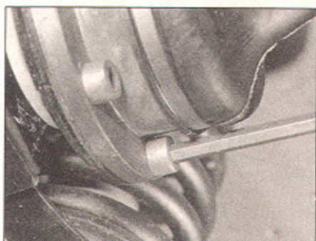
9.5 Tighten driveshaft bolt with suitable key/wrench
