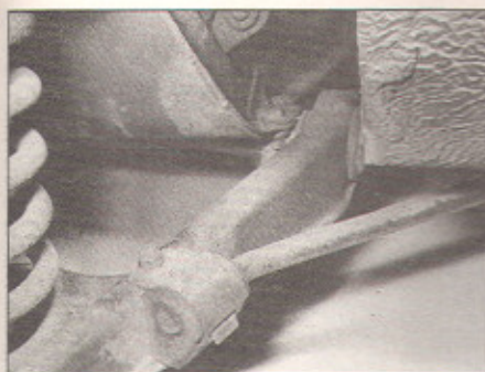
6.1 Anti-roll bar bush and retaining plate on the wishbone arm
