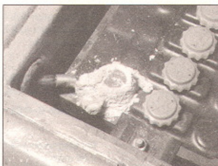
3.2 A badly corroded battery terminal
