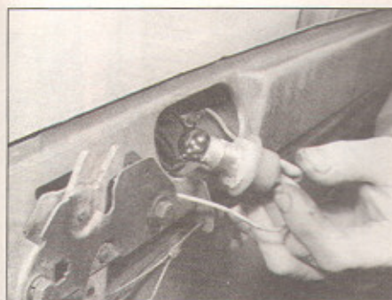
23.1 Rear number plate bulb and holder removed for inspection
