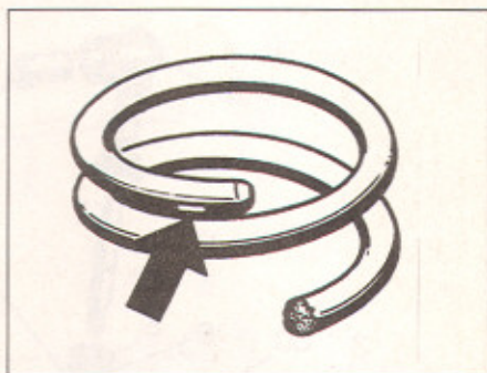
Fig. 8.4 Heavy duty spring is identified by a flat section (arrowed) (Sec 8)
