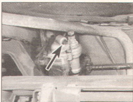
14.4 The steering box in position viewed from underneath. The filler/level plug is arrowed
