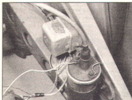
10.1 The coil and voltage regulator location
