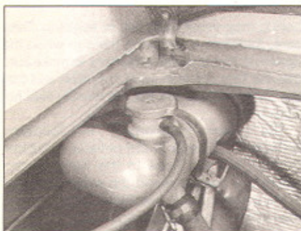
2.4 Remove expansion tank cap
