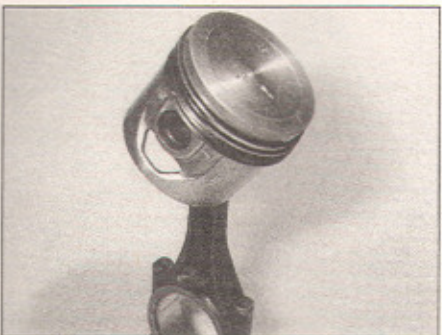
33.4 Arrow on piston crown on opposite side to oil splash hole in connecting rod
