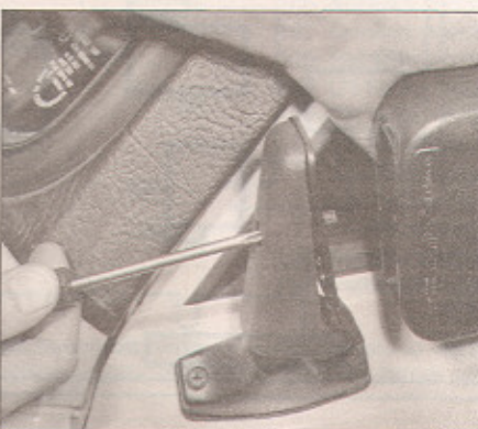
13.31 One screw holds the mirror to the arm
