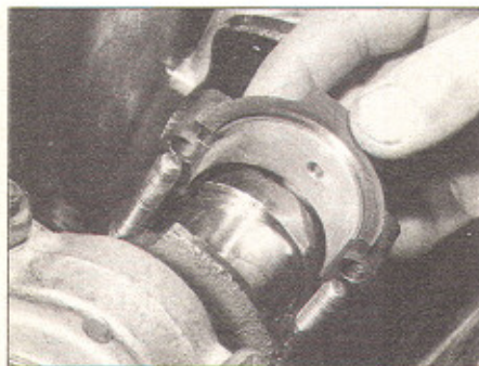
37.5 Refit the bearing end cap
