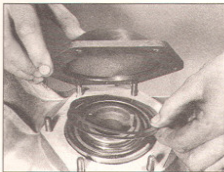
48.1 Fit gasket with breather hole at top and exact number of shims
