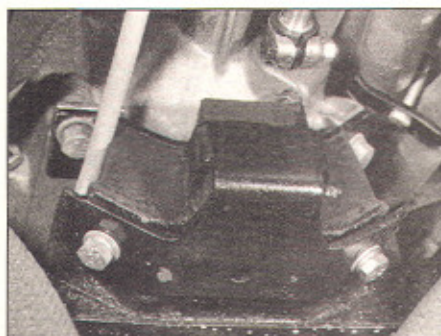
3.15 Gearbox mounting (five-speed)
