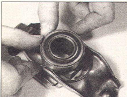
6.4 The release bearing and retaining clip
