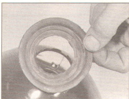
12.8B Remove the seal if necessary
