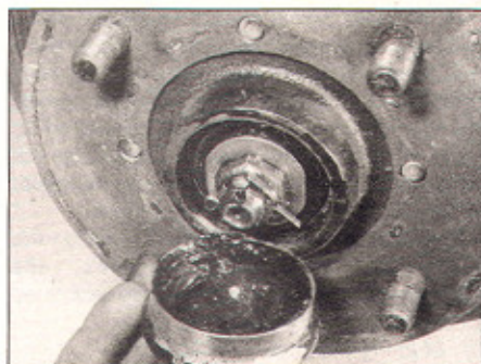
3.3 Grease cap removed to show hub nut and split pin
