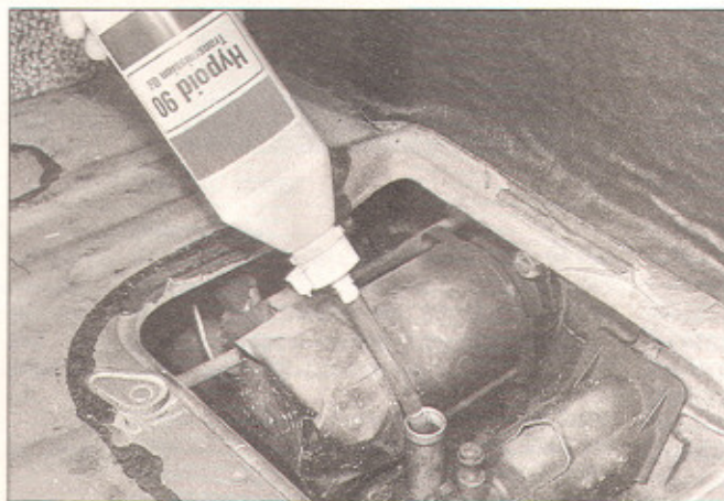
Top up the transmission oil, filling through tube to correct level
