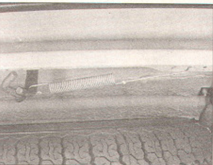
13.3 Spare wheel retaining rod spring
