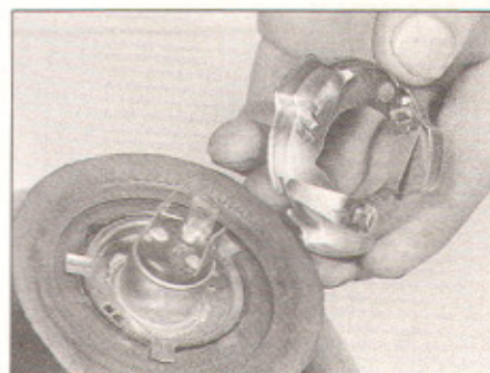
12.7B . . . remove the bulb holder . . .
