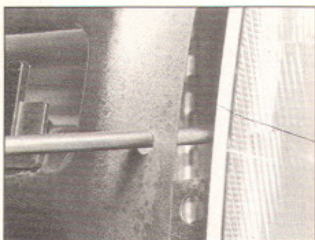
12.4 Horizontal beam adjustment aperture in grille – rectangular headlamps
