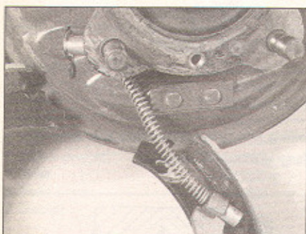
11.9C Handbrake cable attachment to brake shoe
