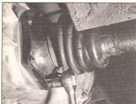
3.9a Unscrew the driveshaft-to-axle housing flange nuts
