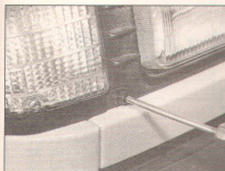
13.5A Radiator grille securing screw removal from outboard edge ...
