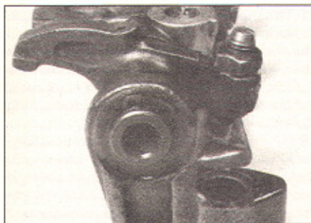
29.1 Remove circlip to dismantle rockers
