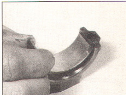
32.2 Locate bearing tongue into groove
