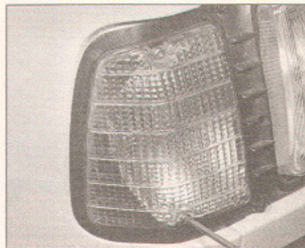
12.17A Undo the indicator lens retaining screws . . .
