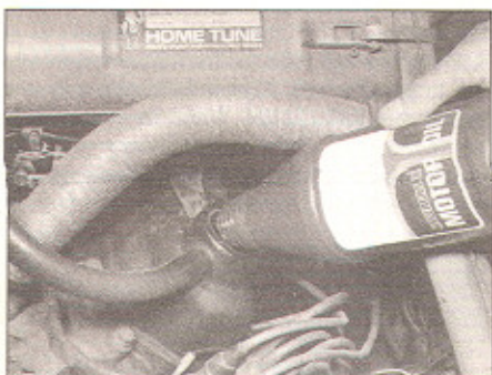
49.19 Refill the engine with oil
