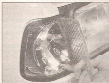
12.17B . . . and remove the lens
