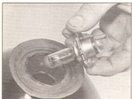
12.8A . . . and withdraw the headlamp bulb
