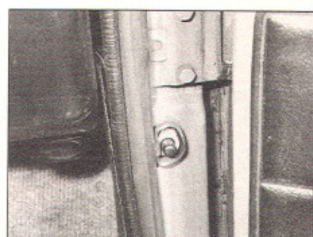
26.8 Door courtesy light switch location in door pillar
