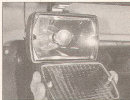
12.23 Rear foglamp lens removed for access to bulb
