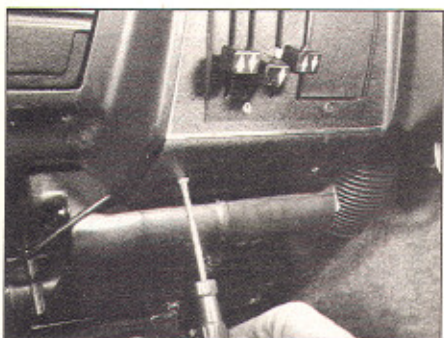
26.4a Remove central panel retaining screws at base ...
