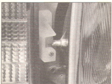
12.9B . . . and nylon holding lugs
