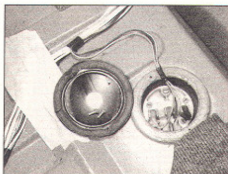
9.5 The fuel tank sender unit with cover removed
