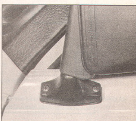
13.32 Two screws secure the mirror arm to the door
