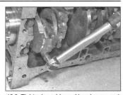
18.9 Tightening a big-end bearing cap nut to the specified torque
