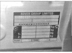
Vehicle identification plate on passenger door pillar
