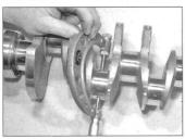
13.6 Measuring the diameter of a crankshaft big-end bearing journal
