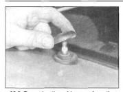
22.2 Removing the rubber cap from the tailgate wiper motor drive spindle
