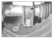
17.13 Steering gear mounting clamp
