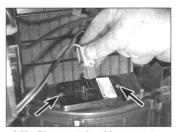
9.28a Disconnect the wiring connector, undo the two screws (arrowed) . . .
