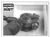
Battery corrosion can be kept to a minimum by applying a layer of petroleum jelly to the clamps and terminals after they are reconnected.
