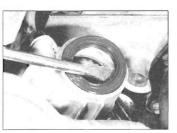
4.4 Levering out a driveshaft oil seal – R65-type transmission
