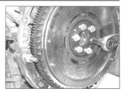
19.8 . . . and tighten to the specified torque
