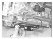
6.18 Removing the clutch release lever shaft – PG1-type transmission
