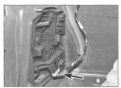
5.28 Disconnecting the wiring connector
