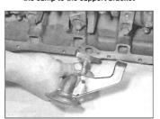
15.10b . . . and remove the oil pump pickup/strainer pipe
