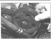
6.9 Removing the power steering pump pulley
