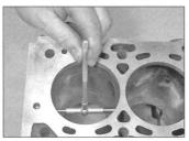
11.15 Measuring a cylinder bore diameter using an internal micrometer
