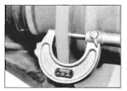
12.3 Using a micrometer to measure brake disc thickness
