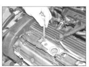
3.4 Remove the two coil bolts . . .
