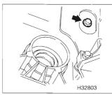
6.23 Prise out the grommet in the cover plate to gain access to the torque converter holts
