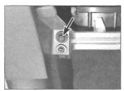
31.20b The facia mounting bolt located in the glovebox aperture
