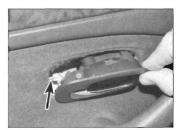
12.4 Slide the door handle forwards, then disconnect the operating rod - arrowed
