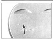
20.6a Arrow of FRONT marking on piston crown must point to timing belt end of engine
