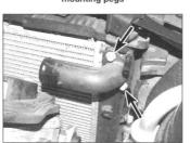
11.10c ... and the radiator coolant elbow
