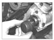
7.21 Remove the exhaust camshaft end caps
