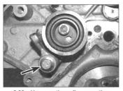
8.22a Unscrew the pulley mounting bolt . . .
