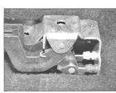
17.4e Lever assembly on the floor bracket
