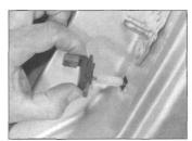
4.19 Removing a courtesy lamp switch
