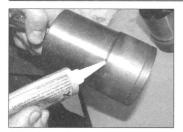
20.14 Apply a bead of sealant around the liner shoulder
