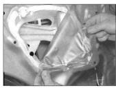
12.18b . . . and carefully peel away the membrane
