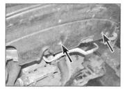
... and inner mounting bolts arrowed
