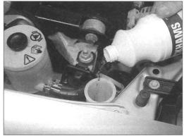
**2** When topping-up the reservoir, a screenwash additive should be added in the quantities recommended on the bottle.
