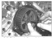
7.19 Fit the camshaft sprocket and new
