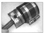
20.10b . . . then slide the piston ring compressor into position
