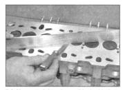
7.6 Use a straight-edge and feeler blade to check the cylinder head for distortion
