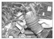
10.3 Removing the inlet air duct
