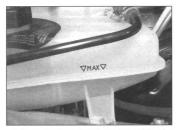
The coolant level varies with the temperature of the engine. When the engine is cold, the coolant level should be on the MAX marking on the side of the reservoir. When the engine is hot, the level may rise slightly.
