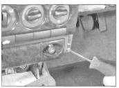
31.6a Undo the outer screws . . .
