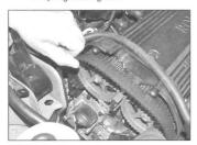
8.5 Fit the timing belt, making sure all the slack is the tensioner side of the belt
