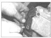
4.4 Unbolt and remove the HT lead guide clip leads from their plugs, and unclip them from
