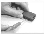
6.1a Using a flat-bladed screwdriver, carefully prise the two halves of the keypad apart . . .
