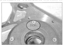
17.3a Some oil pumps have a TOP marking at the top of the cover plate
