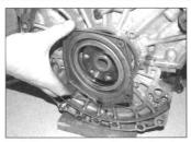
18.7b ... and remove the old oil seal
