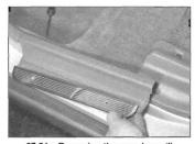
27.24a Removing the rear door sill panel . . .
