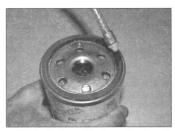
3.12 Apply clean oil to the seal on the oil filter
