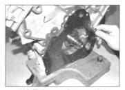
14.9 Fit the new oil pump gasket
