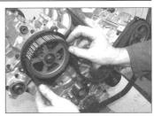
7.20 Fit the timing belt loosely around the sprockets to begin with
