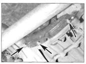
7.12 Undo the bolts (arrowed) from the front cover plate
