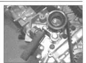
7.28b ... fit and tighten the two bolts ...
