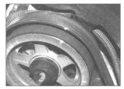
7.39b ... to make marks on the rear inlet sprocket
