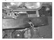
7.16 Undo the two bolts (arrowed) left-hand side shown
