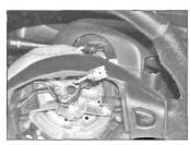
13.8 Withdraw the wiring as the wheel is removed
