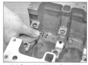
11.1 Removing a piston oil spray jet
