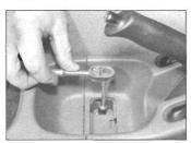
29.3 ... and unscrew the rear console front mounting screws
