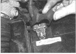
2 Check the tightness of the battery cable clamps to ensure good electrical connections. You should not be able to move them. Also check each cable for cracks and frayed conductors.
