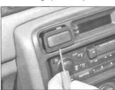
4.7a Using a screwdriver, prise out the hazard switch . . .
