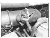
8.20 Disconnect the wiring connector from the MAF sensor – arrowed
