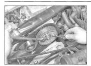
10.8b . . . to hold the sprocket stationary whilst slackening the sprocket adjuster bolts
