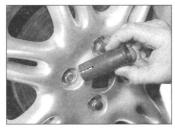
2 On steel wheels, use the end of the wheel brace to lever off the wheel trim. On alloy wheels, remove the locking wheel nut cover with the special tool provided.
