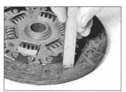
5.7 Using a vernier gauge to check the depth of the lining
