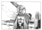
11.7 Removing No 1 cylinder big-end bearing cap and lower bearing shell
