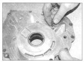
15.2 Remove the pump cover plate screws
