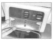
4.42b ... and withdraw the interior light assembly
