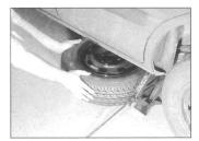
6 Remove the flat wheel and slide it under the sill near the jack; this is a safety measure in case the jack collapses.
