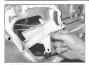
13.15 Removing the rear door lock rod guide and protector
