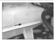
27.17 Coolant expansion tank MAX level
