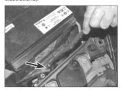
3.4a Unscrew the bolt (arrowed) to remove the retaining clamp . . .
