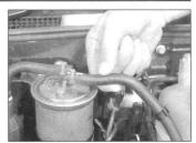
10.5 Check for fuel leaks at the fuel filter unions
