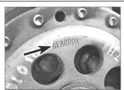
5.12b ... or GEARBOX, which should face the transmission
