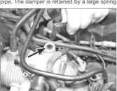
11.21 Release locking collar (arrowed) to disconnect the vacuum hose
