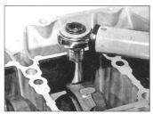
20.8a Tighten the big-end cap bolts to the specified torque setting . . .
