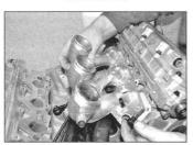
12.31b . . . then refit the rear manifold, and tighten the bolts
