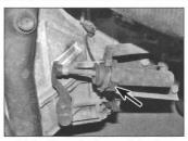
4.4 Locking collar (arrowed) for slave cylinder
