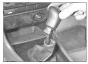
29.11 Removing the gear knob
