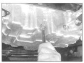
3.5 Slackening the engine oil drain plug
