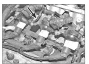
11.5a Coils position marked with masking tape – note earth lead (arrowed)
