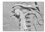
5.3 Remove split pin and upper ballioint nut - arrowed
