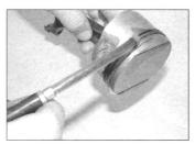
20.10a Lubricate the piston rings with clean engine oil . . .
