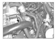
4.8 Remove outlet pipe (arrowed) from turbocharger hose
