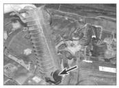
2.3a Disconnect air intake duct from lower part of housing – arrowed
