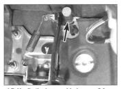
4.7 Unclip the inner cable (arrowed) from the upper end of the pedal
