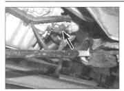
11.1 Oil pressure switch (and oil temperature sensor) location – 4-cylinder petrol engines
