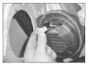
24.1c ... and disconnect the wiring
