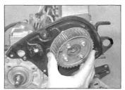
11.3 Removing the fuel injection pump drive (camshaft) sprocket
