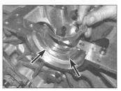
19.22 Oilways (arrowed) must face
