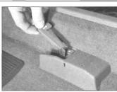
17.3 Pull off the control knobs . . .
