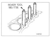
11.25 Tubular spacers and washers used to clamp liners
