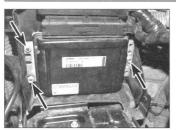
11.66 Undo the three mounting nuts
