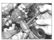
11.4 Use a small screwdriver to release the fuel rail rigid pipe
