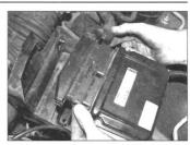
11.67 Slide the locking clips sideways, and disconnect the wiring plug
