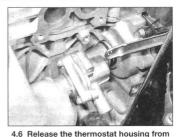
the pump and remove it from the vehicle (inlet manifold removed)
