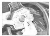
13.5 Disconnecting the airbag wiring connector
