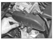
6.26 Undo the two cover retaining bolts
