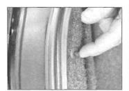
5.32 Press in the clip pins until flush
