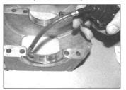
19.26 Lubricate the bearing shells in the bearing ladder with clean engine oil
