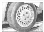
17.4 Checking the condition of the steering and suspension components by rocking a roadwheel
