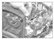
6.12 Release the clips (arrowed) securing the wiring harness to the timing belt cover
