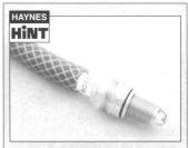
It is often difficult to insert spark plugs into their holes without cross-threading them. To avoid this possibility, fit a short length of suitable internal diameter rubber hose over the end of the spark plug. The flexible hose acts as a universal joint to help align the plug with the plug hole. Should the plug begin to cross-thread, the hose will slip on the spark plug, preventing thread damage to the cylinder head.
