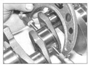
15.10 Measuring a crankshaft main bearing journal diameter
