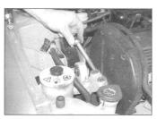
7.9b ... remove the mounting bracket bolts . . .
