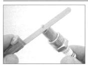
26.19a Measuring a spark plug gap using a feeler blade
