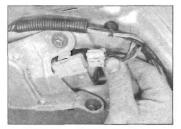
22.5 Disconnect the wiring . . . directly below the jet position (ie, the bottom
