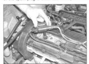
26.9 Undo the bolts and withdraw the coil
