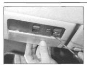
6.2a Use a screwdriver to prise off the interior light lens . . .
