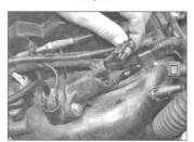
12.4b ... and the wiring plug from the purge valve
