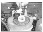
7.3 Using a hydrometer to measure the specific gravity of the coolant
