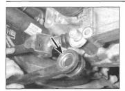
7.27 Disconnect the engine steady bar
