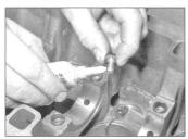
11.11 Apply thread-locking fluid to the oil spray jet securing bolts
