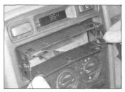
29.13b ... and remove the radio mounting
