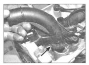
4.14 Remove the coolant elbow from the cylinder block
