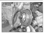
5.16 Withdrawing the coolant pump from its housing – diesel models
