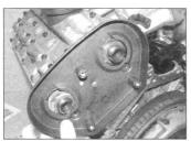
10.5 Removing a secondary belt backplate
