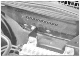
Vehicle identification number on engine compartment bulkhead
