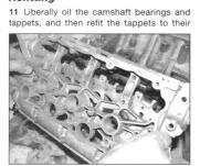
10.14 Refit the camshaft carrier onto the locating dowels
