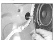
14.3b Loosening the front bolt securing the window glass to the regulator
