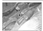
6.8 Locate peg into slot arrowed
