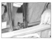
14.13c . . . then twist the channel through 90° and lift from the door
