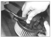
9.24 . . . and disconnect the wiring connector
