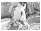
10.11 Using special tool to push the piston into the caliper
