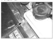
11.9a Remove the expansion tank bolt . . .
