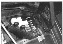
4 Additional fuses and relays are located in the fusebox at the left-hand side rear of the engine compartment.
