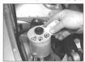
If topping-up is necessary, first wipe the area around the filler cap with a clean rag before removing the cap.
