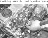
10.19 Removing the injector pipes
