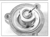
4.24 The stamped marking (arrowed) indicates the temperature at which the thermostat starts to open
