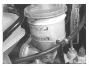
The brake master cylinder and fluid reservoir is located at the rear right-hand end of the engine compartment. The MAX and MIN level marks are indicated on the side of the reservoir and the fluid level should be maintained between these marks at all times.
