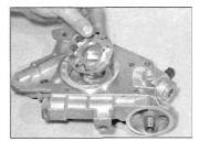
17.4 Lift out the oil pump rotors
