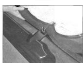
26.8 Unhook the seat cushion from the bracket anchorage point, and then using a socket,
