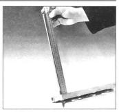
10.26 Measure the distance from the upper surface of the oil rail to the lower surface of the bolt head
