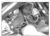
14.8 Disconnecting the MAP sensor pipe (arrowed) from the turbocharger
