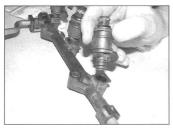
11.9b ... then ease each injector out of the fuel rail
