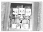
18.5 Handbrake cable adjuster nut (arrowed) and equaliser mechanism
