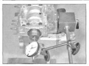
13.16 Checking camshaft endfloat using a dial gauge
