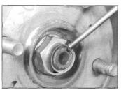
4.24 Use a punch to stake the driveshaft retaining nut
