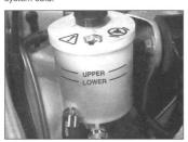
The power steering fluid reservoir is located on the right-hand side of the engine compartment. UPPER and LOWER level marks are indicated on the side of the reservoir and the fluid level should be maintained between these marks at all times.
