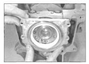
18.11 Slide the protector sleeve, oil seal and housing assembly over the end of the crankshaft – viewed with engine removed
