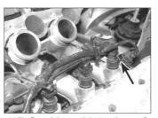
11.7b One of the rear injectors (arrowed) is reversed
