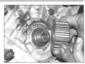
8.11 Removing the crankshaft sprocket
