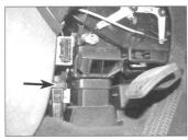
11.67 Fuel inertia cut-off switch location
