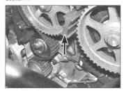
9.2 With the sprocket bolts slackened, remove the locking tool (arrowed)
