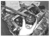
19.29b ... using an angle gauge ...
