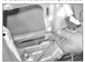
13.22 Releasing the front door lock operating rod from the guide
