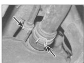
3.6 Release the clips (arrowed) and
