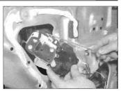
13.33 Removing the rear door lock from the door
