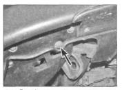
6.4a Front bumper outer mounting screw (RH side shown) . . .
