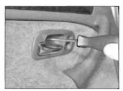
12.12 Removing the screw from the rear door interior door handle
