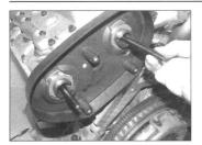
7.60 Fit the alignment pins into the camshafts
