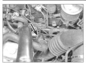
3.4 Crankcase pressure limiting valve - arrowed
