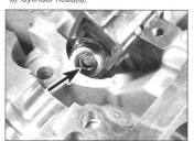
7.3a Using a valve spring compressor to release the split collets – arrowed
