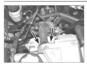
10.4 Undo the two EGR cooler pipe bolts - arrowed
