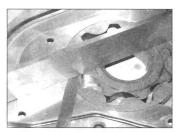
15.7 Check the rotor endfloat with a feeler blade and straight-edge
