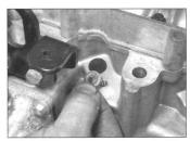
11.12 Fit new injector sealing washers in the cylinder head
