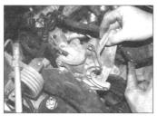
7.11d ... and remove the engine front plate
