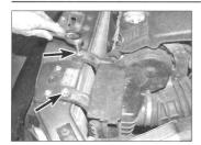
2.1 Remove the two bolts - arrowed
