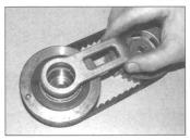
7.62a Place special tool 12-175 over the sprockets . . .
