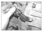
11.30 Disconnect the wiring plug . . .
