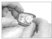
6.3 Fit the new battery, handling it with a piece of tissue paper to avoid touching the battery contact surfaces
