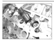
10.8 Using a suction tool to withdraw the hydraulic tappets
