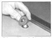
22.4b ... and remove the flat washer and rubber seal
