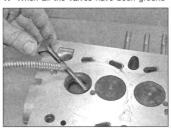
8.1 Lubricate the valve stems with clean engine oil
