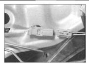
13.32 Disconnecting the wiring connectors
