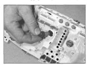
6.11a Removing a main panel illumination bulbholder . . .
