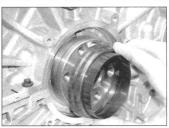
18.9 Fit the protector sleeve over the crankshaft
