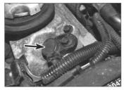
11.46 Camshaft position sensor location
