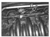
13.2d Low-pressure valve – 6-cylinder petrol models
