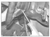
13.4 Undo the two airbag retaining screws
