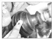
16.1 Inspecting a driveshaft joint rubber gaiter
