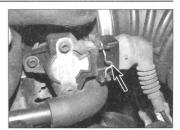
10.4 Disconnect the throttle position sensor wiring connector – arrowed
