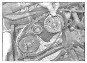
10.10 Slide the fuel injection pump drivebelt from the sprockets
