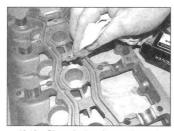
10.13a Clean the bearing carrier and cylinder head surfaces . . .
