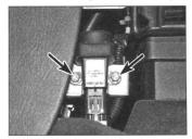
11.57 Undo the two bolts - arrowed
