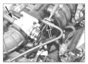
11.10 Disconnect intake and purge hoses (arrowed) from throttle housing
