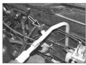
13.2e Low-pressure valve - diesel models
