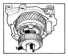
Install sliding sleeve for 5th and 6th gear complete with shift fork and driver, observing correct position. Installation position: Marks on synchromesh hub and sliding sleeve must line up.
