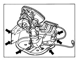
Headlight assembly is removed
