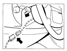
Direct to 2-pin plug of contact unit (below steering column).
