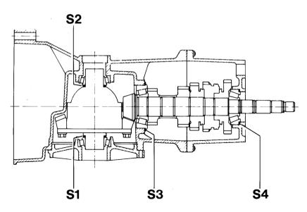
S1 = Ring gear adjustment shim
