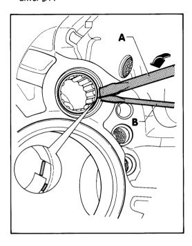
2. Drive out tapered roller bearing for drive pinion with Special Tool 9247/4 and punch tool VW 771/1.
