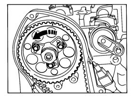
Tighten auxiliary bolts to 6 Nm (4 ftlb) and central bolt to approx. 40 Nm (29 ftlb). Remove oil line from camshaft adjuster.
