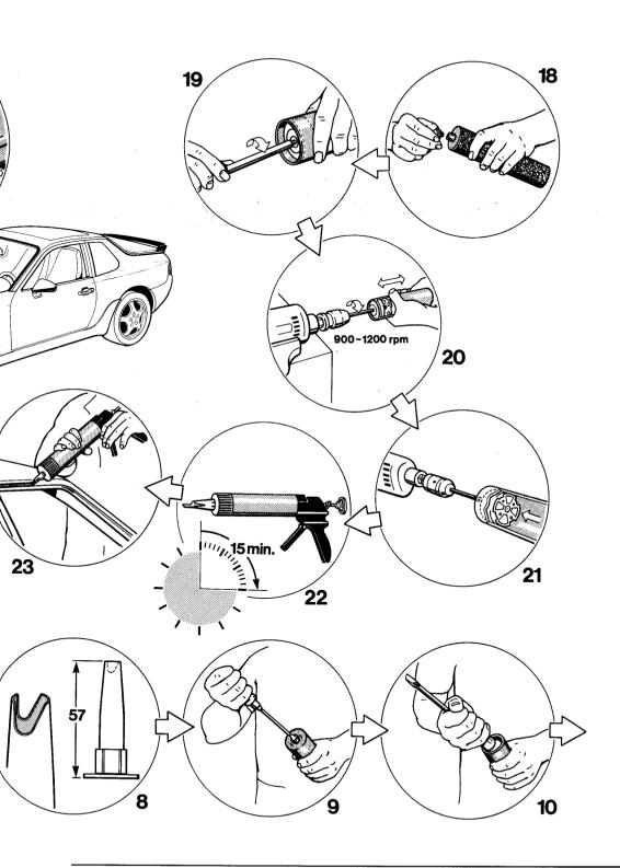
Removing and installing windshield — 2-pack adhesive
