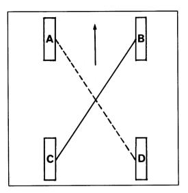
The left-to-right wheel load difference at the front and rear axles should be as small as possible (below 20 kgs, if possible).
