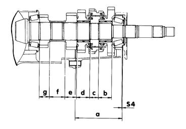
Dim. "a" = Housing depth of the end shield
