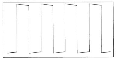
If no audible pulse is detected even though voltage is present and a signal is applied, replace the idle stabilizer.
