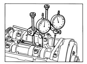
Remove distributor rotor and fit camshaft gear with 3 auxiliary bolts (M 5 x 15) to prevent the camshaft gear and the camshaft, respectively, from turning when the central camshaft bolt is undone.
