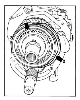
4. Press in roll pin, using Special Tool 3276.
