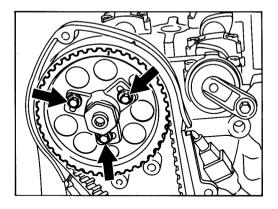
4. Undo central camshaft bolt, using a suitable retainer to keep the camshaft from turning. Rotate engine against the sense of rotation until the camshaft gear is against the stop within the woodruff key groove.
