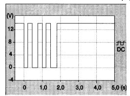
For the K wire, the following signal must be displayed:
