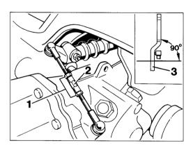
To adjust shift lever, move the shift lever support mount (arrow) to the front or rear until the inclination is 85°. The shift lever must remain in neutral position during this adjustment operation.
