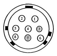
Bushing 3 = L wire Bushing 7 = K wire
