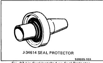
Fig. 27 Lip Seal Installed on Seal Protector
