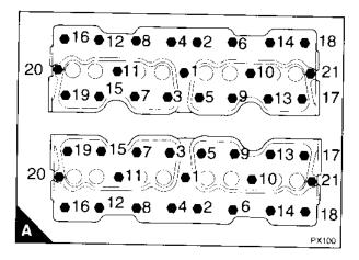
**Note:** Release the cylinder head setscrews evenly and gradually in the reverse sequence to that shown in (A).
