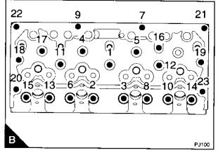
**Note:** Release the cylinder head setscrews evenly and gradually in the reverse sequence to that shown in (A).
