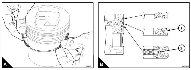
New second rings have a green identification mark which must be on the left of the ring gap when the ring is fitted and the piston is upright.
