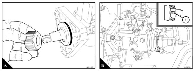
**4** Rotate the drive shaft of the fuel pump clockwise from the drive end of the pump until the pin in the shaft aligns with number 1 outlet. Loosen the screw (C3) on the timing tool 21825610 and set the timing tool to the correct pump mark angle, see "Engine timing (Stanadyne fuel injection pump)" on page 46. Tighten the screw.
