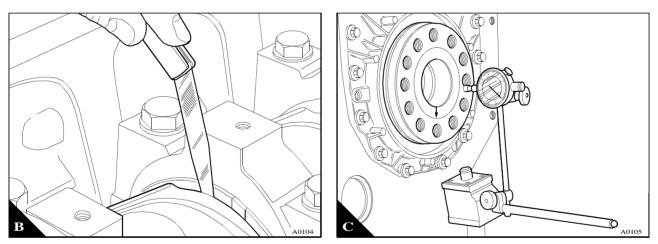
If the end-float is more than the tolerance given in the relevant Data and dimensions for the "Crankshaft" on page 36, thrust washers which are 0,019 mm (0.0075 in) oversize can be fitted.
