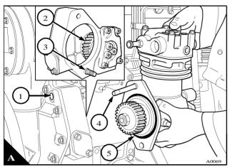
**3** Rotate the crankshaft of the compressor until the mark (B1) or (C1) on the rear face of the crankshaft aligns with the 6A line (six cylinder engines) or the 4A line (four cylinder engines) on the label on the rear face of the compressor.
