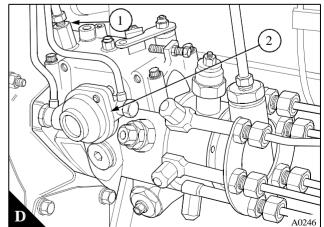
Some naturally aspirated engines have a Stanadyne fuel injection pump (A) fitted. The electrical stop solenoid on these fuel pumps is fitted inside the governor housing. The earth connection (A1) and the electrical supply connection (A2) are on top of the governor housing.
