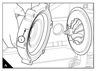
It is important that the waste-gate actuator setting is not altered. Do not remove the actuator or mounting bracket unless it is necessary to renew the actuator assembly.
