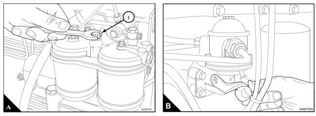
*Caution:* spanner to prevent movement of the fuelled starting aid (C1) when the union nut is loosened or tightened.
