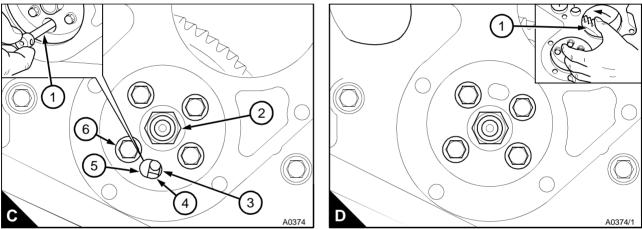
**Caution:** Do not tighten the union nuts of the high-pressure pipes more than the recommended torque tension. If there is a leakage from the union nut, ensure that the pipe is correctly aligned with the atomiser inlet. Do not tighten the atomiser union nut more, as this can cause a restriction at the end of the pipe. This can affect the fuel delivery.
