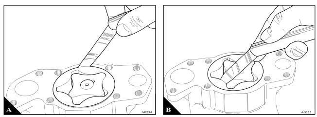
**5** Check the rotor end-float with a straight edge and a feeler gauge (C). For all the above clearances, refer to the relevant Data and dimensions for the "Lubrication system" on page 48.
