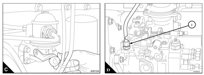
**Caution:** spanner to prevent movement of the fuelled starting aid (E1) when the union nut is loosened or tightened.
