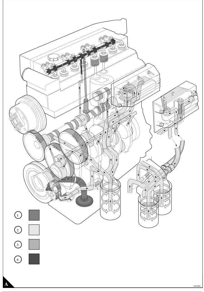
Lubrication system flow diagram for the relief valve and balancer
