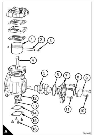
**2** Ensure all components are clean. Fit a new 'O' ring (A6) in its recess in the end plate (A7). Lubricate the 'O' ring with clean engine lubricating oil.
