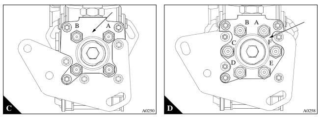
7 Check that the pump plunger is at its lowest position and set the dial of the gauge to zero. There will be no tension on the bar used to turn the pump in this position.
