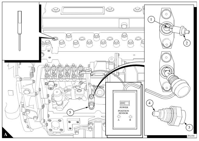
**Caution:** Ensure that the drive shaft of the pump is not rotated while the pin is engaged with the tag in the governor housing. If the shaft is rotated, damage could occur to the tag in the governor housing.
