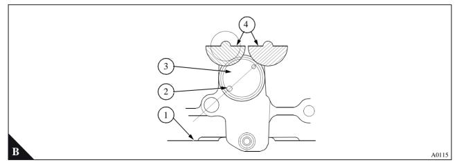
**7** Fit the two dowels to the rear face of the balancer frame. Lubricate the bushes in the rear cover of the balance frame with clean engine lubricating oil. Put the rear cover in position with the rear spigots of the balance weights in the bushes of the cover. Hit lightly the rear cover with a soft face hammer to fit the cover onto the dowels. Fit the cover setscrews and tighten them to 54 Nm (40 lbf ft) 5,5 kgf m.
