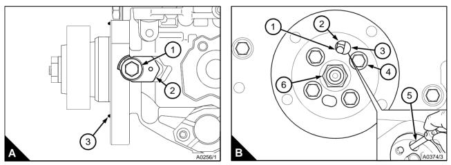
5 Tighten the flange nuts of the fuel pump to 28 Nm (20 lbf ft) 2,8 kgf m.
