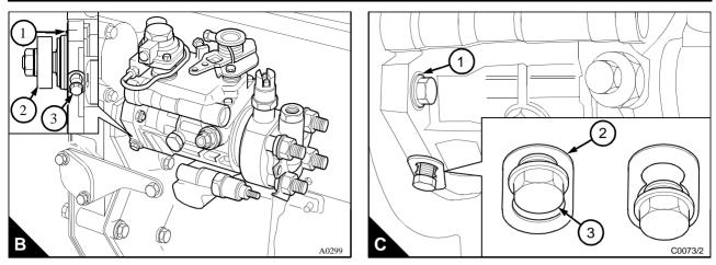
The fuel injection pump has a locking screw (B3) and (C3) and a spacer (C2). The locking screw prevents the rotation of the drive shaft.
