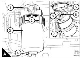
**Note:** If the filter does not have a drain device fitted release the cap (A1) on top of the filter head. Remove the nylon insert to lower the level of the fuel in the filter canister. This will prevent fuel spill when the clamp ring is released.
