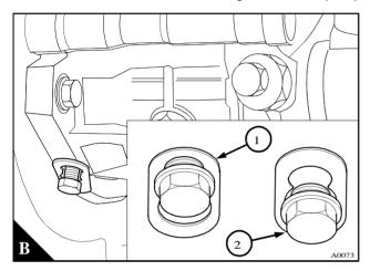
1 Inspect the "O" ring and, if necessary, fit a new "O" ring.
