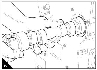
1 Ensure that all components are clean and are lubricated with clean engine lubricating oil.
