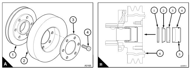
**3** Remove the three setscrews and the thrust block (B4). If the pulley is not free, **do not use an extractor to remove the pulley**. Hold a wooden block against the inner hub of the pulley and with a hammer, lightly hit the wooden block towards the rear (C) to loosen the tapered rings.
