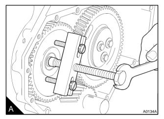
1 Ensure that the key in the camshaft is fitted correctly.
