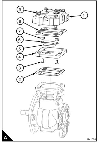
**3** Fit and align a new inlet reed (A2).
