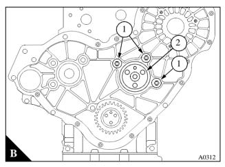
**7** Fit the camshaft gear, see Operation 6-13, and the idler gear, see Operation 6-7. Ensure that all the timing marks are correctly aligned.
