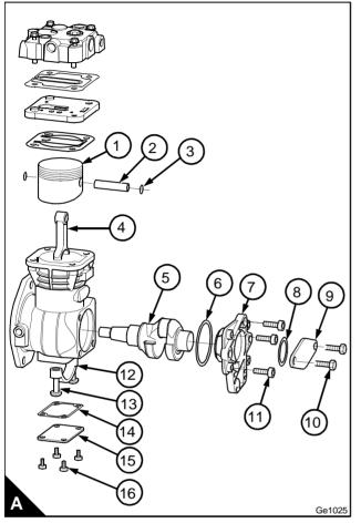
5 Remove the connecting rod setscrews (A13) and remove the connecting rod bearing cap (A12).
