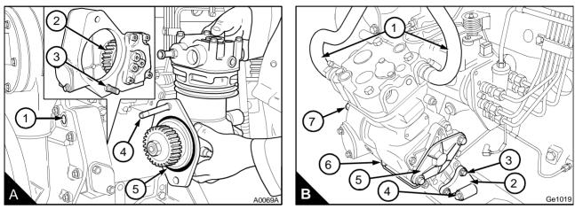
**3** With the rear cover plate (B5) (or the hydraulic pump removed), rotate the crankshaft of the compressor until the mark (C1 - DIN crankshafts) or (D1 - SAE crankshafts) on the rear face of the crankshaft aligns with the 6A line (six cylinder engines) or the 4A line (four cylinder engines) on the label on the rear face of the compressor.
