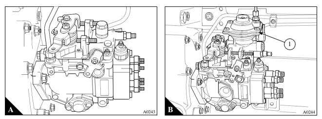
Lucas/Delphi DPA fuel injection pumps (B) are fitted to naturally aspirated engines. Turbocharged engines have Lucas/Delphi DPA or DPS fuel pumps (B). The DPS fuel pumps have a boost control (D2). Some of these pumps are fitted with a self-vent feature (D1).
