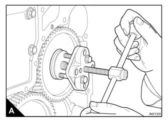
1 Ensure that the key is fitted correctly in the fuel pump shaft. Fit the gear and the spring washer and loosely fit the nut.
