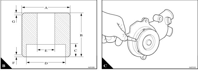
The dimensions of the tool to fit the coolant seal, will ensure that the seal is the correct length after it is installed. It will also prevent axial distortion of the seal when it is pressed onto the shaft.
