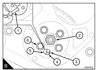
**7** Carefully turn the gear counter-clockwise, by hand (C1), to remove the backlash between the idler gear and the fuel pump gear. Do not rotate the crankshaft or the fuel pump shaft. Tighten the flanged setscrews for the fuel pump gear to 28 Nm (20 lbf ft) 2,8 kgf m.
