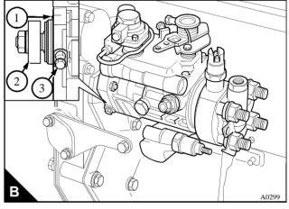
**Caution:** Do not remove the nut (C2) from the shaft of the fuel injection pump. The fuel pump hub is fitted to the shaft in the factory to ensure that the fuel pump is in the correct position for timing. If the hub is removed, it will need to be accurately fitted to the pump by use of special equipment available to Perkins distributors.
