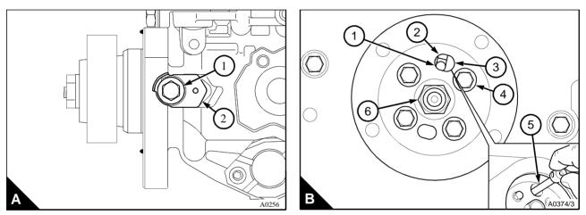
**Caution:** Use a second spanner to prevent movement of the high-pressure outlet when the union nut for each high-pressure pipe is released.
