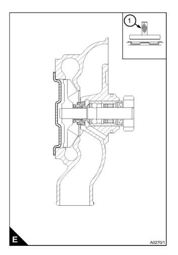
**7** Clean the threads in the front face of the pump body. Fit a new joint (F8) and the cover (F7). Fit the setscrews and tighten them to 9 Nm (6 lbf ft) 0,9 kgf m. If the setscrews are new, a sealant will have been applied to the threads by the manufacturer. If the original setscrews are to be used again, the threads should be cleaned and a POWERPART Threadlock and nutlock applied.
