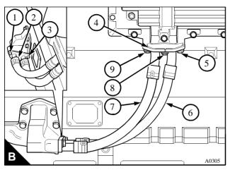
**2** Put the outer pipe (B7), in position on the flange of the oil cooler and fit the third setscrew (B9) finger tight. Beginning with the centre setscrew, tighten the three setscrews to 22 Nm (16 lbf ft) 2,2 kgf m.
