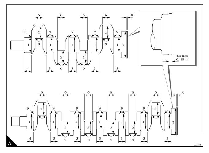
With the crankshaft on mountings at the front and rear journals, the maximum run-out (total indicator reading) at the journals must not be more than shown below:
