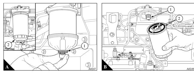
Warning! Discard the used canister and fuel oil in a safe place and in accordance with local regulations.
