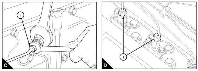
Warning! When the starter motor is operated to eliminate air from the high pressure pipes, the engine may run.
