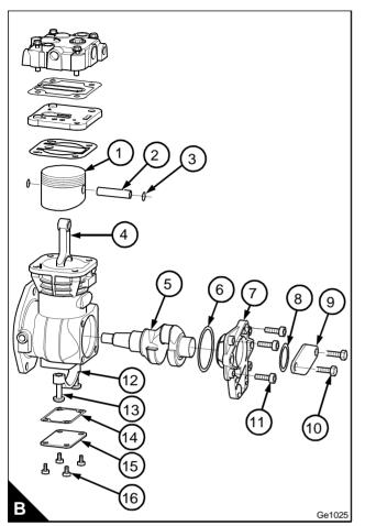
**9** Fit the two bearing cap retaining setscrews (B13) by hand. If they do not fit freely by hand, fit new setscrews. If the new setscrews do not fit freely by hand, fit a new connecting rod.
