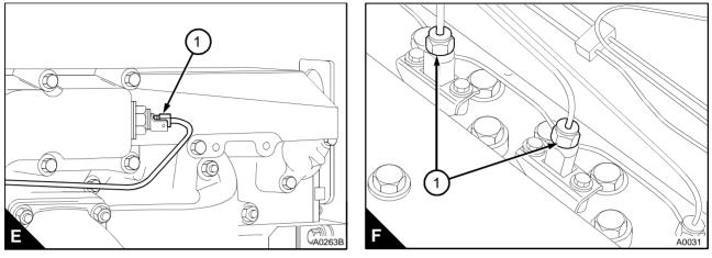
7 Loosen the high-pressure pipe connections (F1) at two of the atomisers.
