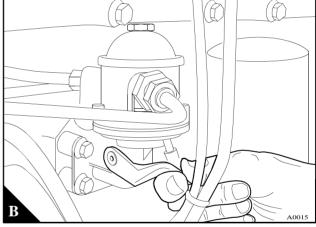
*Caution:* spanner to prevent movement of the fuelled starting aid (E1) when the union nut is loosened or tightened.
