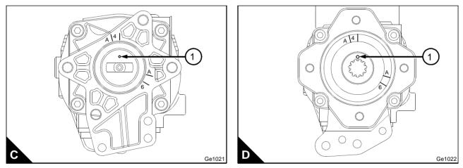
**5** Slide the compressor forward until the teeth of the drive gear are against the teeth of the idler gear (A2). Slowly rotate the crankshaft of the compressor clockwise (from the rear) until the drive gear and the idler gear are in mesh.
