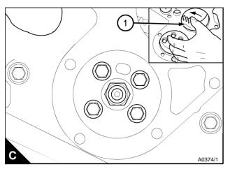
9 Remove the timing pin.
