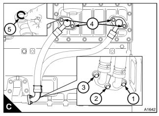
**2** Put the flange of the outer pipe in position and fit the third setscrew (C3), tighten it finger tight. Beginning with the centre setscrew, tighten the three setscrews to 22 Nm (16 lbf ft) 2,2 kgf m.
