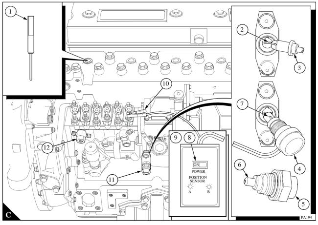
**15** Press the switch on the timing light to the "OFF" position. Disconnect the earth lead, remove the probe of the timing light from the timing attachment and remove the timing light.
