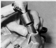
11.98B Settle the circlip by tapping the socket
