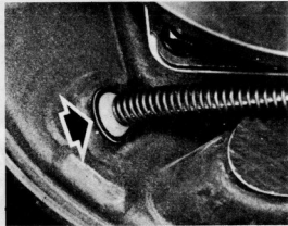
Fig. 9.13. Brake cable locking clip on backplate (Sec. 10)
