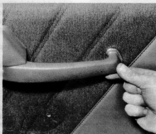
16.3B Swivel the arm rest through 90° to remove it
