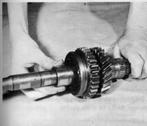
6.15ii Refitting the mainshaft sleeve
