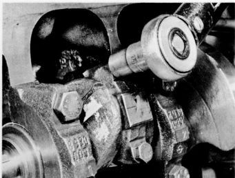
41.5 Tightening the big-end bolts
