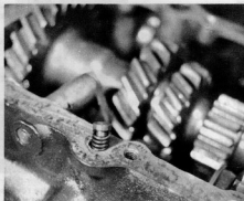
7.19b Refitting the spring end caps
