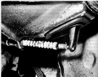
3.8. Lower end of clutch cable and rubber sleeve
