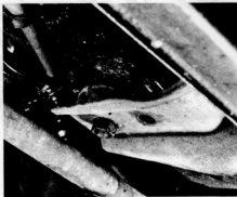
5.4a Radiator lower attachment point
