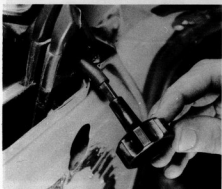
16.10B Removing the exterior mirror control knob
