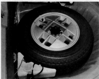
14.13 View of spare wheel and tailgate washer reservoir
