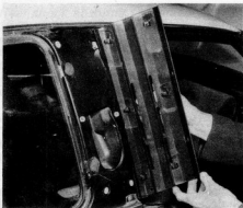
16.13 Removing the rear extractor grille (Hatchback)
