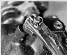
7.25 Split pin retaining RH lever to transverse selector shaft
