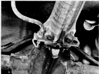
2.19 Location of brake pipe on extension housing
