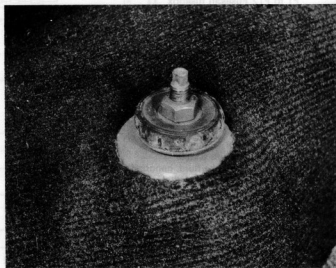
15.13 Rear shock absorber upper mounting on a late Manta
