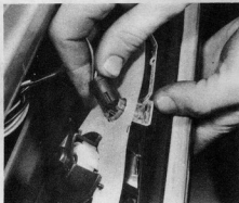
14.62 Disconnecting the multi-plug from the rear light cluster
