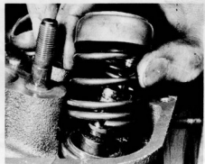
45.5 Installing an exhaust valve spring and cap
