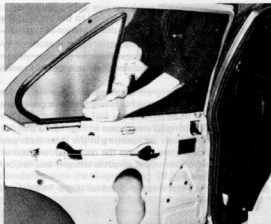
Fig. 12.16. Lifting out the rear door quarter glass (Sec. 14)
