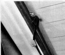
16.19 Heated rear window connection (Hatchback)
