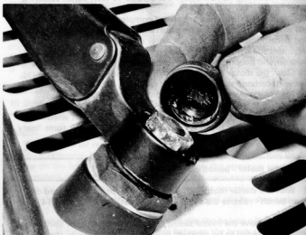
19.3 Removing the wiper arm cap (early models)
