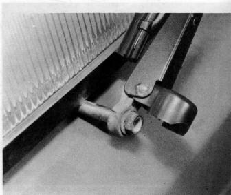
14.28A Unscrew the nut ... on the pump on this side of the wiper
