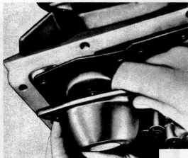
Fig. 6.24. Removing the brake band servo cover (Sec. 21)
