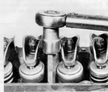
47.8 Tightening the cylinder head bolts
