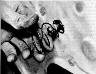
10.11 Replacing the window regulator shaft spring
