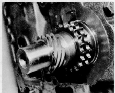
43.2 Correct position of the timing sprocket and auxiliary drive gear
