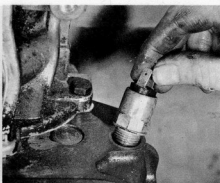
7.21b Refitting the reversing light switch
