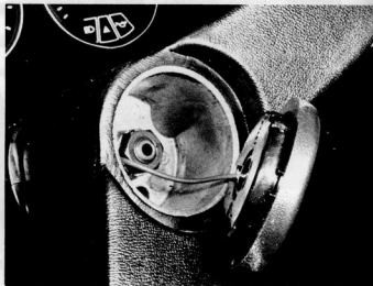
22.1 Lifting out the horn button
