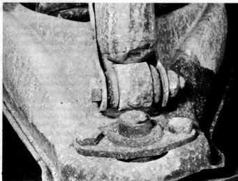
3.2 Front shock absorber lower mounting
