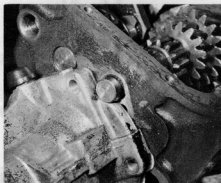
7.15b Refitting layshaft gearcluster shaft
