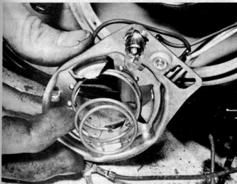
27.3 Headlight bulb retaining plate, note side light bulb
