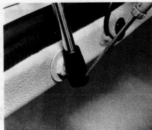
16.20A Prising out the lid stay wedge (Hatchback)
