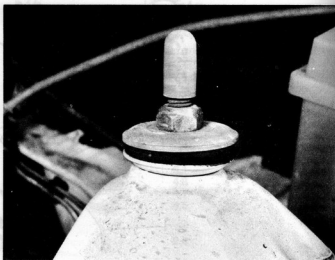
3.3 Front shock absorber upper mounting
