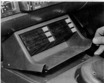
16.48 Removing the cassette storage box
