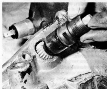
3.11 Speedometer drive removal
