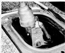
51.4e Refitting the gearstick
