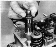
5.201 Fitting a hydraulic valve lifter to the cylinder head
