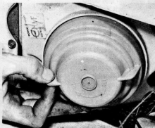
27.1 Removing the plastic cover from the rear of the headlight unit
