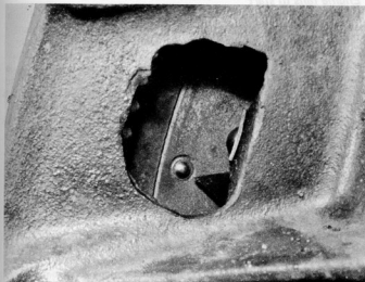
8.4 Static timing ball and pointer on flywheel
