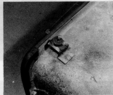
14.48C Trim strip mounting screw on the headlight (removed)
