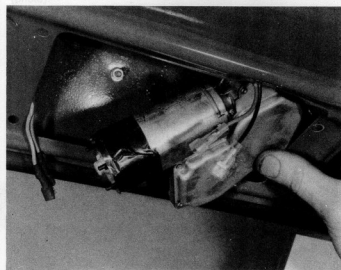
14.10 Removing the tailgate wiper motor
