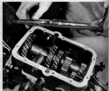
7.20 Refitting the gearbox baseplate
