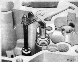
Fig. 13.23 Removing the partial load piston retainer (Sec 8)
