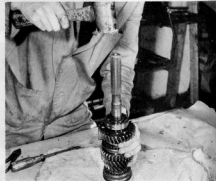
6.4 Removing mainshaft bearing and first gear
