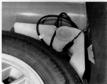
14.14 Tailgate washer reservoir showing wiring and tubing
