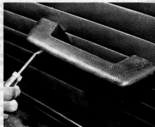
10.6 Removing the front door armrest
