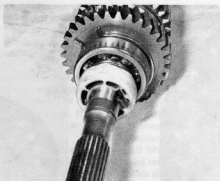
6.15ix Refitting speedometer drive
