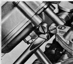
Fig. 3.30. Removing the vacuum control unit - Zenith (Sec. 9)
