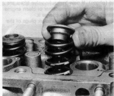
5.199 Fitting a valve spring and cap
