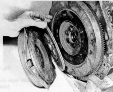
6.4 Clutch friction disc and pressure plate
