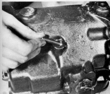
7.10a Inserting the selector shaft locking bolt and spring
