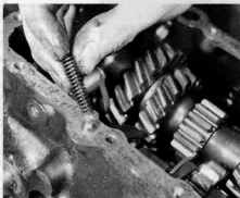
7.19a Inserting the selector shaft ball and spring
