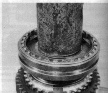
11.70 Using a piece of tube to fit 1st/2nd synchro body
