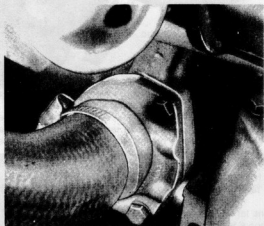
Fig. 13.14 Thermostat housing on the 1.8 ohc engine (Sec 7)
