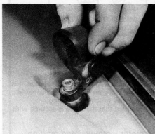
14.6 Tailgate wiper arm securing nut
