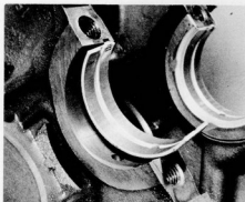
37.2 Fitting the main bearing shells
