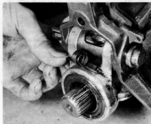
3.8a The pivot spring being removed
