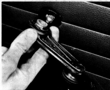
10.4a Removing the window regulator handle
