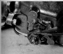
7.22 Location of lever on the transverse selector shaft
