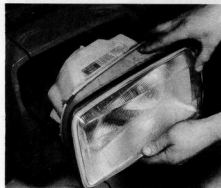
14.49 Removing the headlight unit
