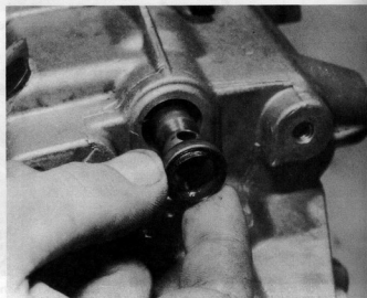
11.113 Fitting the selector rod oil seal
