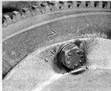
6.2 Alignment marks on clutch cover and flywheel
