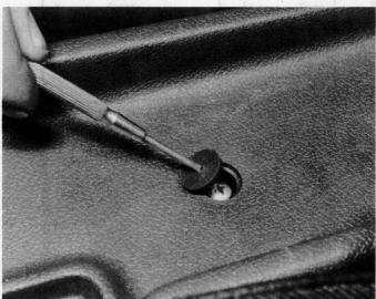
16.49A The rear screws are covered with plastic plugs
