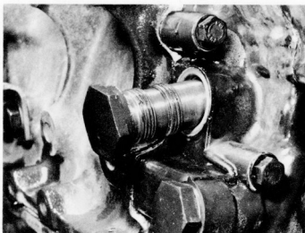
43.10 Insert the timing chain tension plunger
