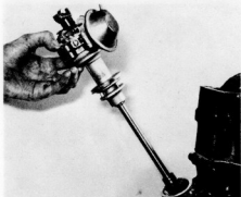
49.4 Refitting the distributor and driveshaft
