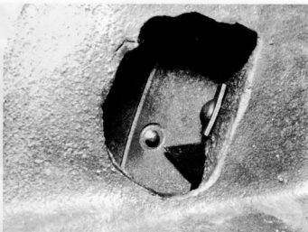
49.2 Static timing mark on flywheel
