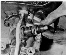
7.21a Installing the speedometer drive
