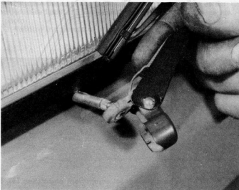
14.28B ... and remove the headlamp wiper arm
