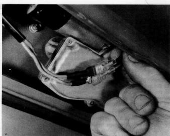
14.9 Tailgate wiper motor wiring
