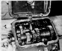
3.10 Lifting off the gearbox baseplate
