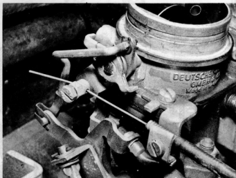
5.3 Choke control cable - single barrel carburettor
