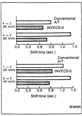
Compared to the conventional A/T manual shifting, the down-shifting time is shortened by 0.1 sec. or more, and the up-shifting time by 0.2 sec. or more.
