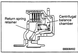
When the engine is running at high speed, the transmission fluid remaining in the piston hydraulic pressure chamber is subjected to centrifugal force and pushes against the piston, but the piston does not move because the fluid which fills the centrifugal balance chamber (between the piston and the return spring retainer) also generates centrifugal force which pushes back the piston, and both forces cancel each other out.
