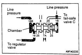
(2) In 3rd, 4th and 5th gear, because hydraulic pressure is also supplied to the chamber in the left side of the valve from the No.16B port, the valve is pushed to the right because of the difference in area between the No.1 land and the No.4 land. This causes the No.18 port to open, and hydraulic pressure is thus supplied to the No.18B port of the regulator valve.
