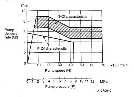
P-Qf characteristic: Pump pressure and pump delivery rate
