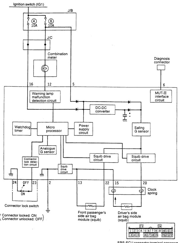
SRS-ECU connector terminal arrangement
