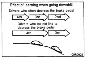
For drivers who frequently depress the brake pedal when going downhill, the learning control causes the transmission to downshift earlier so that the engine brake can be used more easily. Conversely, for drivers who do not like to depress the brake pedal much even when going downhill, down-shifting is made more difficult in order to suppress the engine brake.
