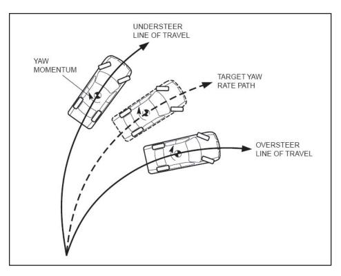
Direction of travel is determined by inputs from the steering angle sensor and the combined sensor. The combined sensor measures yaw angle, and forward and lateral G-forces.
