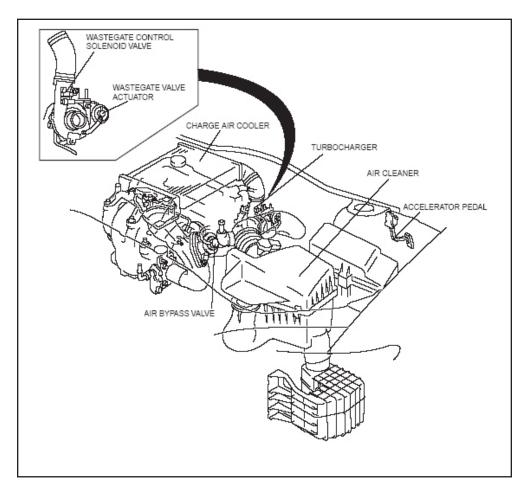
The main components of the turbocharging system are:
