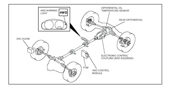
The 4WD ECU uses real-time data to manage torque.
