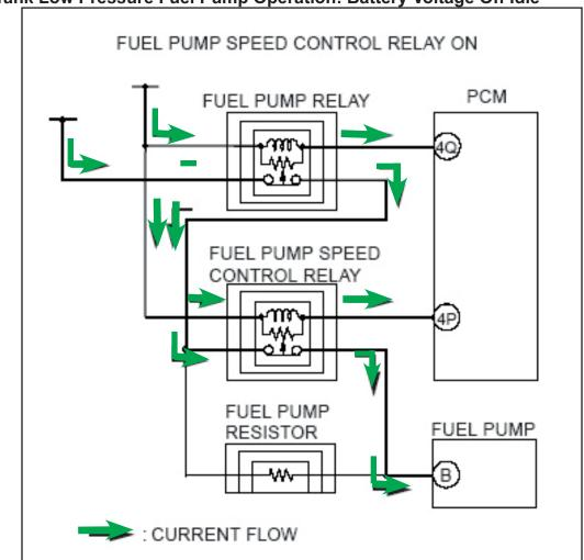
In-Tank Low Pressure Fuel Pump Operation: Battery Voltage Off Idle
