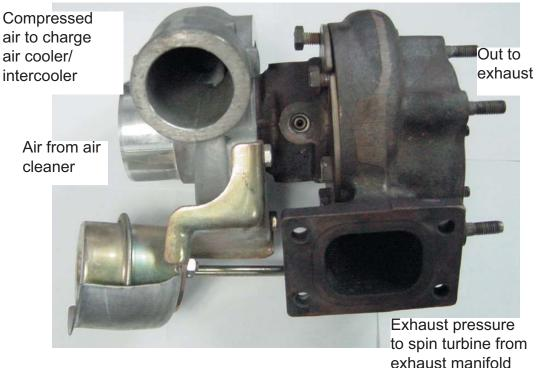
Turbochargers consist of a housing, a blade assembly, inlet ducts for low pressure air and outlet ducts for high pressure air, an intercooler, oil inlet and return, coolant inlet and return, and boost control circuits.
