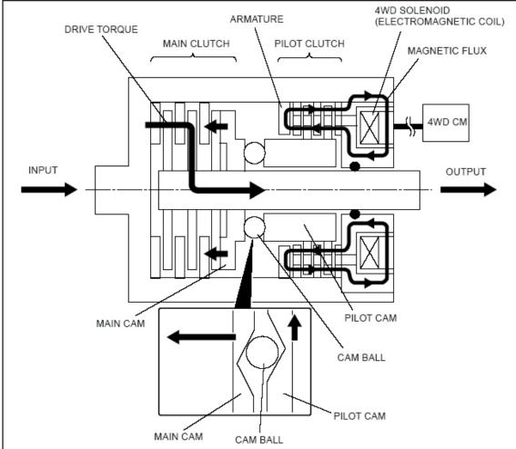
When the electromagnetic coil is energized and the front wheels rotate at a different rate than the rear wheels, the ball separates the main cam and the pilot cam. This exerts force on the main clutch and torque is transmitted from the driveshaft to the rear differential.
