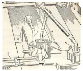
Fig. 21. Setting gearbox control levers
