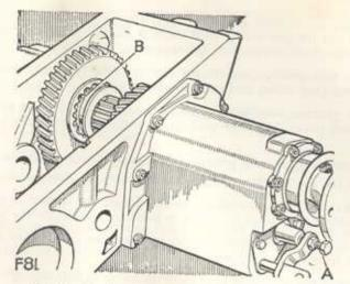
Fig. 13. Setting the transfer selector travel stop.
