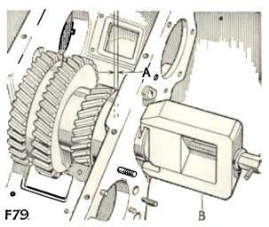
Fig. 8. Removing the intermediate shaft
