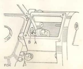
Fig. 14. Adjusting 2nd gear stop bolt
