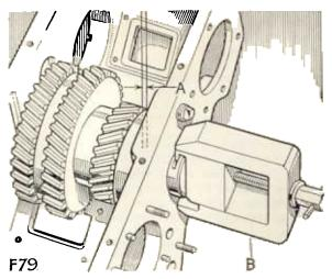
Fig. 12. Checking end-float of intermediate gears
