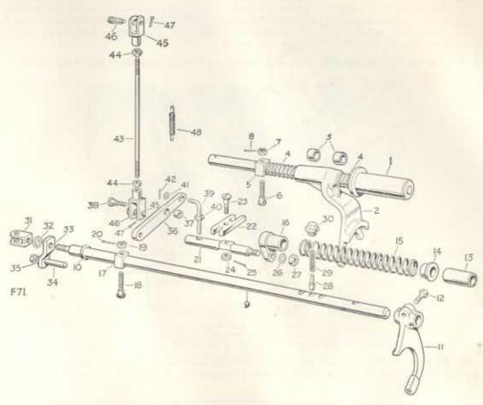
Fig. 7. Front wheel drive and transfer selector assemblies
