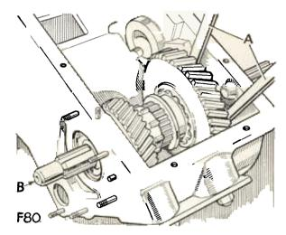
Fig. 9. Removing transfer box output shaft
