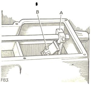
Fig. 20. Adjusting reverse stop hinge plate
