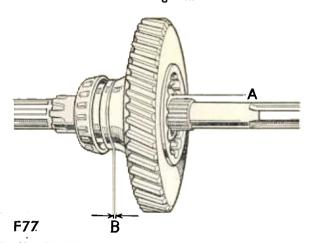
Fig. 10. Checking end-float of the 'low' transfer gear wheel
