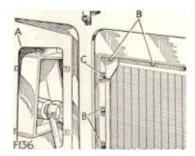
Fig. 25. Radiator securing bolts
