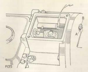
Fig. 15. Adjusting reverse gear stop bolt
