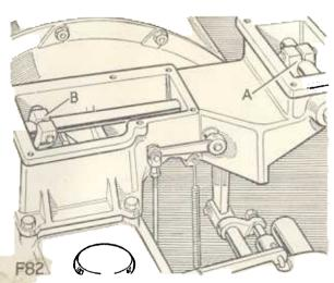
Fig. 19. Gearbox controls, rear housing
