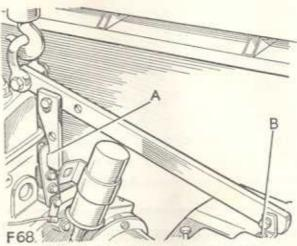
Fig. 5. Engine lifting sling in position
