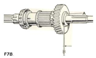
Fig. 11. Checking end-float of the 'high' transfer gear wheel
