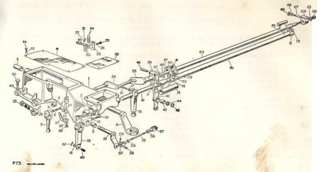
Fig. 18. Gearbox controls, rear assembly
