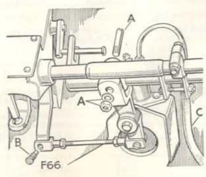
Fig. 4. Removing gearbox controls
