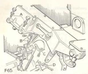
Fig. 3. Removing gearbox controls
