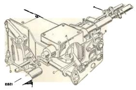
Fig. 22. Setting gearbox control linkage
