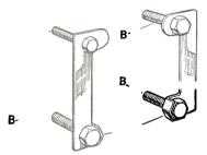
Fig. 24. Assembling securing bolts to lock-plate  $B = \frac{3}{9}$  in, bolt C = Lock heads of
