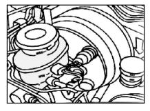
Examine the brake performance and whether there is any leakage at joints and whether the level of oil cup meets requirements.
