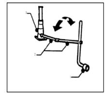
Lock the component 3 as indicated and than connect the components 2 and 1. Rotate as indicated direction to raise or lower the jack to fulfill desired operations. When the jack has been lowered to its lowest point, component 3 can be released and take way easily.
