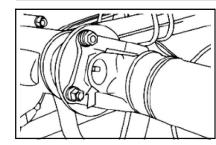
Lubricating the driveshaft Add No. 3 lubricant to the drive shaft as indicated. Stop filling until an overflow.
