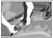
Pull the webbing attached to the latch plate over the chest and pelvis. Lock the latch plate in the buckle and examine it manually, where an expected "click" sound means successful engagement.
