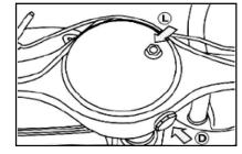
Replacing Main Reducer Oil Remove the drain plug to discharge gear oil from the rear axle. Fill the specified gear oil into the axle housing through the screw-plug hole. Stop filling until oil overflows from the same hole.
