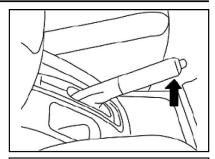
Lifting up handbrake forcibly while parking. The first gear may be selected if parking on s steep surface. The braking light will illuminate when the handbrake is engaged and the ignition switch is on.
