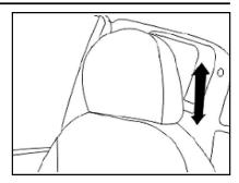
A front headrest can be regulated in height and angle to suit an individual's physical conditions. Properly adjust both the headrest and belt can provide you effective protection.
