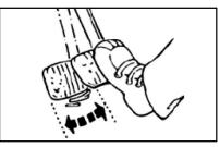
Adjusting the brake pedal The push-rod serves as the stopper when the brake pedal has been completely released.
