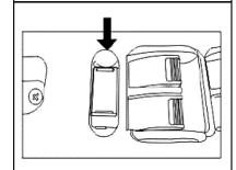
Central Control Door Lock Button The central control door lock button is provided to open/close all doors internally that is positioned in the driver's handle (As shown in figure above).
