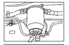
Drain moisture in the circuit as indicated in order to clean fuel
