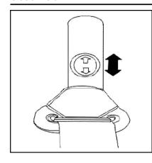
Use belt height-adjusting device to adjust and get your desired frontal sash height.
