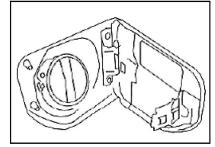
The filling pipe is attached to rear RH cover.
