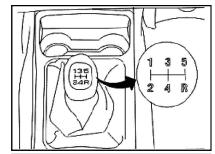
Do not select the reverse gear until the vehicle comes to a full stop. Fully press the clutch pedal when the engine is running, wait a moment to avoid abnormal noises from gear shifting. The reverse light will illuminate when the reverse gear is selected and the ignition switch is turned to ON Position.
