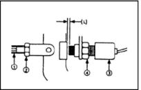
Adjusting the clutch pedal
