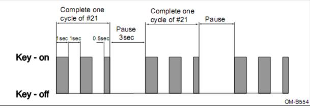
Example of displaying two fault codes 13 and 22
