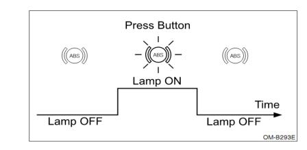
**Note:** On some bus models, the ABS self-diagnosis button is combined to the button Inspection lamps "Bulb Check".
